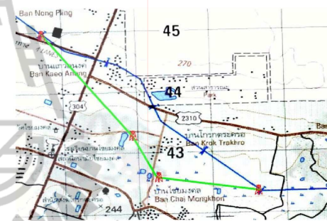
Fig. 9 Topographic map of a power transmission line portion for rerouting (first example)
