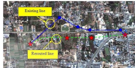
Fig. 12 Satellite image of a power transmission line portion for rerouting (second example)
