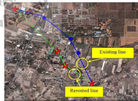
Fig. 10 Satellite image of a power transmission line portion for rerouting (first example)
