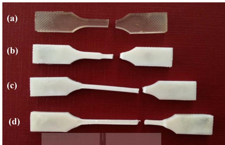
**Figure 4.7** Optical photographs of tensile-fractured samples of (a) PLA, (b) PLA/PBAT 90/10 blend, (c) PLA/PBAT 80/20 blend, and (d) PLA/PBAT 70/30 blend.
