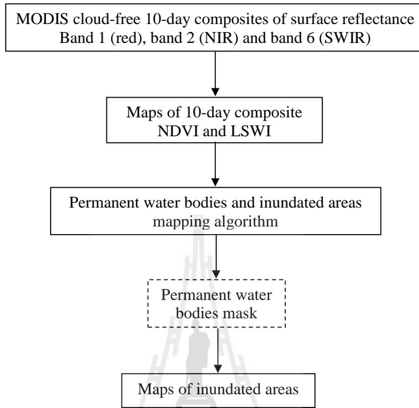
**Figure 3.2** Diagram of algorithm for mapping of inundated areas.
