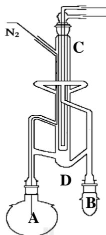
**Figure 2.1** Scheme of the microextractor for simultaneous steam distillation-solvent extraction. A= Sample flask, B = Solvent flask, C= Cold-finger, D = Separation chamber.
