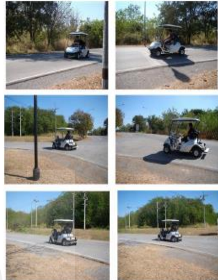
Figure 14. Testing left-turn action in actual road environment.
