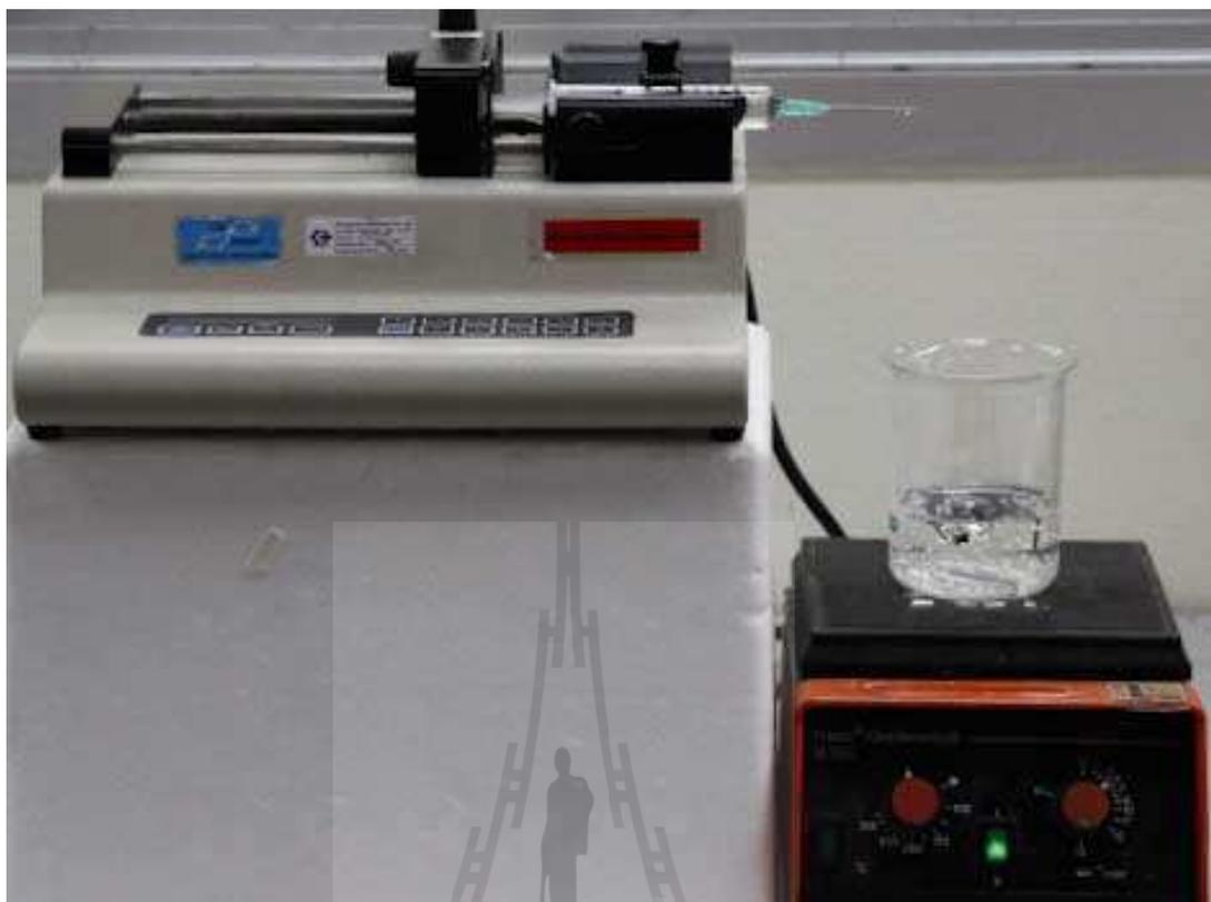
**Figure 11.** Equipment for gel forming using hypodermic syringe.
