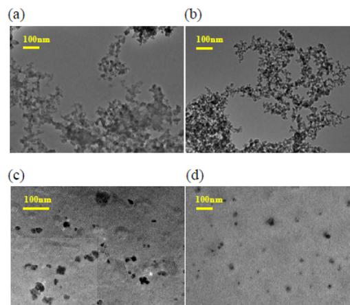
Figure 5. TEM images of (a) pure 7 nm, (b) pure 14 nm, (c) 0.5 wt% of 7nm filled H14, and (d) 1 wt% of 14 nm filled L5 at the scale bar of 100 nm.
