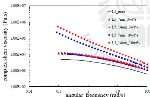
Figure 4. Complex viscosity versus frequency for 7 and 14 nm fumed silica filled L5 at 0, 3, and 10 wt%
