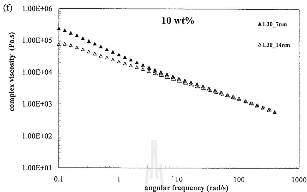
**Figure 4.8** Variations of complex viscosity versus frequency for 7 and 14 nm fumed silica filled L30 at constant filler loadings of (a) neat, (b) 0.5 wt%, (c) 1 wt%, (d) 3 wt%, (e) 5 wt% and (f) 10 wt% at the reference temperature of 160°C (continued).
