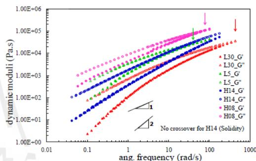
Figure 2. Master curve of dynamic moduli versus frequency of long-chain branched (L30 and L5) and linear (H14 and H08) polyethylenes at 160°C.
