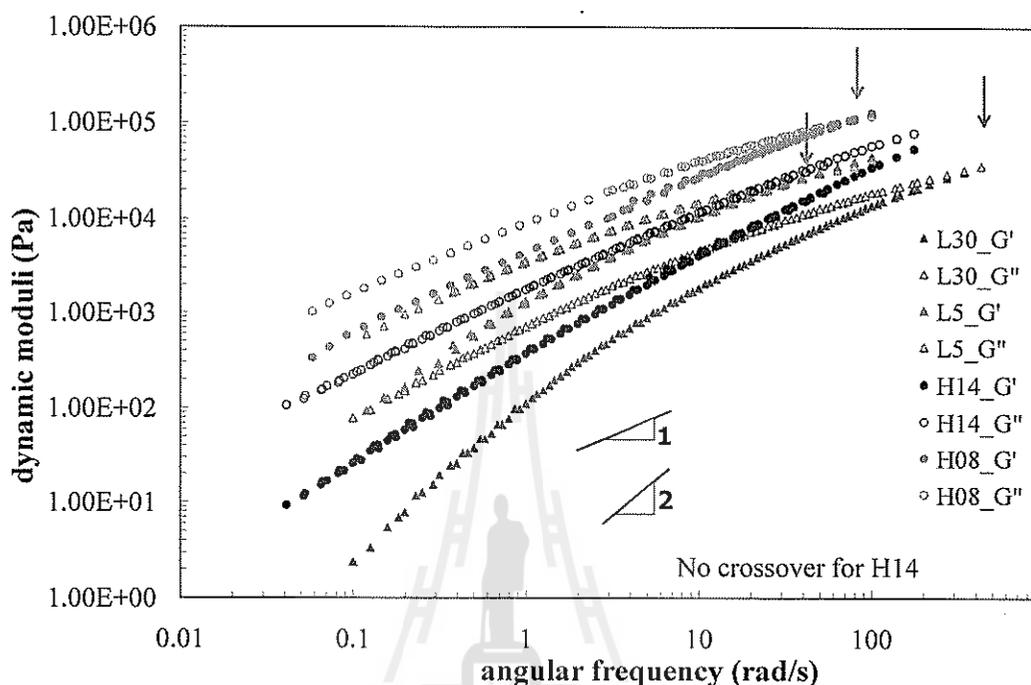
**Figure 4.3** Master curve of dynamic moduli versus frequency of long-chain branched (L30 and L5) and linear (H14 and H08) polyethylenes at the reference temperature of 160°C.
