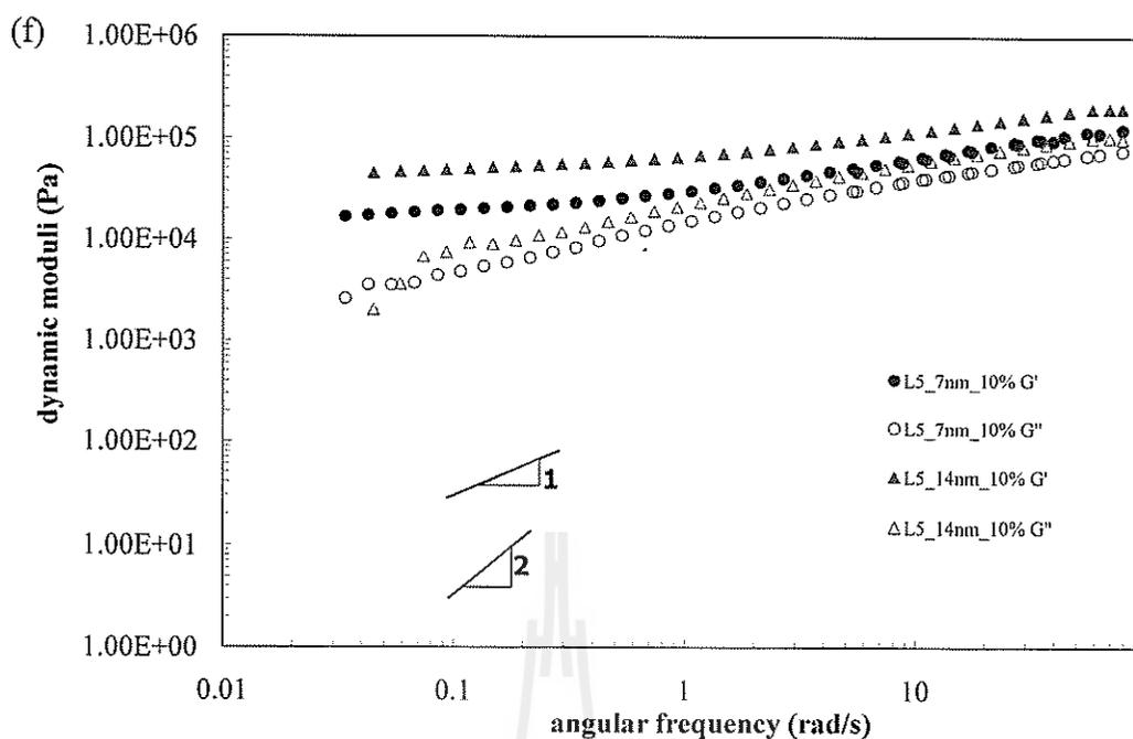
**Figure 4.5** Storage and loss moduli of the fumed silica (7 and 14 nm) filled L5 melts at various contents (wt%) as a function of the angular frequency at the temperature of 160°C (continued).
