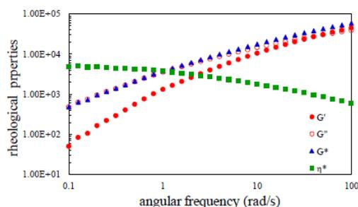
Figure 1. Typical LVE behavior in the terminal region of polymer melts (here is neat L5 at temperature of 160°C).
