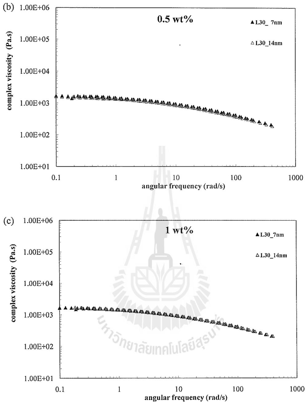
**Figure 4.8** Variations of complex viscosity versus frequency for 7 and 14 nm fumed silica filled L30 at constant filler loadings of (a) neat, (b) 0.5 wt%, (c) 1 wt%, (d) 3 wt%, (e) 5 wt% and (f) 10 wt% at the reference temperature of 160°C (continued).
