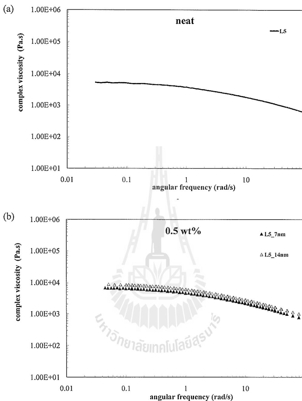
**Figure 4.7** Variations of complex viscosity versus frequency for 7 and 14 nm fumed silica filled L5 at constant filler loadings of (a) neat, (b) 0.5 wt%, (c) 1 wt%, (d) 3 wt%, (e) 5 wt% and (f) 10 wt% at the reference temperature of 160°C.
