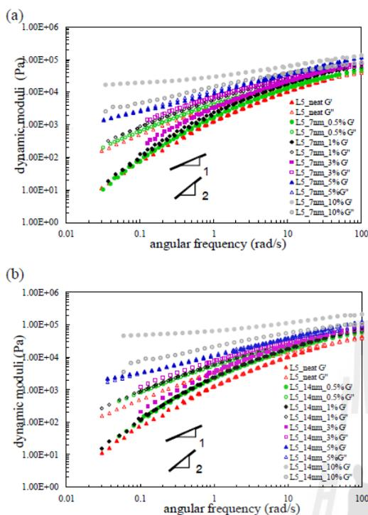
Figure 3. Storage and loss moduli of the fumed silica (a) 7 and (b) 14 nm filled L5 melts at various contents (wt%) as a function of the angular frequency at the temperature of 160°C.
