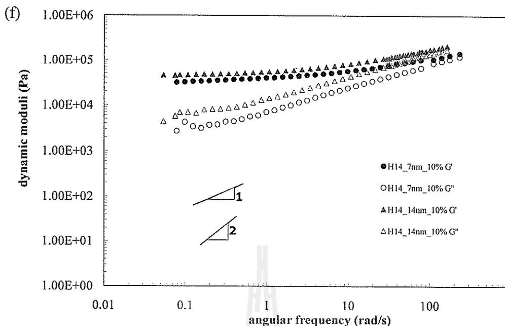
**Figure 4.10** Storage and loss moduli of the fumed silica (7 and 14 nm) filled H14 melts at various contents (wt%) as a function of the angular frequency at the temperature of 160 °C (continued).
