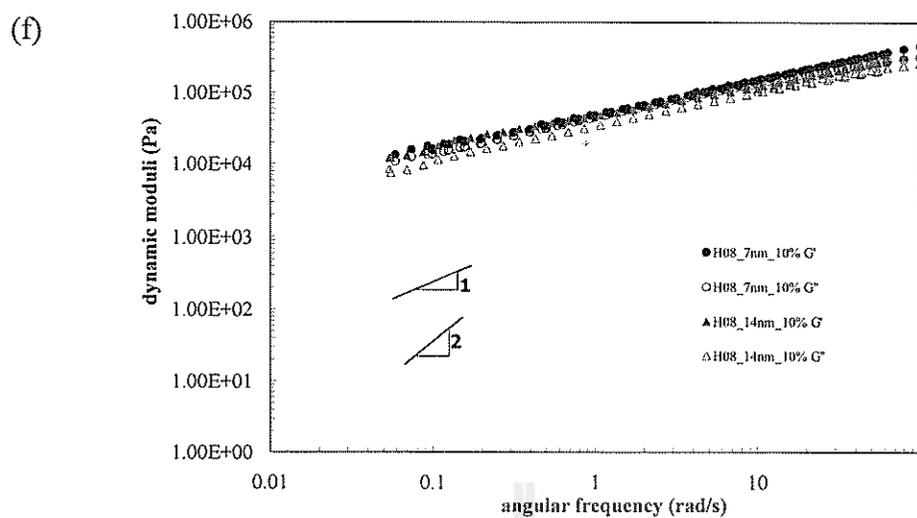
**Figure 4.9** Storage and loss moduli of the fumed silica (7 and 14 nm) filled H08 melts at various contents (wt%) as a function of the angular frequency at the temperature of 160 °C (continued).
