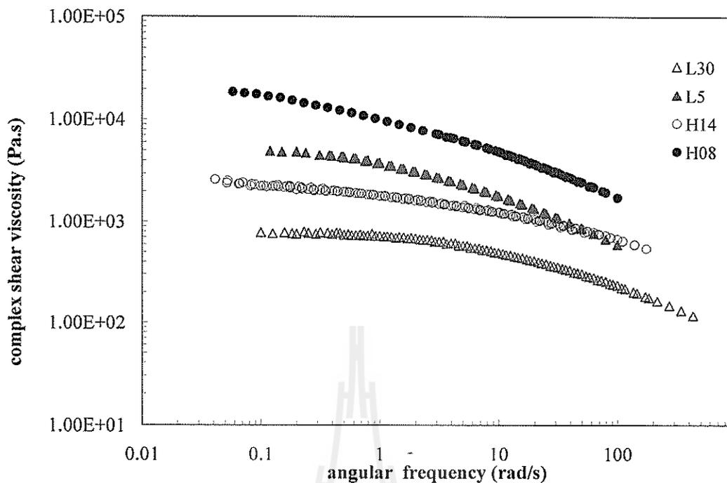
**Figure 4.2** The complex viscosity versus angular frequency for polyethylene melts at the reference temperature of 160°C.
