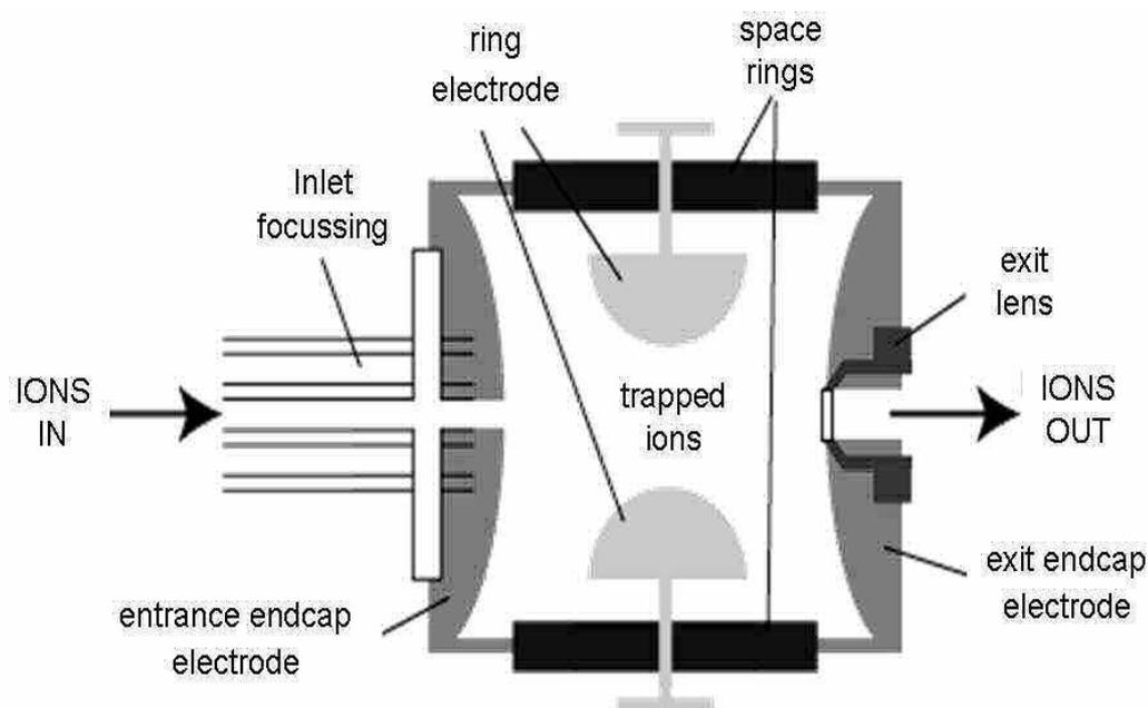
**Figure 2.6** A Schematic (cutaway view) of a quadrupole ion trap mass analyser.
