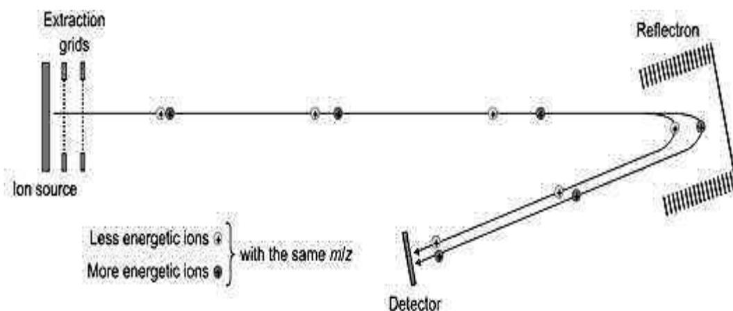
**Figure 2.5** A sketch of a reflectron time-of-flight mass analyzer (Lane, 2005).
