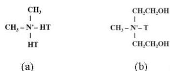
Fig. 1. Chemical structures of the organic modifiers of organoclay: (a) Cloisite<sup>®</sup>20A where HT is hydrogenated tallow (~65% C18; ~30% C16; ~5% C14) and (b) Cloisite<sup>®</sup>30B where T is tallow (~65% C18; ~30% C16; ~5% C14) [8].
