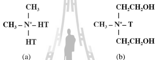
**Figure 3.1** Chemical structures of the organic modifiers of OMMTs: (a) Cloisite<sup>®</sup> 15A and Cloisite<sup>®</sup> 20A where HT is hydrogenated tallow (approximately 65% C-18, 30% C-16, 5% C-14) and (b) Cloisite<sup>®</sup> 30B where T is tallow (approximately 65% C-18, 30% C-16, 5% C-14) (<http://www.scprod.com>).
