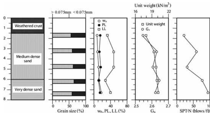
Figure 5. Soil profile of the construction site
