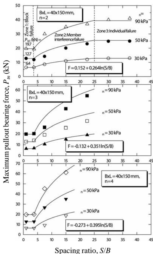
Figure 4. Effect of spacing ratio on pullout bearing resistance of the bearing reinforcement (Horpiulsuk and Niramitkornburee, 2010)
