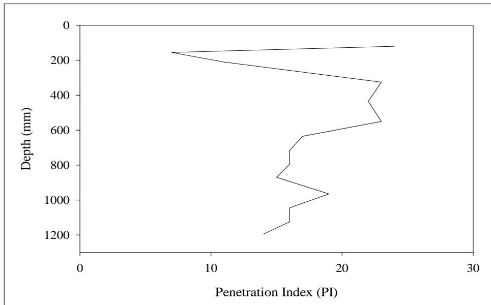
**Figure D.27** PI vs. depth graph for Core#11 at Sikkhawithee 1(a) Road.
