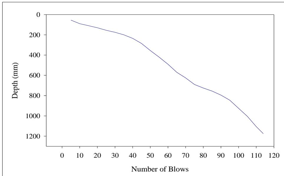
**Figure D.9** Blow vs. depth graph for Core#9 at Withayawithee 2 Road.
