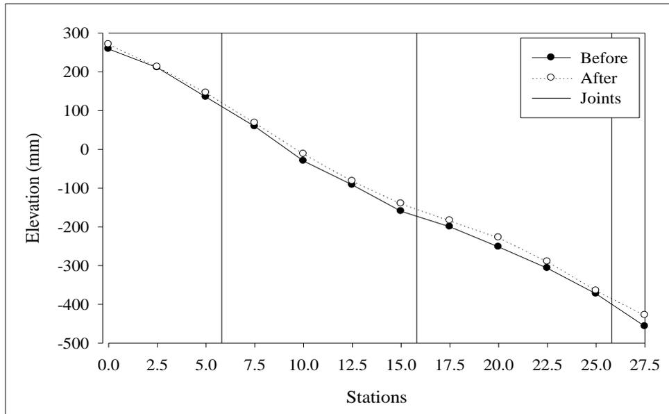
**Figure A.25** Profile leveling before and after polyurethane foam injection on right lane of Sikkhawithee 1(a) Road.
