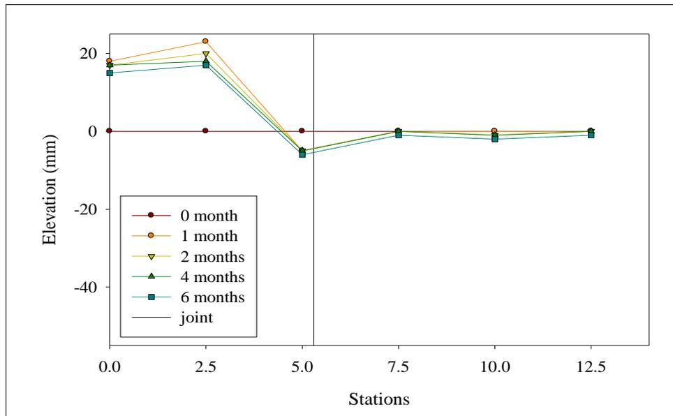
**Figure 4.15** Differential settlement on the right lane of Sikkhawithee 1(b) Road during the study period.
