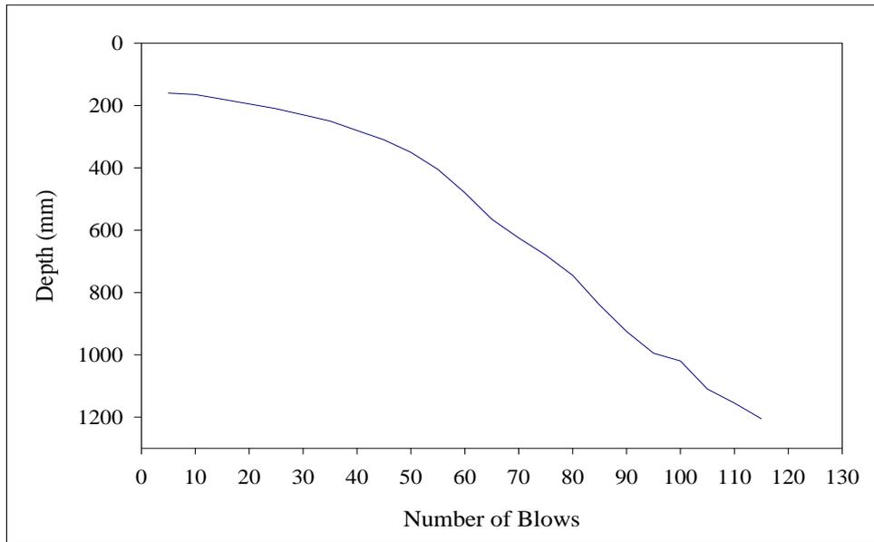
**Figure D.5** Blow vs. depth graph for Core#5 at Withayawithee 2 Road.
