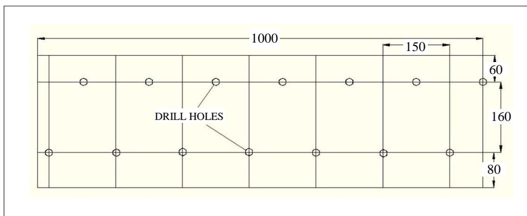
**Figure 4.1** Layout of drill holes (dimension in cm).
