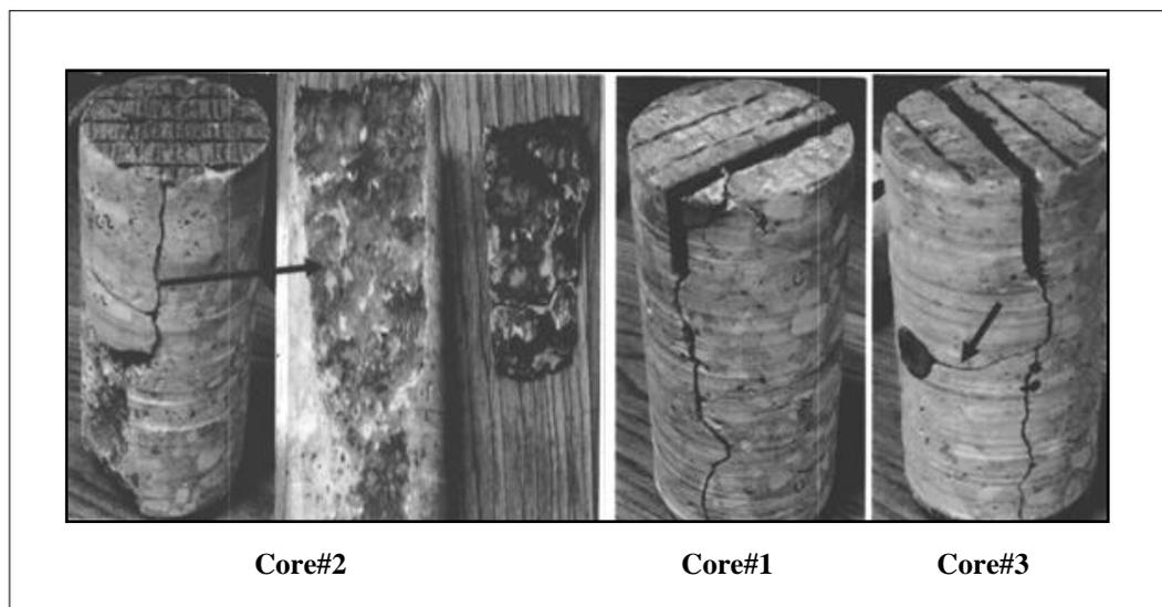
**Figure 2.3** (Left) Core#2 condition as cracks appear to have had formed long ago. (Right) Condition of Core#1 and Core#3 as the mid-depth horizontal crack near the dowel bar was due to the locking action (Chen and Won, 2007).
