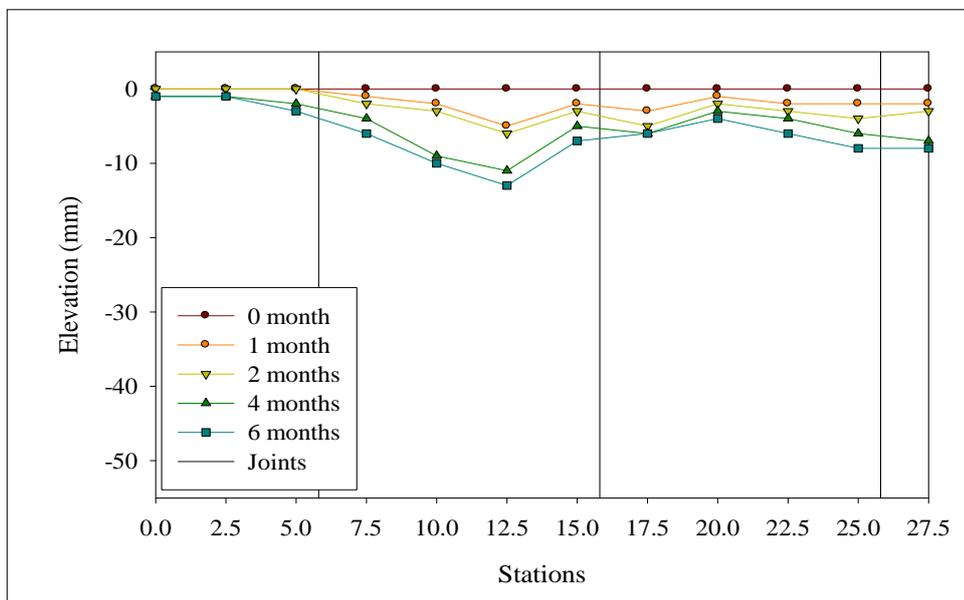
**Figure A.24** Differential settlement at the middle of lanes at Sikkhawithee 1(a) Road during the study period.
