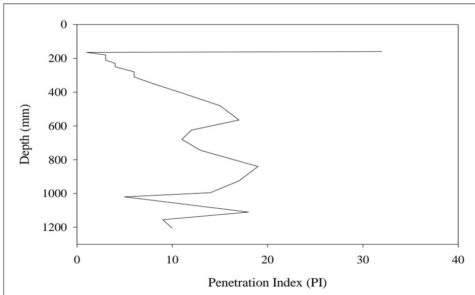
**Figure D.21** PI vs. depth graph for Core#5 at Withayawithee 2 Road.
