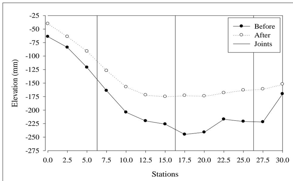
**Figure A.16** Profile leveling before and after polyurethane foam injection on right lane of Withayawithee 3 Road.
