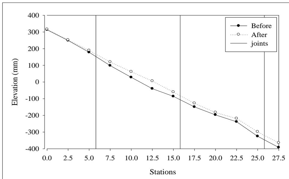
**Figure A.22** Profile leveling before and after polyurethane foam injection at the middle of lanes of Sikkhawithee 1(a) Road.
