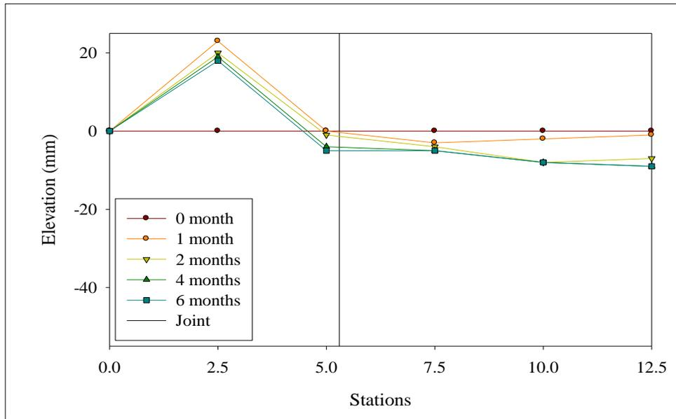
**Figure A.33** Differential settlement at the middle of lanes of Sikkhawithee 1(b) Road during the study period.
