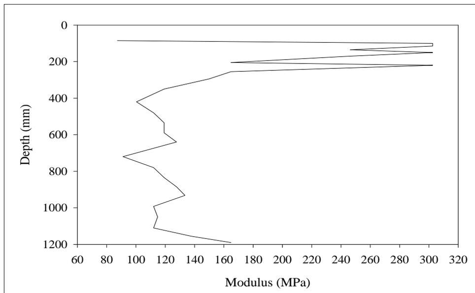
**Figure D.38** Modulus of subgrade reaction from Core#6 at Withayawithee 2 Road.
