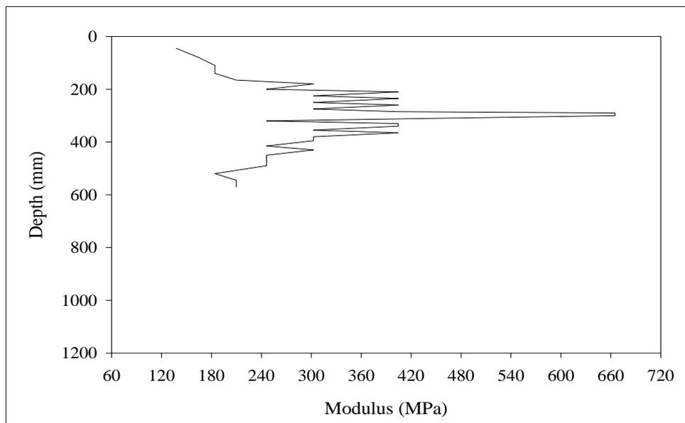
**Figure D.42** Modulus of subgrade reaction from Core#10 at Withayawithee 2 Road.
