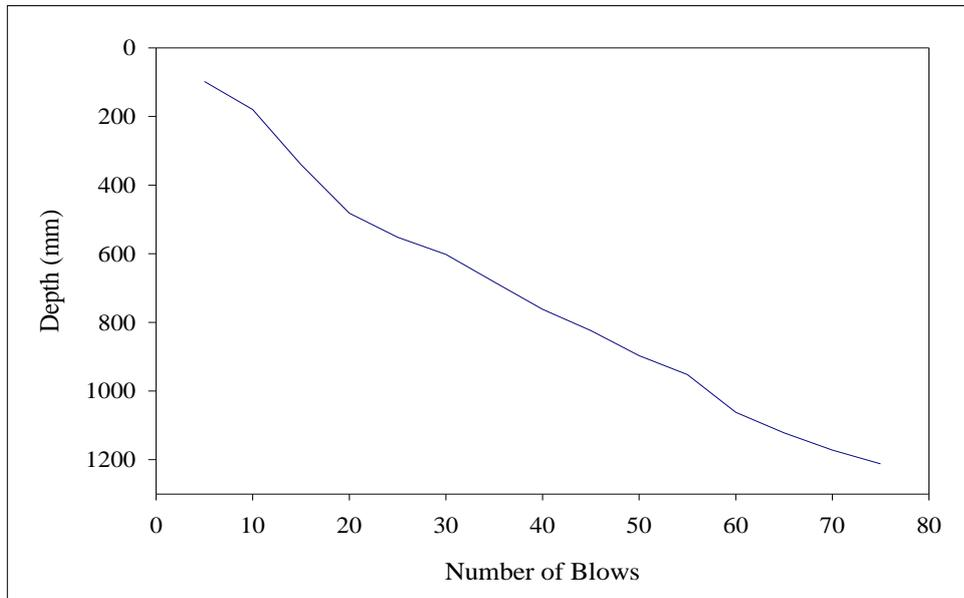
**Figure D.7** Blow vs. depth graph for Core#7 at Withayawithee 2 Road.
