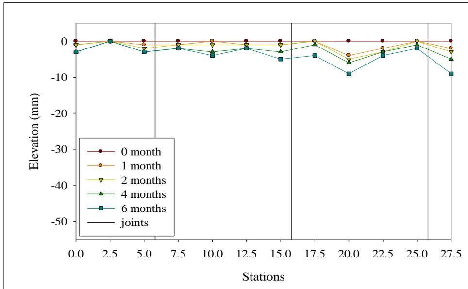
**Figure A.27** Differential settlement on right lane of Sikkhawithee 1(a) Road during the study period.
