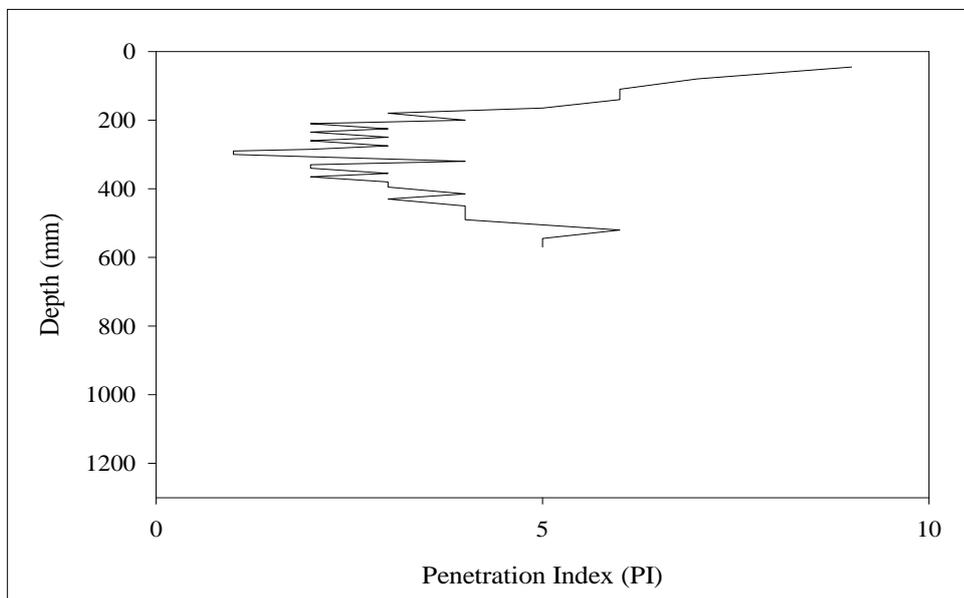
**Figure D.26** PI vs. depth graph for Core#10 at Withayawithee 2 Road.
