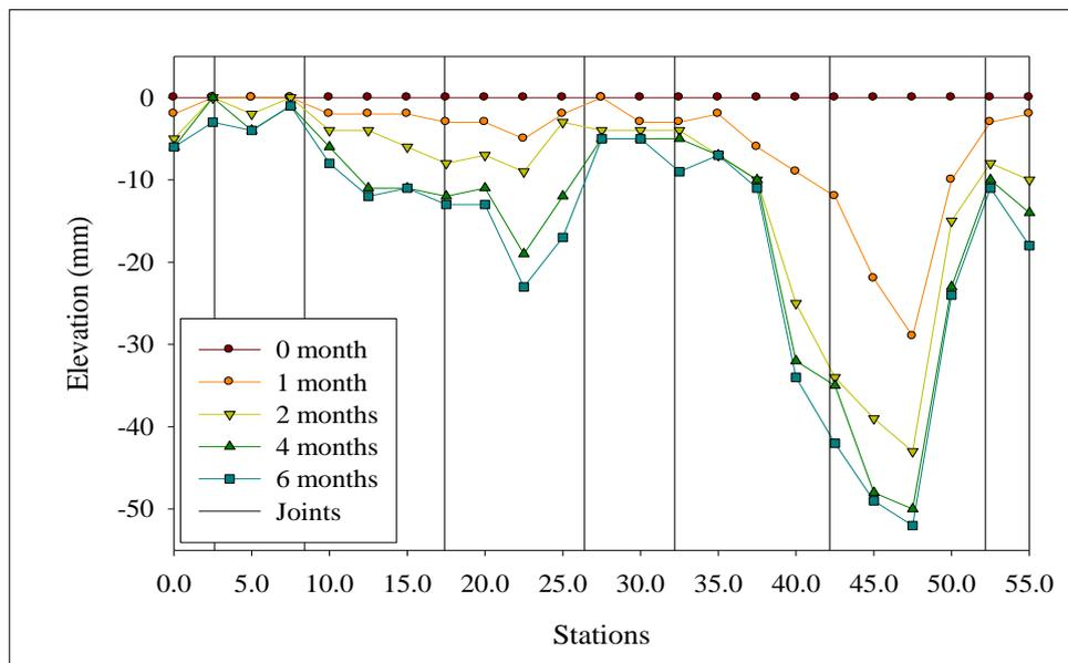
**Figure A.9** Differential settlement on right lane of Withayawithee 2 Road during the study period.
