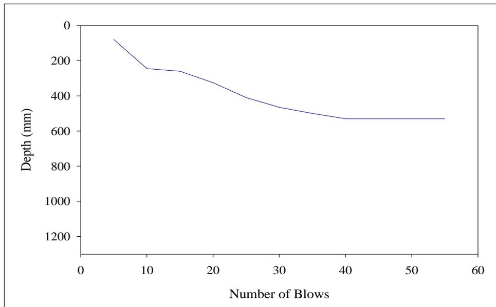
**Figure D.15** Blow vs. depth graph for Core#15 at Sikkhawithee 1(b) Road.
