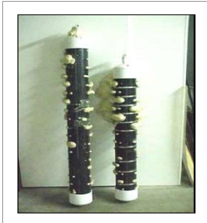
**Figure 2.2** Penetration tubes after injection (Soltesz, 2002).
