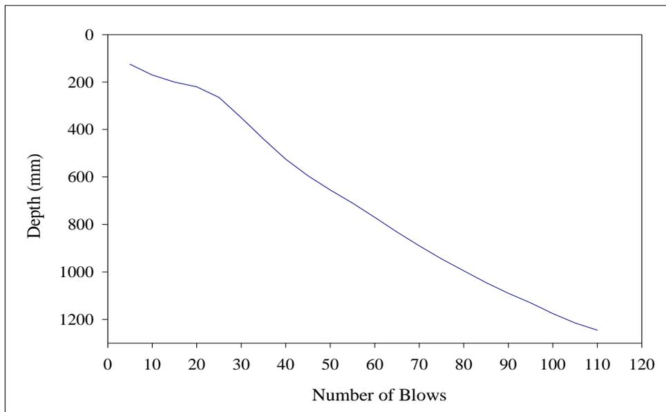
**Figure D.12** Blow vs. depth graph for Core#12 at Sikkhawithee 1(a) Road.
