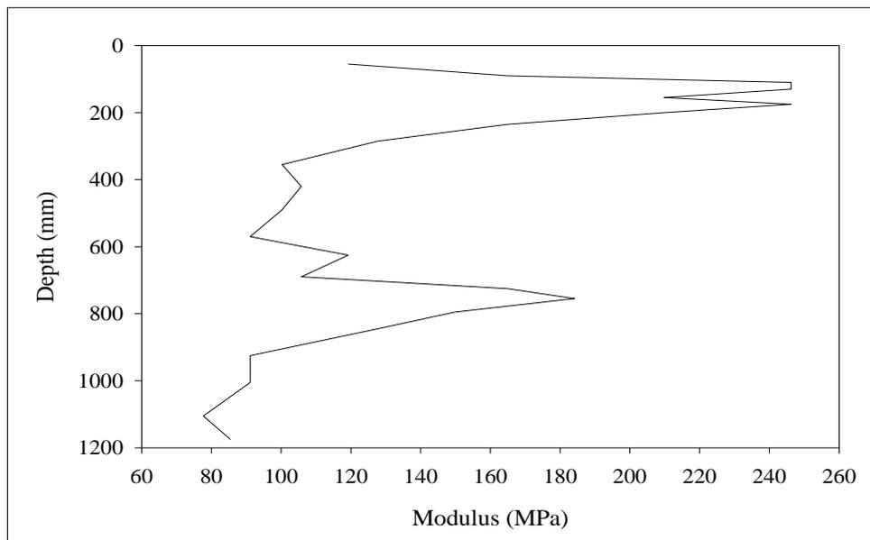
**Figure D.41** Modulus of subgrade reaction from Core#9 at Withayawithee 2 Road.
