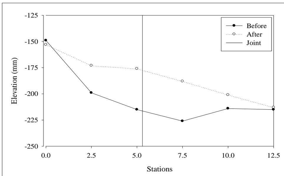
**Figure A.28** Profile leveling before and after polyurethane foam injection on left lane of Sikkhawithee 1(b) Road.
