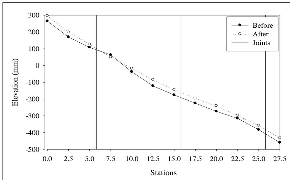
**Figure A.19** Profile leveling before and after polyurethane foam injection on left lane of Sikkhawithee 1(a) Road.
