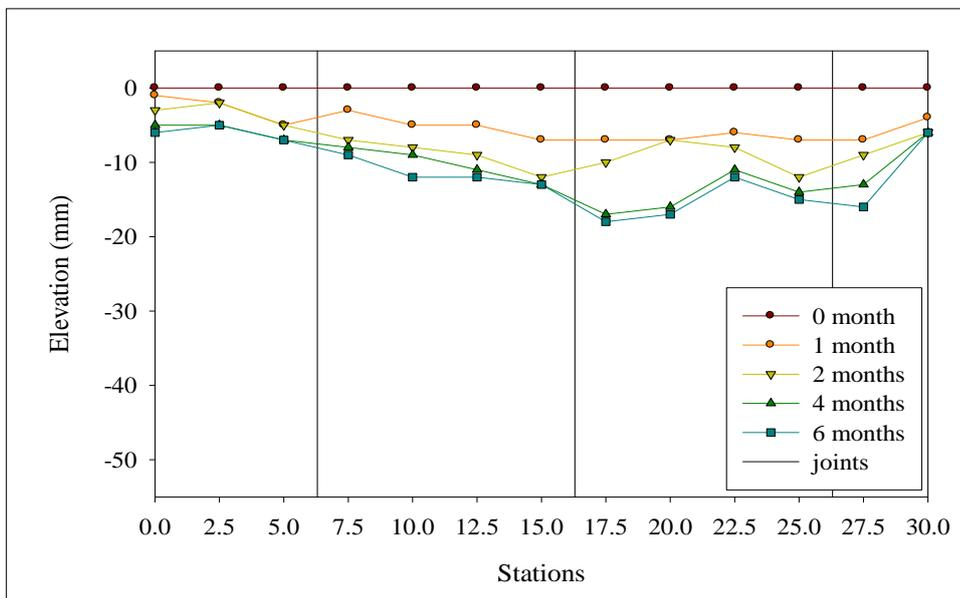
**Figure A.18** Differential settlement on right lane of Withayawithee 3 Road during the study period.
