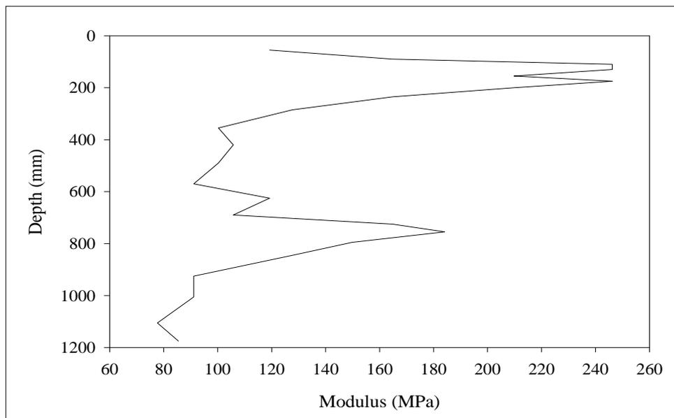
**Figure 4.30** Modulus of subgrade reaction from Core#9 at Withayawithee 2 Road.
