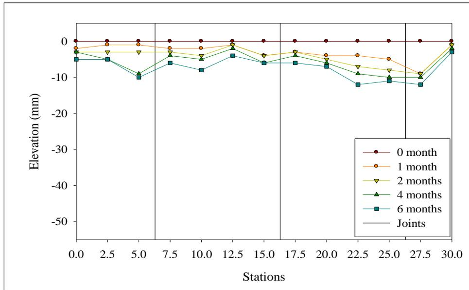
**Figure A.15** Differential settlement at the middle of lanes of Withayawithee 3 Road during the study period.
