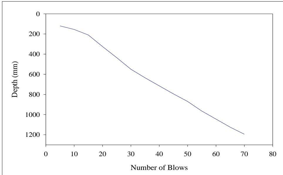
**Figure D.11** Blow vs. depth graph for Core#11 at Sikkhawithee 1(a) Road.
