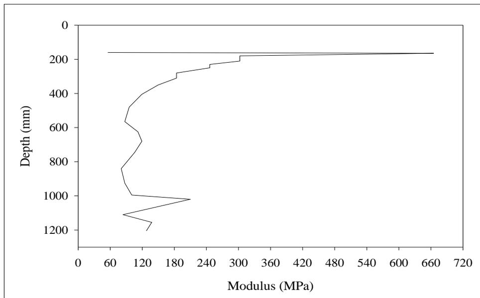
**Figure D.37** Modulus of subgrade reaction from Core#5 at Withayawithee 2 Road.
