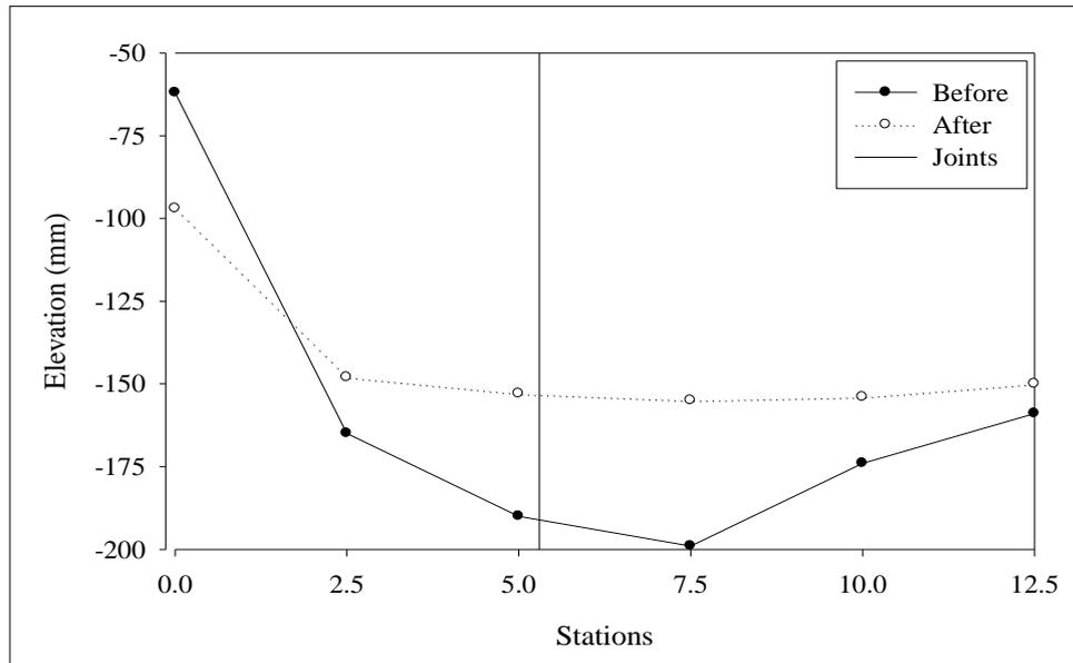
**Figure A.31** Profile leveling before and after polyurethane foam injection at the middle of lanes of Sikkhawithee 1(b) Road.
