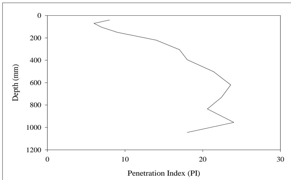
**Figure D.20** PI vs. depth graph for Core#4 at Withayawithee 3 Road.
