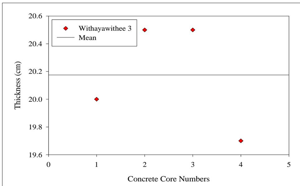
**Figure C.2** Variation of concrete core thickness and its mean at Withayawithee 3 Road.
