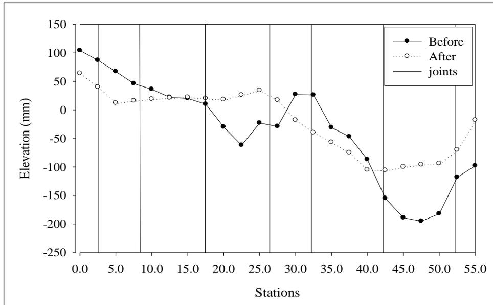
**Figure A.7** Profile leveling before and after polyurethane foam injection on right lane of Withayawithee 2 Road.
