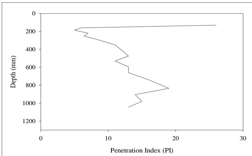
**Figure D.24** PI vs. depth graph for Core#8 at Withayawithee 2 Road.
