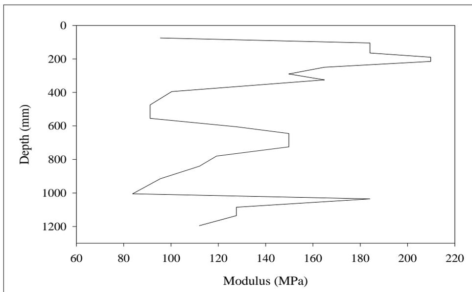
**Figure D.46** Modulus of subgrade reaction from Core#14 at
