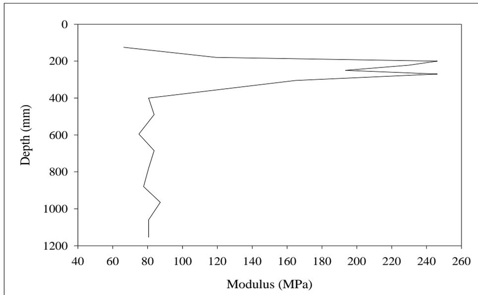
**Figure D.33** Modulus of subgrade reaction from Core#1 at Withayawithee 3 Road.
