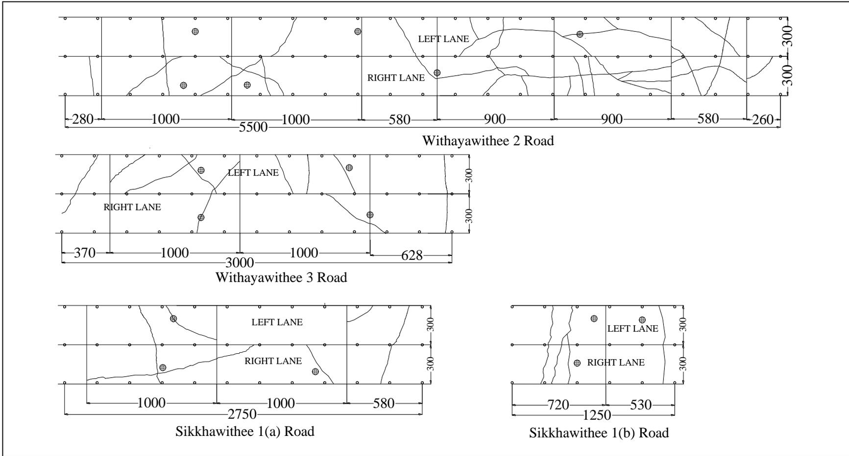
**Figure B.1** Distress map for all the four section (showing linear cracks).
