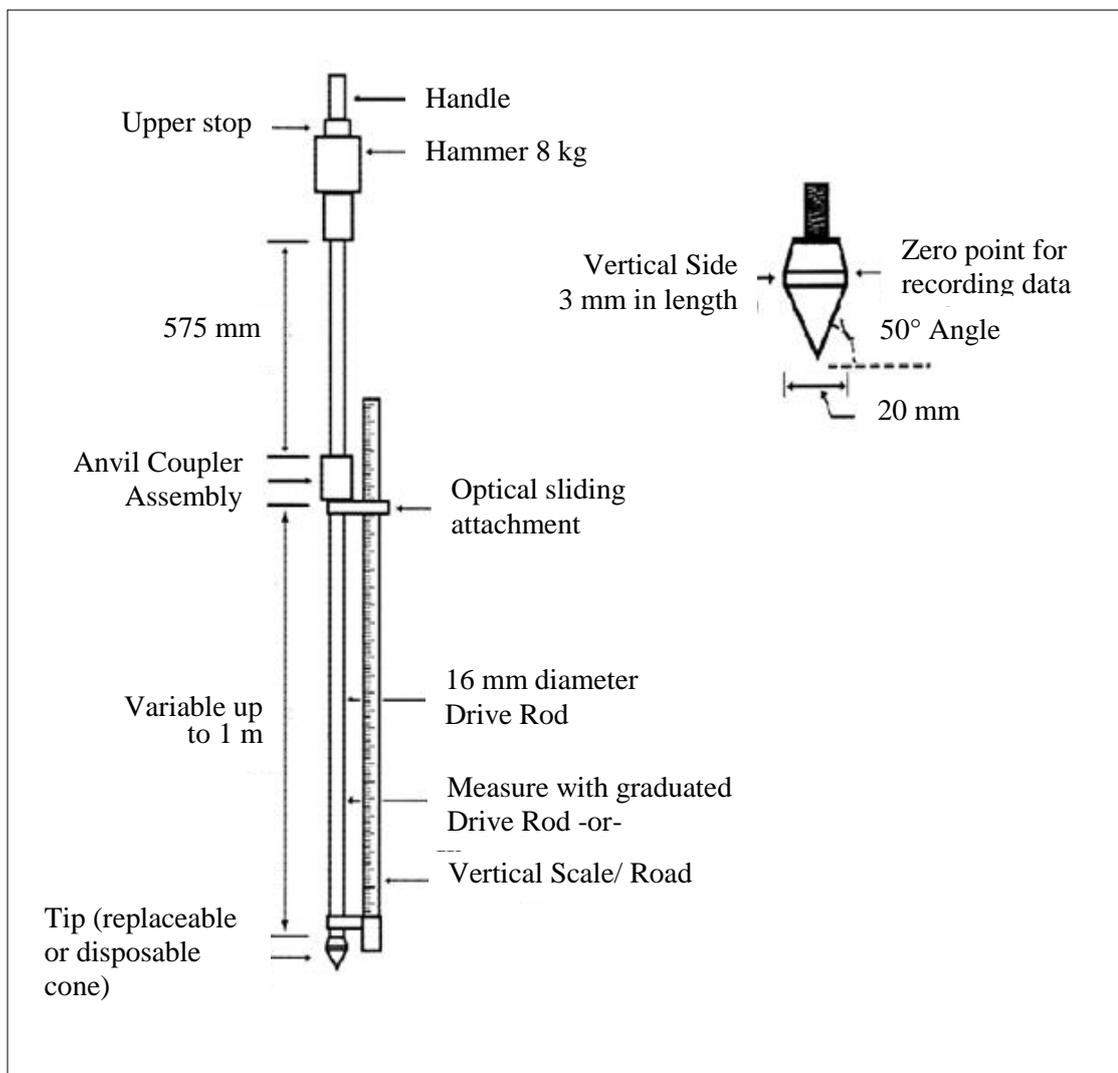
**Figure 3.2** The Dynamic Cone Penetrometer (modified from ASTM D6951).
