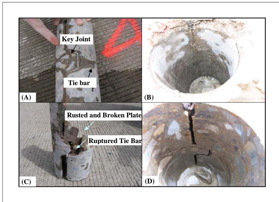
**Figure 2.4** Comparisons of the key joint conditions (A) Core showing good core with key joint configuration. (B) Core hole condition- joint width is very tight and no settlement. (C) Core showing broken core with rusted plate and ruptured tie bar. (D) Core hole condition-joint width is much wider and with statement (Chen et al., 2009).
