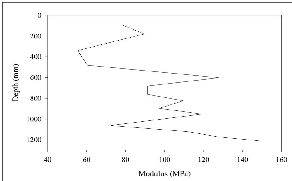
**Figure 4.31** Modulus of subgrade reaction from Core#7 at Withayawithee 2 Road.
