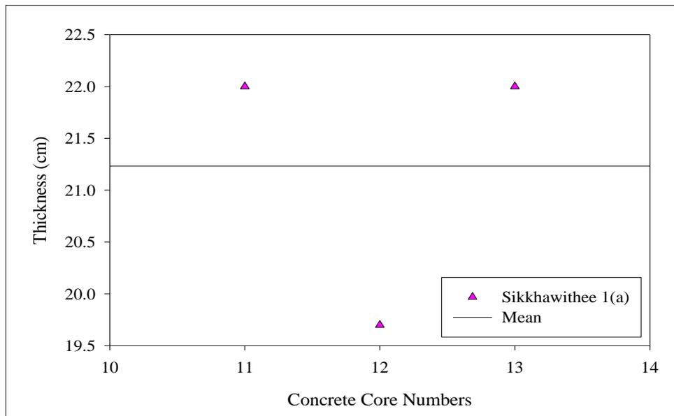
**Figure C.3** Variation of concrete core thickness and its mean at Sikhawithee 1(a) Road.
