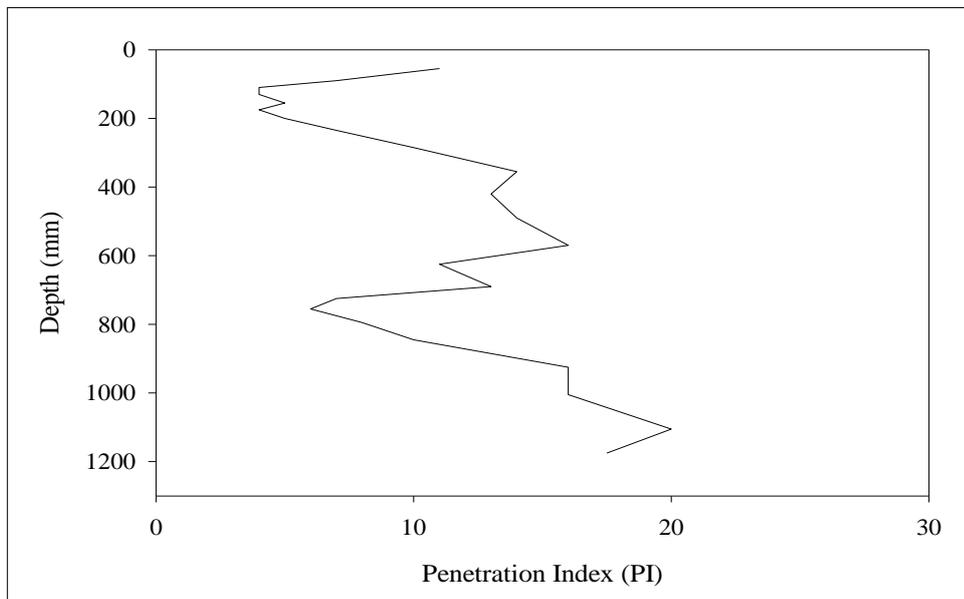
**Figure D.25** PI vs. depth graph for Core#9 at Withayawithee 2 Road.
