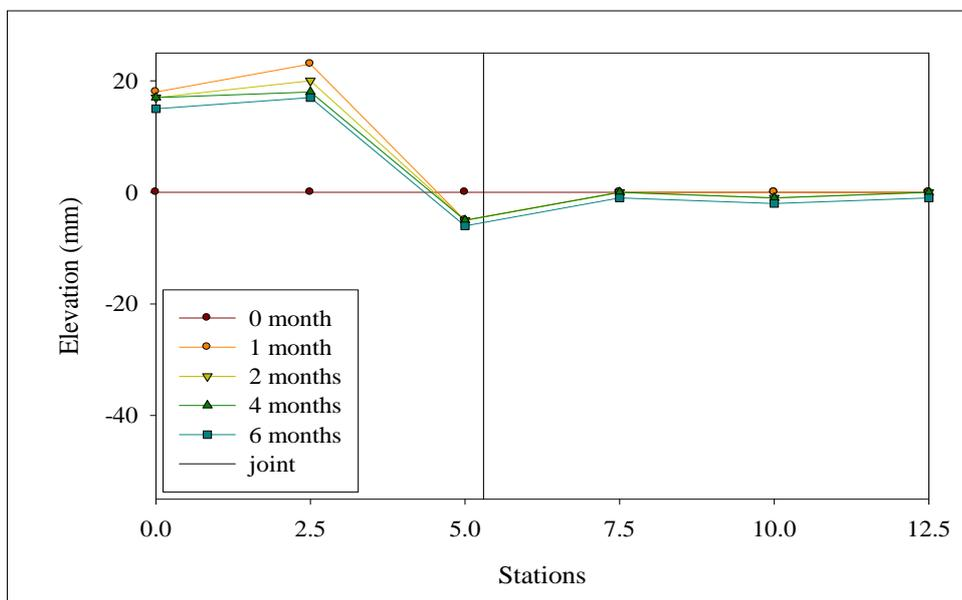
**Figure A.36** Differential settlement on right lane of Sikkhawithee 1(b) Road during the study period.
