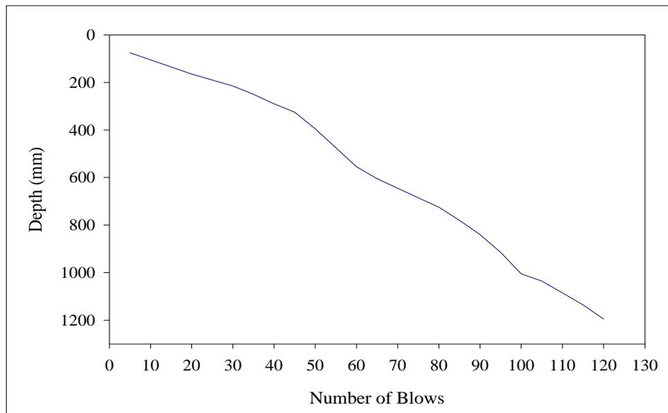
**Figure D.14** Blow vs. depth graph for Core#14 at Sikkhawithee 1(b) Road.
