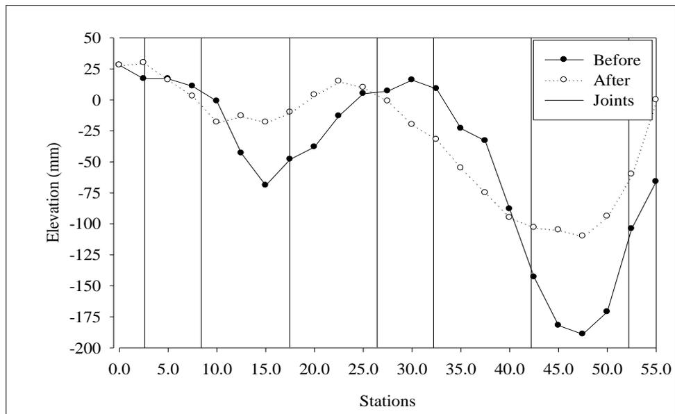
**Figure A.1** Profile leveling before and after polyurethane foam injection on left lane of Withayawithee 2 Road.
