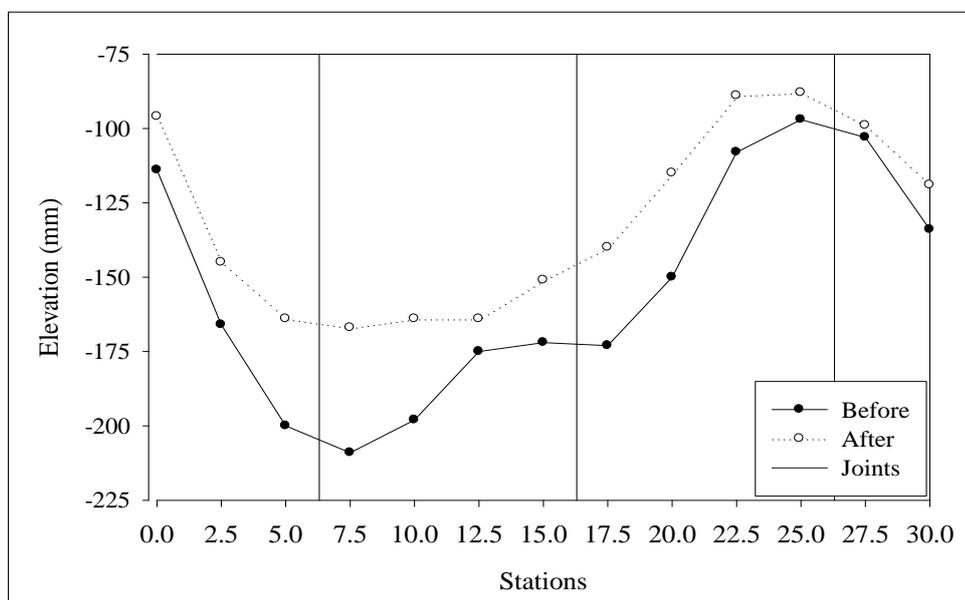
**Figure A.10** Profile leveling before and after polyurethane foam injection on left lane of Withayawithee 3 Road.
