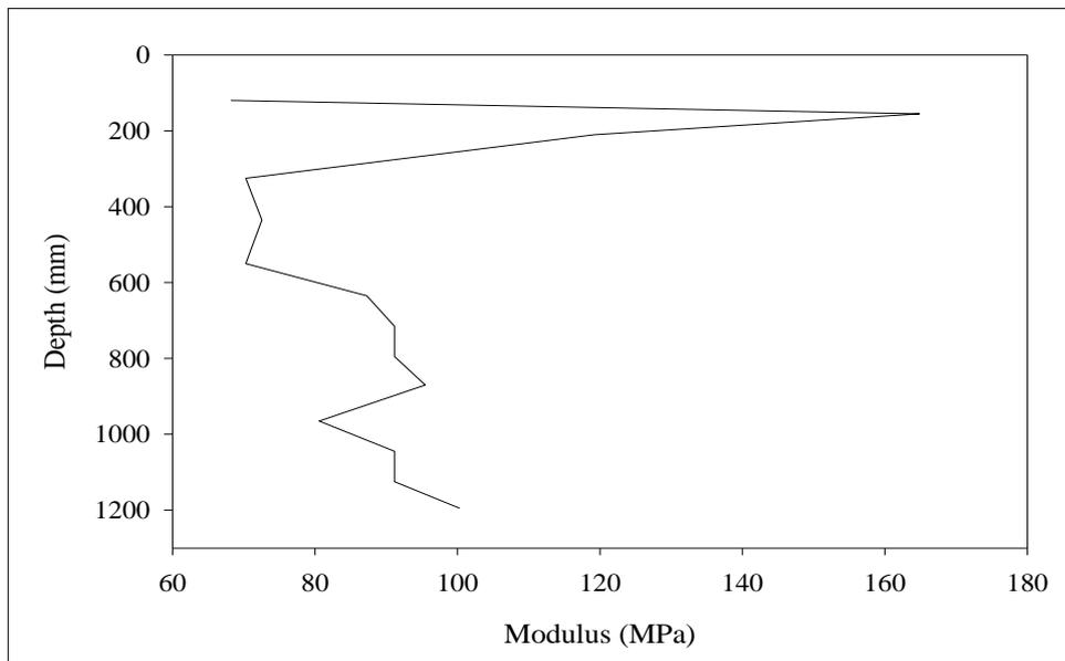
**Figure D.43** Modulus of subgrade reaction from Core#11 at
