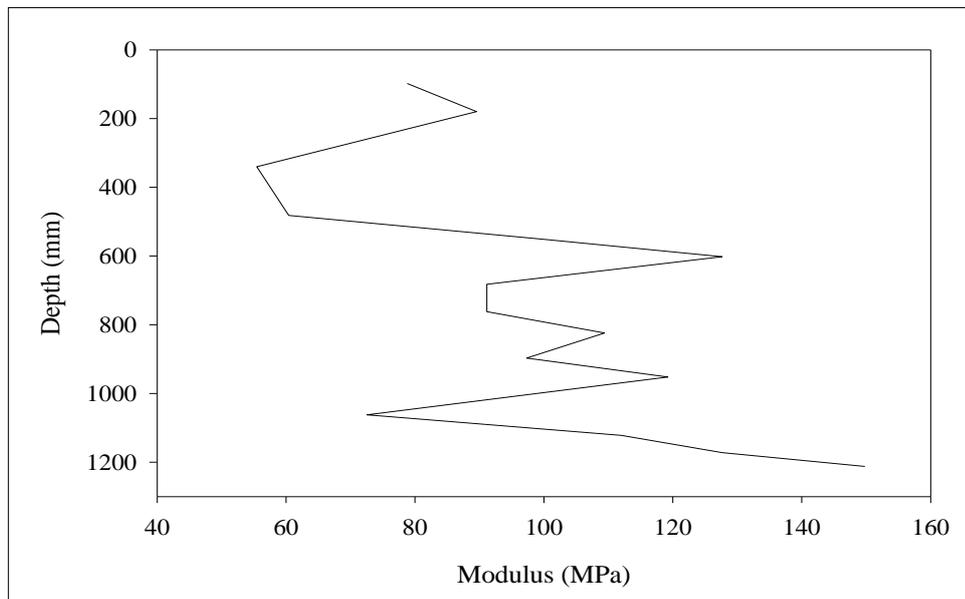
**Figure D.39** Modulus of subgrade reaction from Core#7 at Withayawithee 2 Road.
