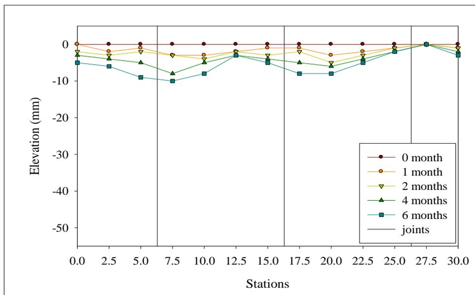
**Figure A.12** Differential settlement on left lane of Withayawithee 3 Road during the study period.
