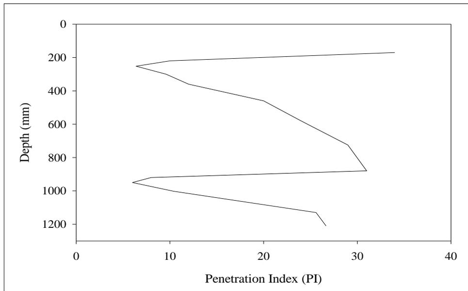
**Figure D.19** PI vs. depth graph for Core#3 at Withayawithee 3 Road.
