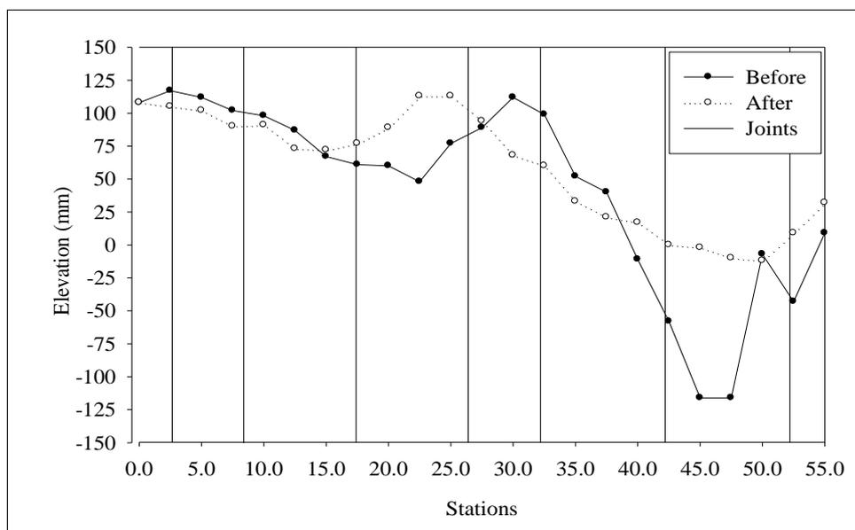
**Figure A.4** Profile leveling before and after polyurethane foam injection at the middle of lanes of Withayawithee 2 Road.
