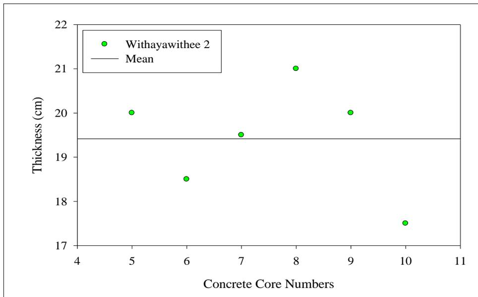
**Figure C.1** Variation of concrete core thickness and its mean at Withayawithee 2 Road.
