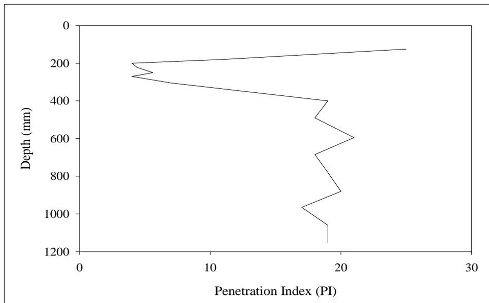
**Figure D.17** PI vs. depth graph for Core#1 at Withayawithee 3 Road.
