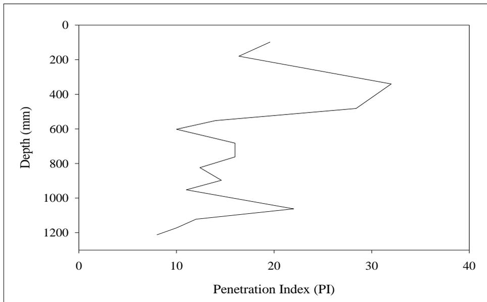
**Figure D.23** PI vs. depth graph for Core#7 at Withayawithee 2 Road.
