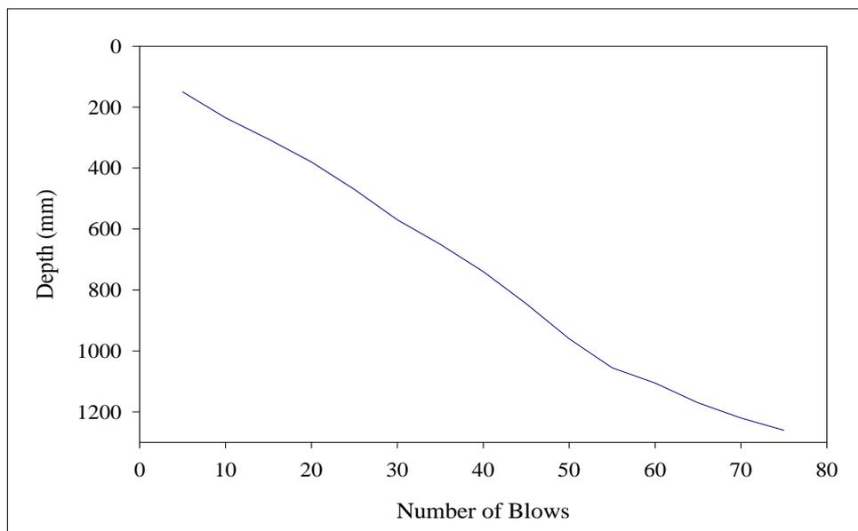
**Figure D.16** Blow vs. depth graph for Core#16 at Sikkhawithee 1(b) Road.
