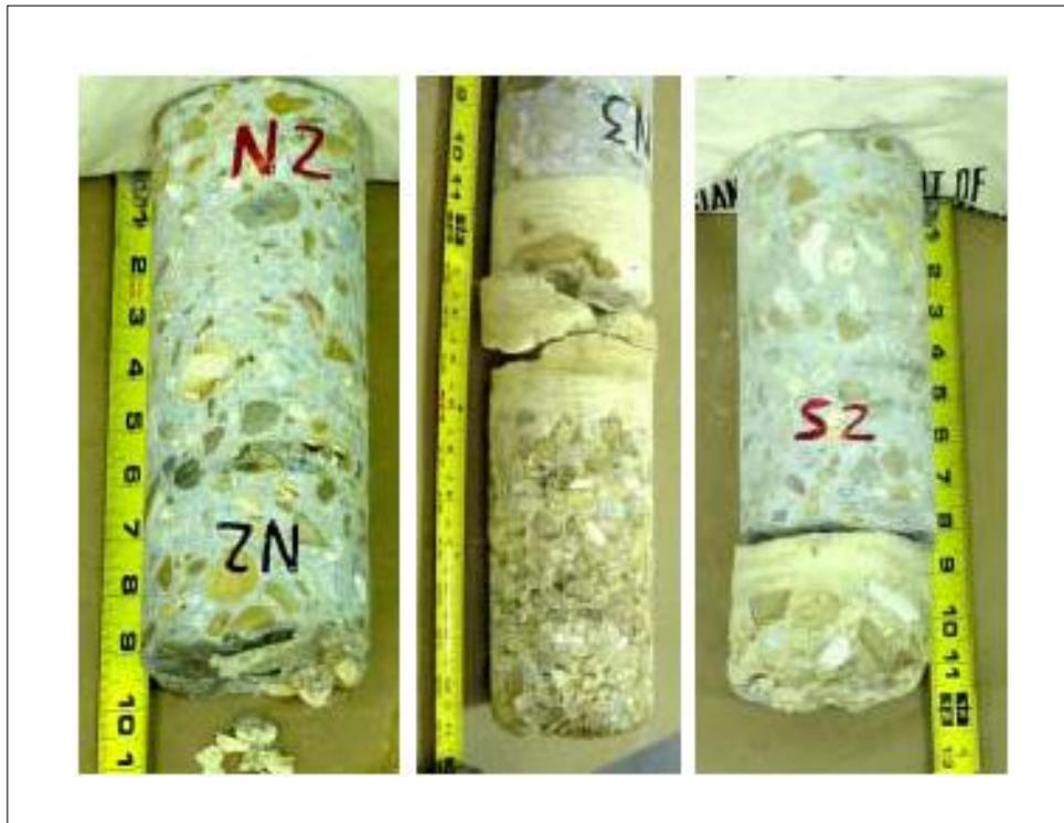
**Figure 2.5** Concrete cores with polyurethane (Gaspard and Morvant, 2004).
