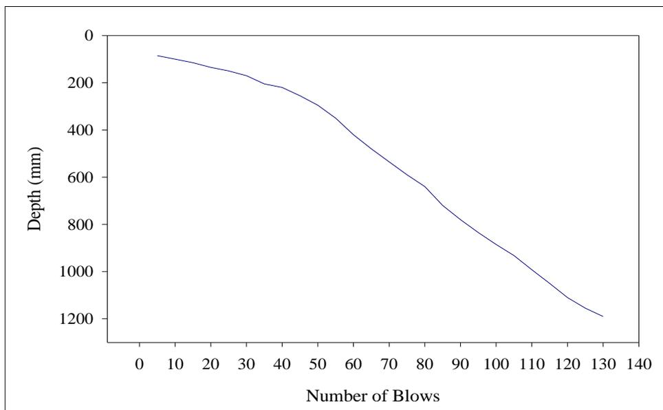
**Figure D.6** Blow vs. depth graph for Core#6 at Withayawithee 2 Road.
