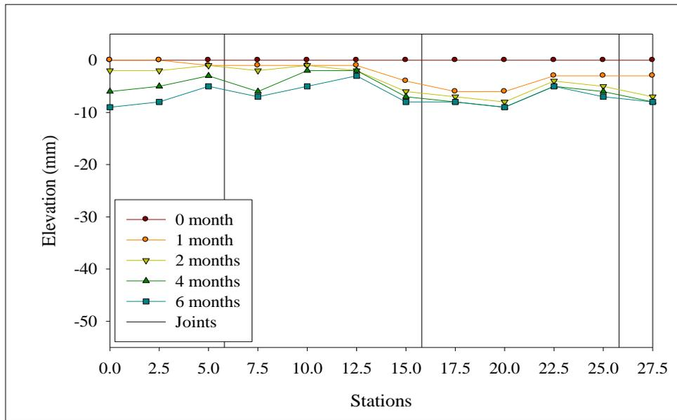
**Figure A.21** Differential settlement on left lane of Sikkhawithee 1(a) Road during the study period.
