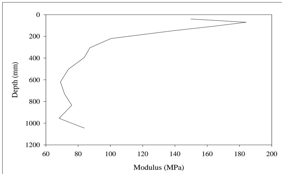
**Figure D.36** Modulus of subgrade reaction from Core#4 at Withayawithee 3 Road.
