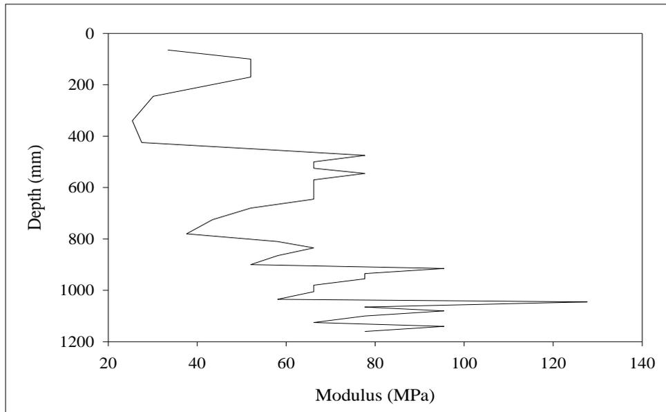
**Figure D.45** Modulus of subgrade reaction from Core#13 at
