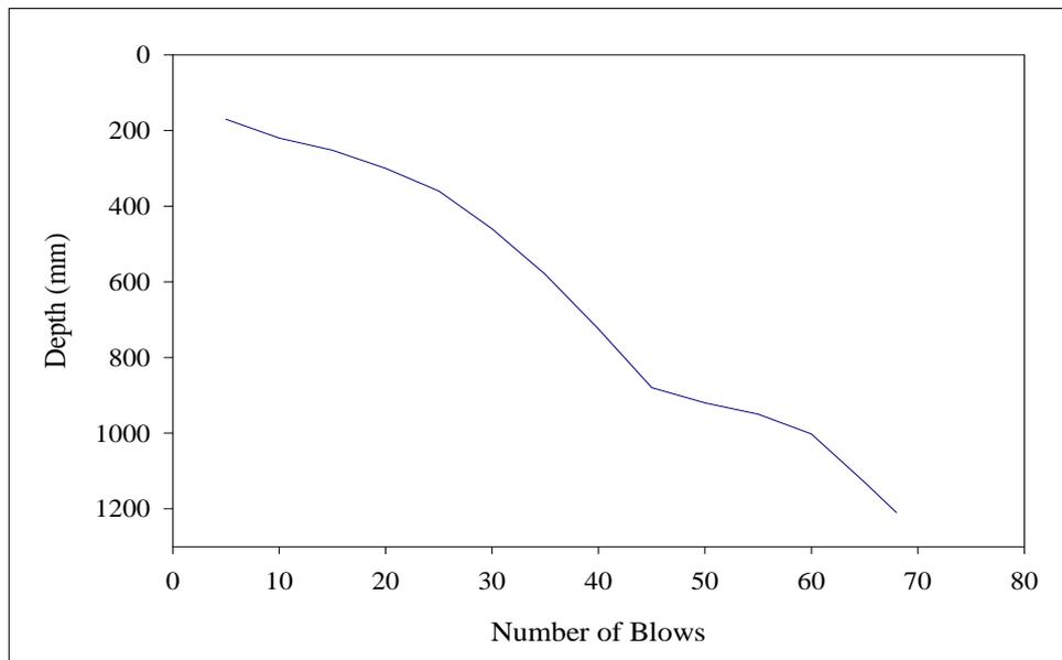
**Figure D.3** Blow vs. depth graph for Core#3 at Withayawithee 3 Road.
