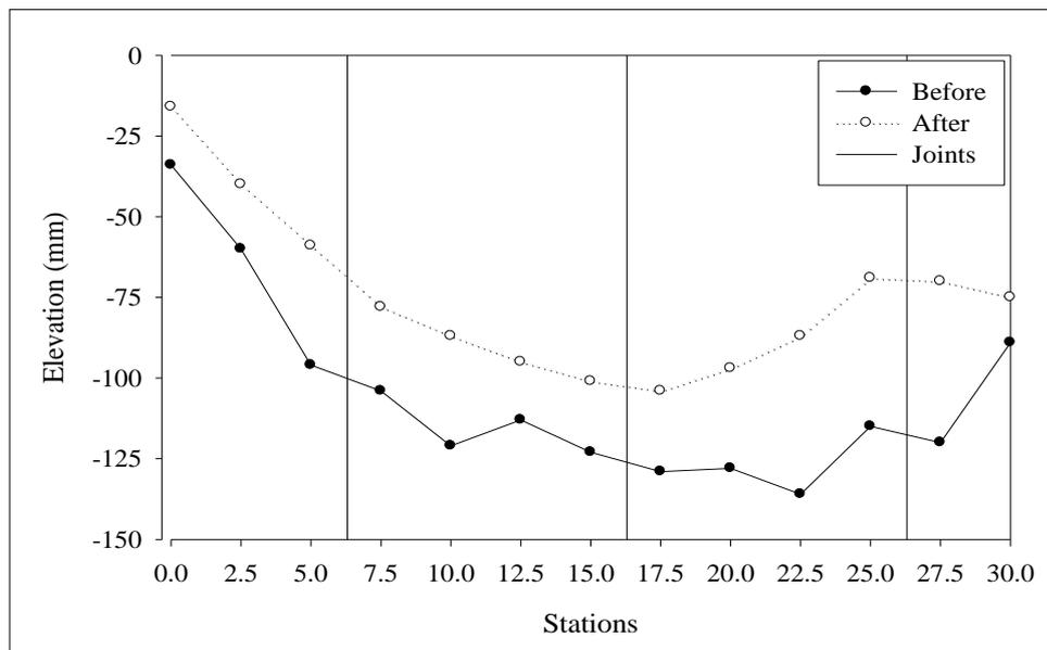
**Figure A.13** Profile leveling before and after polyurethane foam injection at the middle of lanes of Withayawithee 3 Road.
