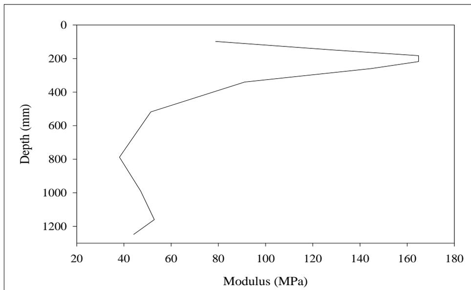
**Figure D.34** Modulus of subgrade reaction from Core#2 at Withayawithee 3 Road.
