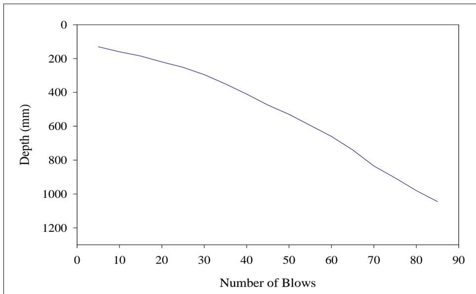
**Figure D.8** Blow vs. depth graph for Core#8 at Withayawithee 2 Road.
