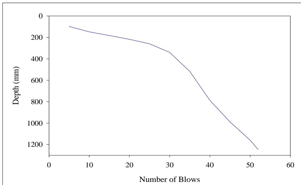
**Figure D.2** Blow vs. depth graph for Core#2 at Withayawithee 3 Road.
