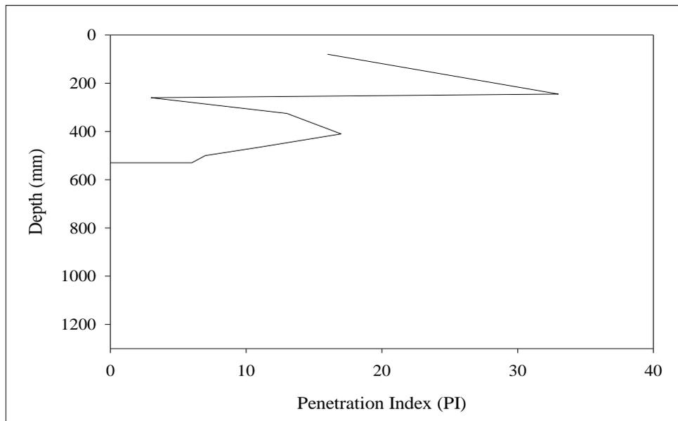
**Figure D.31** PI vs. depth graph for Core#15 at Sikkhawithee 1(a) Road.
