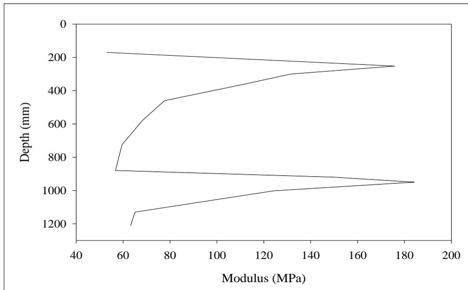
**Figure D.35** Modulus of subgrade reaction from Core#3 at Withayawithee 3 Road.
