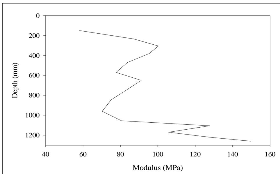
**Figure D.48** Modulus of subgrade reaction from Core#16 at Sikhawithee 1(b) Road.
