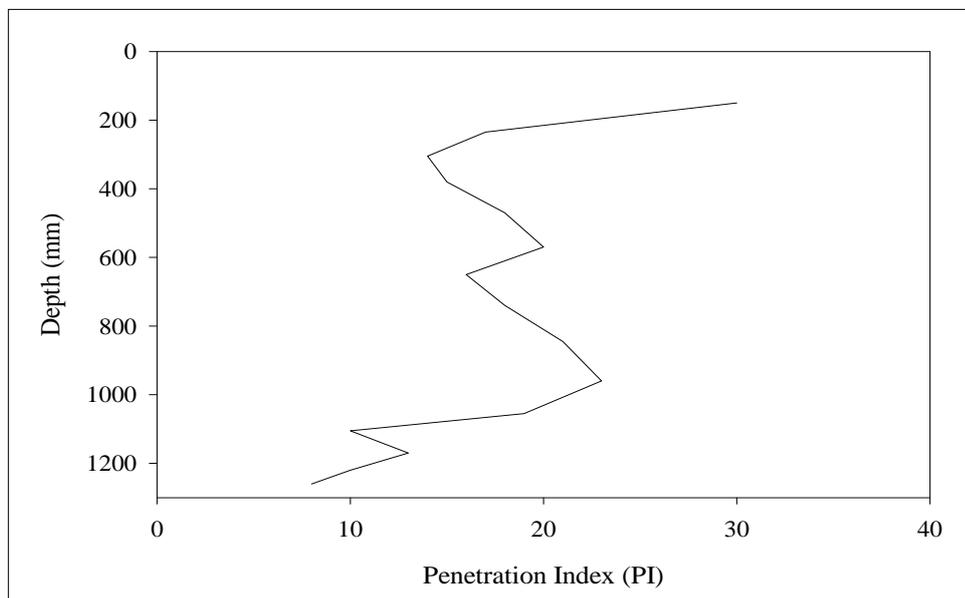
**Figure D.32** PI vs. depth graph for Core#16 at Sikkhawithee 1(b) Road.
