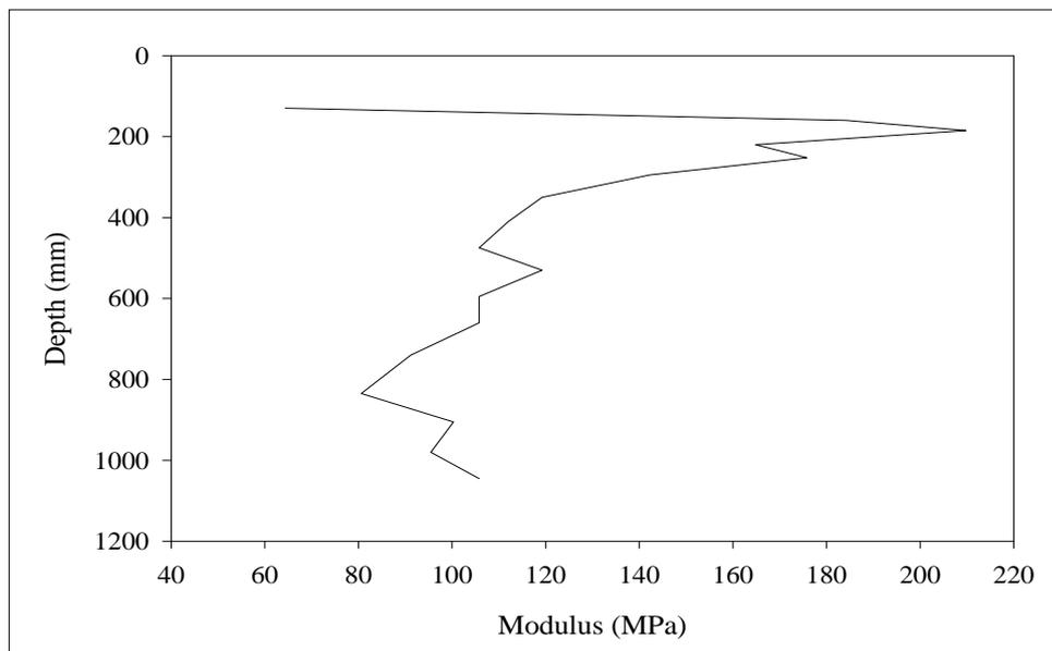
**Figure D.40** Modulus of subgrade reaction from Core#8 at Withayawithee 2 Road.
