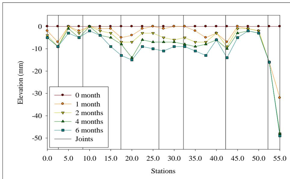
**Figure A.3** Differential settlement on left lane of Withayawithee 2 Road during the study period.
