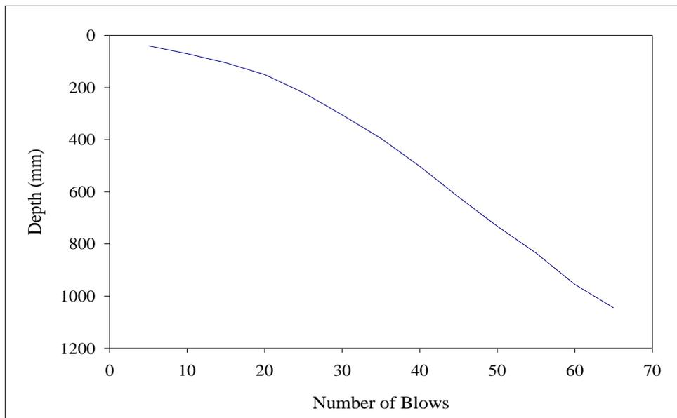
**Figure D.4** Blow vs. depth graph for Core#4 at Withayawithee 3 Road.
