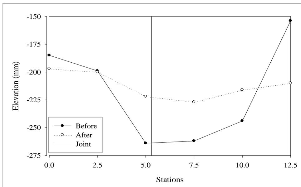
**Figure A.34** Profile leveling before and after polyurethane foam injection on right lane of Sikkhawithee 1(b) Road.
