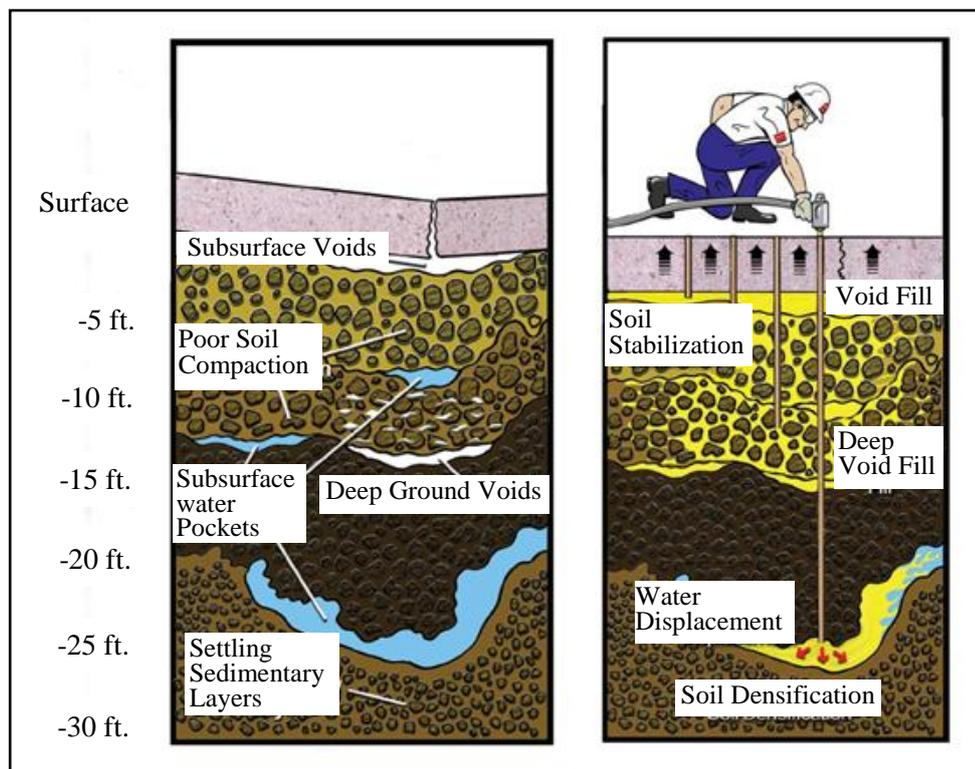
**Figure 2.1** (Left) Elements of a shifting/unstable/damaged underground base and (Right) the polyurethane material injection (Uretek USA, 2004).
