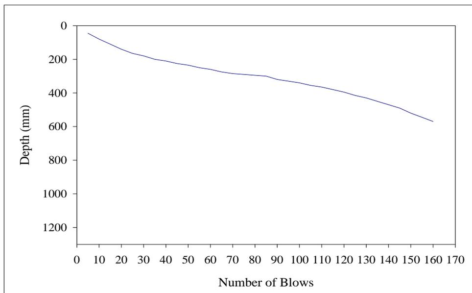
**Figure D.10** Blow vs. depth graph for Core#10 at Withayawithee 2 Road.
