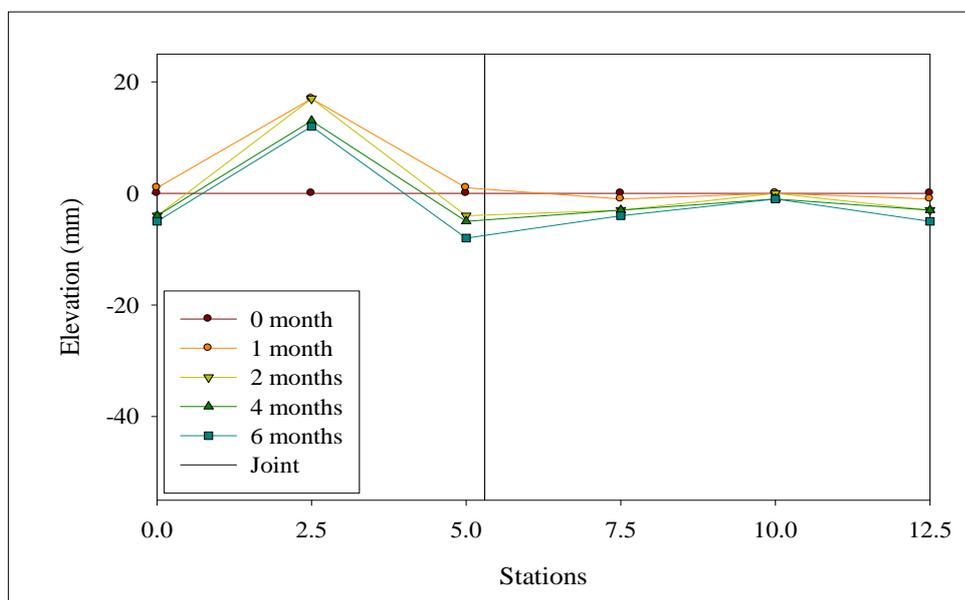
**Figure A.30** Differential settlement on left lane of Sikkhawithee 1(b) Road during the study period.
