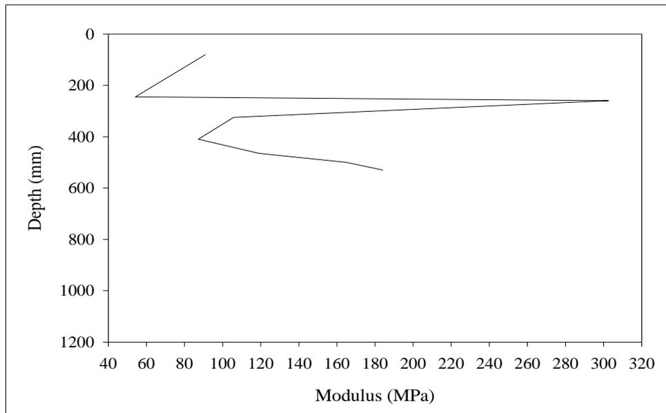
**Figure D.47** Modulus of subgrade reaction from Core#15 at Sikhawithee 1(b) Road.
