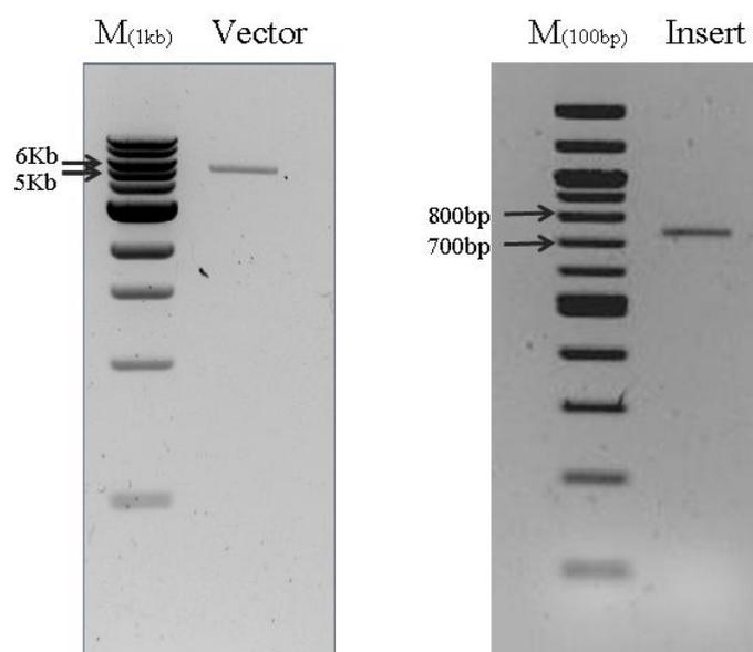
**Figure 18.** Agarose gel analysis of *NcoI* and *NotI* digestion products. M, 1 kb DNA ladder and 100 bp ladder. A vector (pKP300 $\Delta$ III) and insert (scFv-F6) band can be seen at approximately 5,000 bp and 800 bp, respectively. The concentration of DNA of vector and insert were 12.1  $\mu$ g/ml and 12.3  $\mu$ g/ml, respectively.
