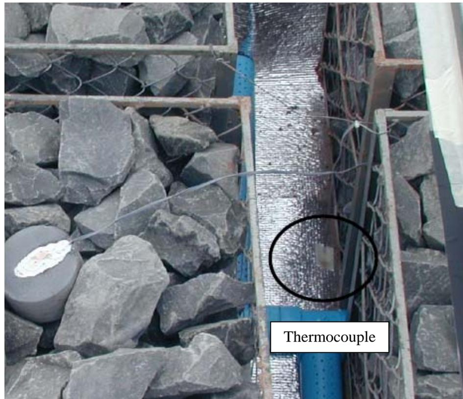
**Figure 5.5** Thermocouple was mounted on a glass sheet and hung in the air to monitor the temperature of pit air.
