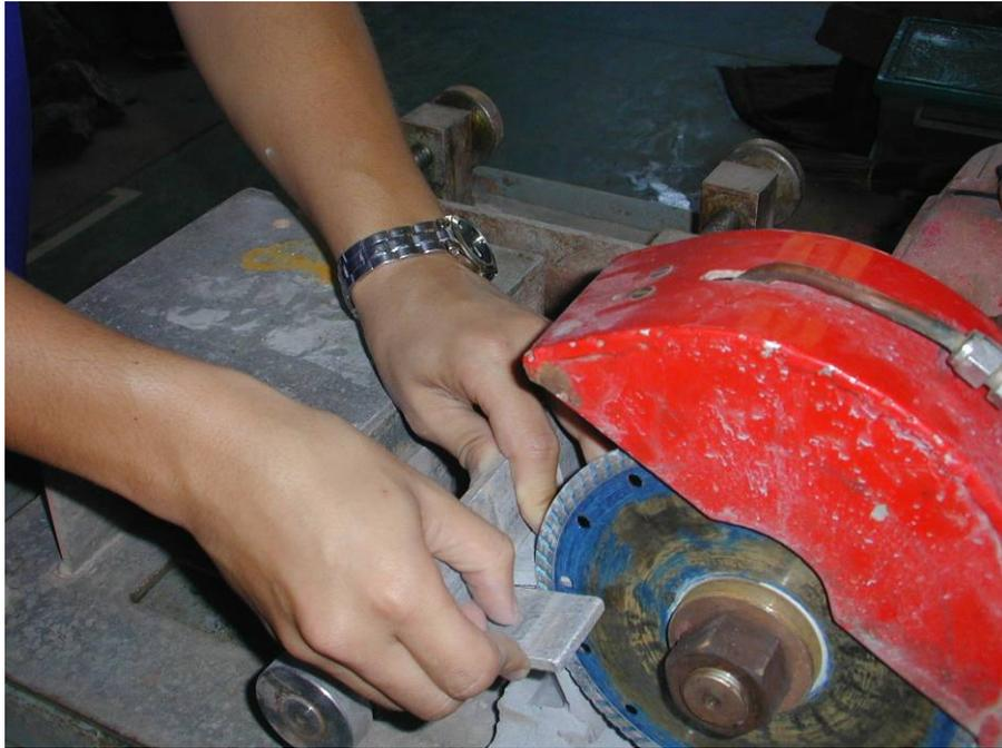
**Figure 3.2** Rock sample is cut to obtain the desired geometry and size.
