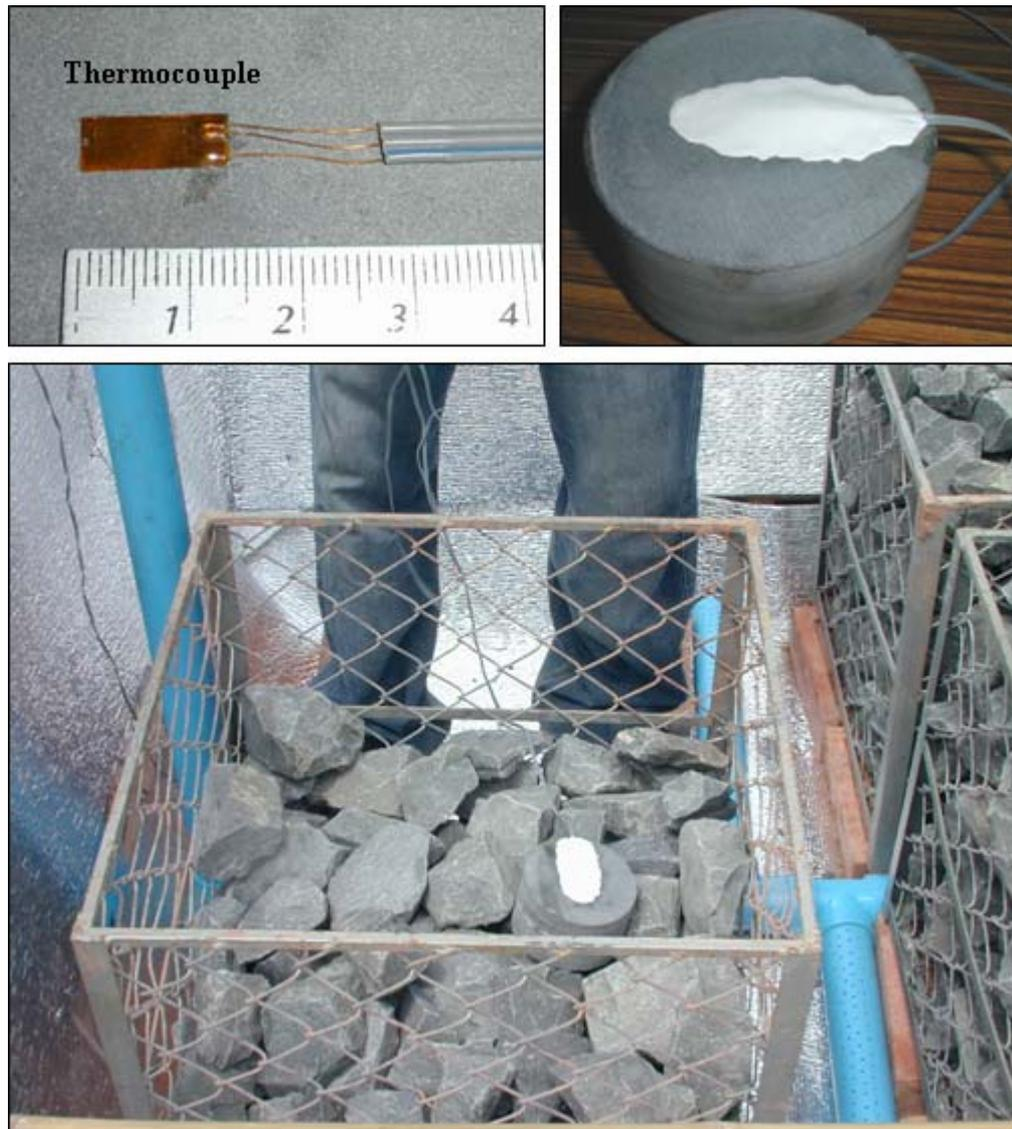
**Figure 5.4** Thermocouple (the upper left) is installed onto the polished surface of rock sample using protective glue (the upper right) and placed into the middle of chain-link basket to measure the temperature of rock fragments (bottom).
