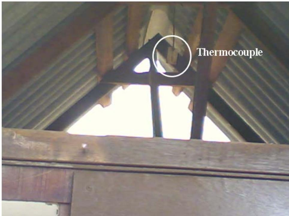
**Figure 5.8** Thermocouple was hung under the roof to monitor the surrounding air temperature.
