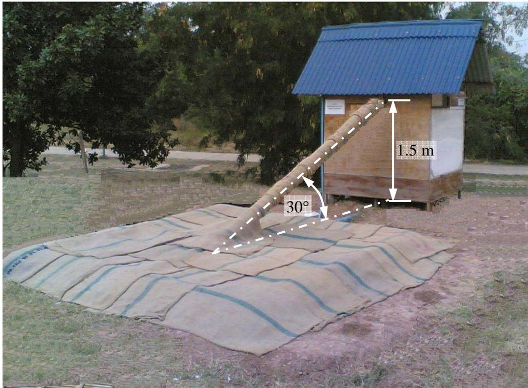
**Figure 5.11** The storage pit (front) was connected to the housing model (back) with 10.2-cm diameter hot-air tube. The tube was inclined at an angle of 30 degrees with the vertical height of 1.5 m.
