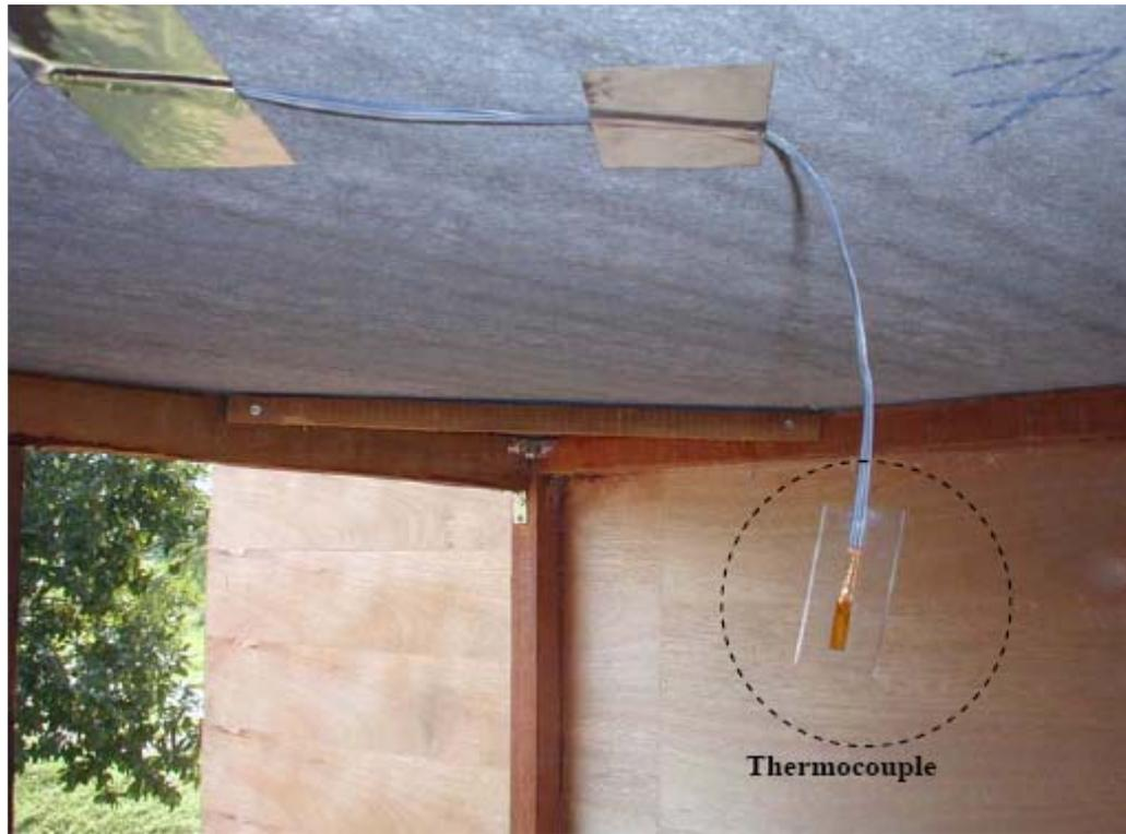
**Figure 5.7** Thermocouple was hung in the housing model to monitor its temperature.
