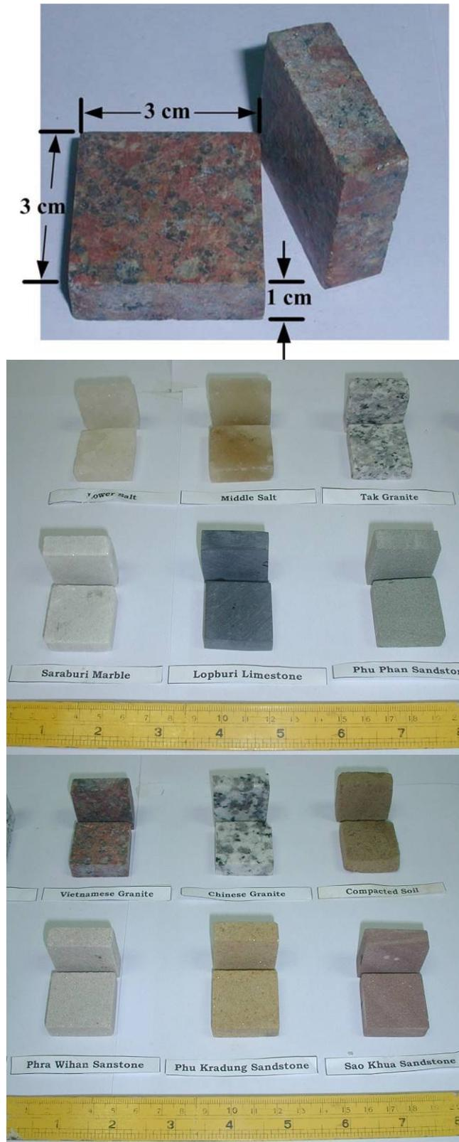
**Figure 3.3** Rock and soil specimens prepared for the thermal property determination.
