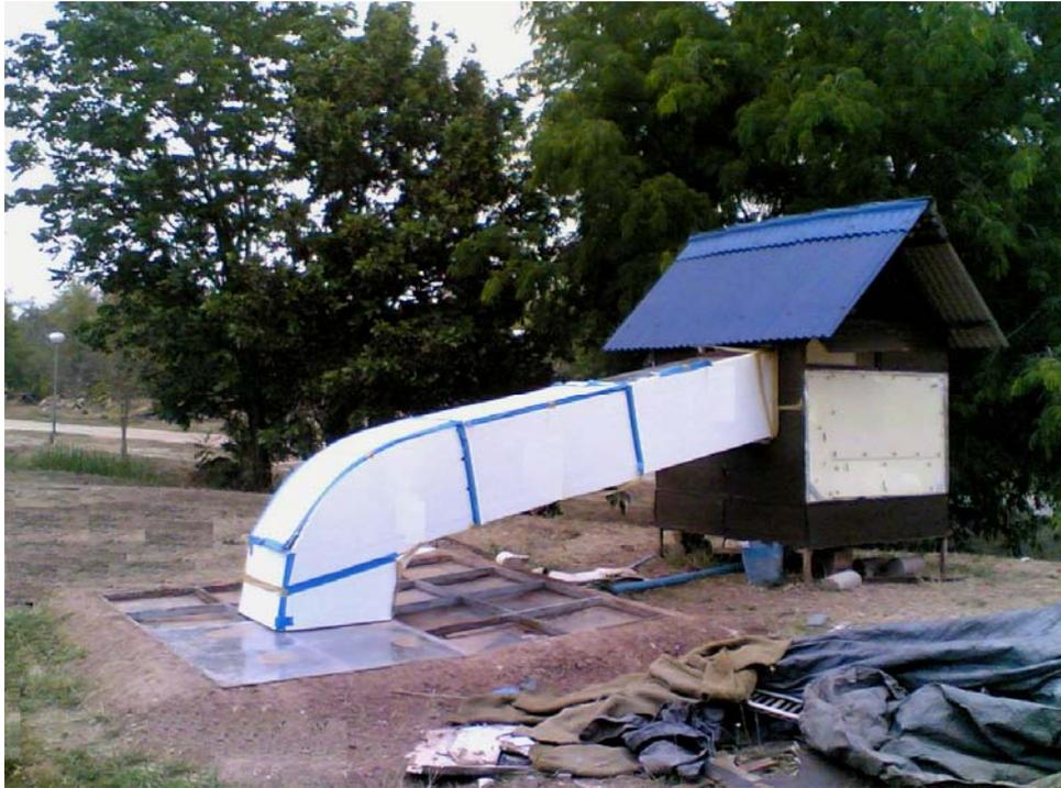
**Figure 5.15** The storage pit (left) connected to the housing model (right) by a  $0.6 \times 0.6$  m cross-sectional area vent. The vent made from zinc sheet and covered by 2-cm thick foam sheet.
