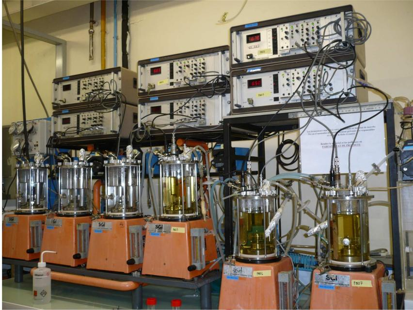
**Figure 3.1** Bioreactor apparatus for uncontrolled oxygen interaction experiments
