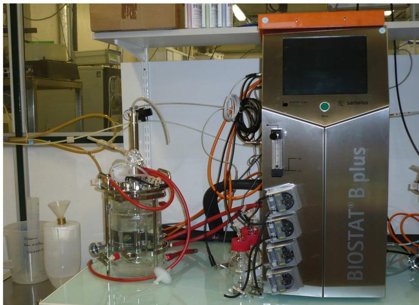
**Figure 3.2** Bioreactor apparatus for 80 % oxygen interaction experiments
