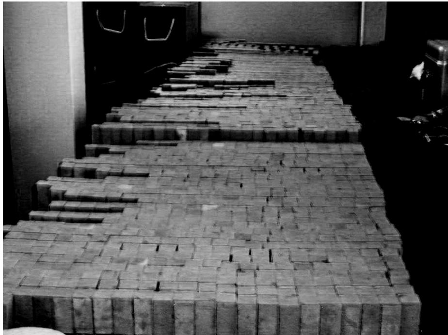
**Figure 4.1.** Nearly 1000 blocks of Phu Phan sandstone prepared for testing.
