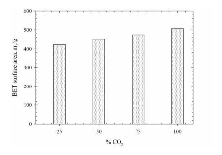
**Figure 3.51** Effect of CO<sub>2</sub> concentration on BET surface area of the palm fiber based activated carbon activated at 850°C for 2.0 hrs.
