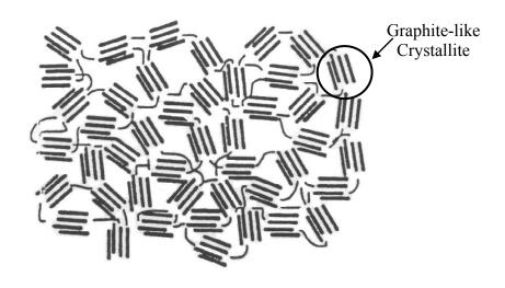
Figure 4.2 Schematic diagram of char structure.
