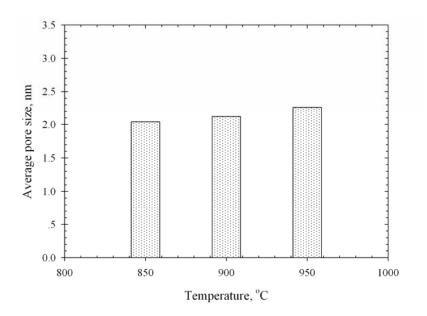
Figure 3.21 Effect of activation temperature on average pore size of the palm shell based activated carbon activated with pure  $CO_2$  for 2.0 hrs.
