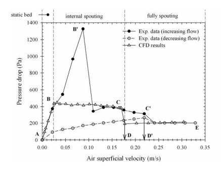
**Figure 5.48** The experimental and CFD simulated results of pressure drop-air flow rate diagram.
