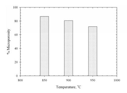
**Figure 3.23** Effect of activation temperature on percentage microporosity of the palm shell based activated carbon activated with pure CO<sub>2</sub> for 2.0 hrs.
