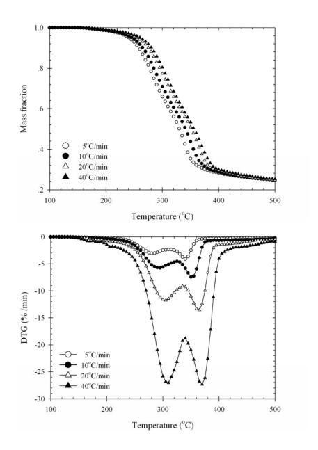
Figure 2.6 TG and DTG data of palm fiber pyrolyzed at different heating rate.
