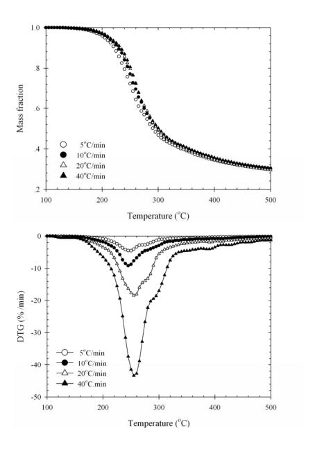
**Figure 2.7** TG and DTG data of palm kernel cake cake pyrolyzed at different heating rates.
