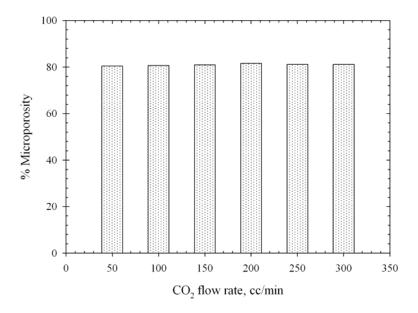
**Figure 3.28** Effect of CO<sub>2</sub> flow rate on percentage microporosity of the palm shell based activated carbon activated at 900°C with pure CO<sub>2</sub> for 2.0 hrs.
