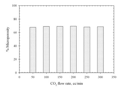
Figure 3.48 Effect of  $CO_2$  flow rate on percentage microporosity of the palm fiber based activated carbon activated at  $850^{\circ}$ C with pure  $CO_2$  for 2.0 hrs.
