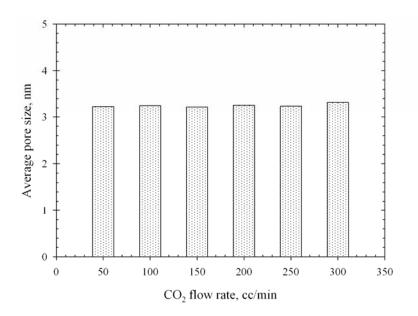
**Figure 3.68** Effect of  $CO_2$  flow rate on average pore size of the palm kernel cake based activated carbon activated at  $900^{\circ}$ C with pure  $CO_2$  for 2.0 hrs.
