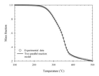
Figure 2.19 TG data and model fitting for bagasse pyrolyzed at 10°C/min.
