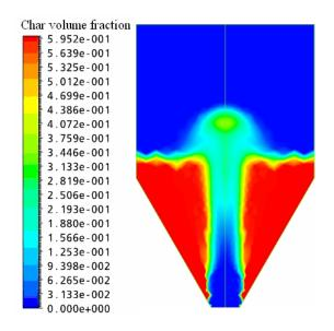
**Figure 5.68** Steady-state concentration profile of palm-shell char at t = 0 in the spouted bed activator
