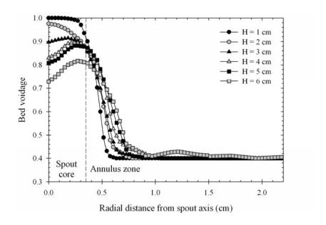
**Figure 5.53** Bed voidage profiles of palm-shell char particles at air velocity of  $1.143 U_{MS}$ .
