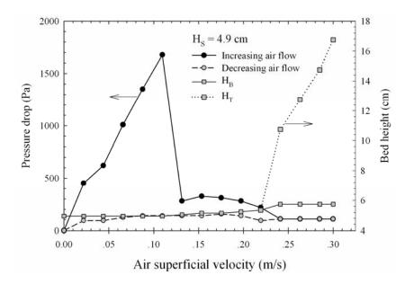
**Figure 5.26** Pressure drop–flow rate diagram and bed height of spouted bed for  $D_I = 5.0$  mm,  $d_P = 0.7$  mm,  $\theta = 45^{\circ}$  and  $H_S = 4.9$  cm.
