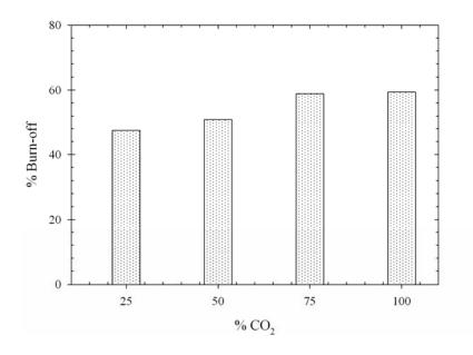
Figure 3.70 Effect of  $CO_2$  concentration on char burn-off of the palm kernel cake based activated carbon activated at  $900^{\circ}C$  for 2.0 hrs.
