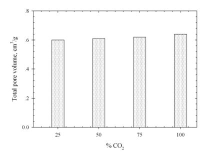
**Figure 3.72** Effect of CO<sub>2</sub> concentration on total pore volume of the palm kernel cake based activated carbon activated at 900°C for 2.0 hrs.
