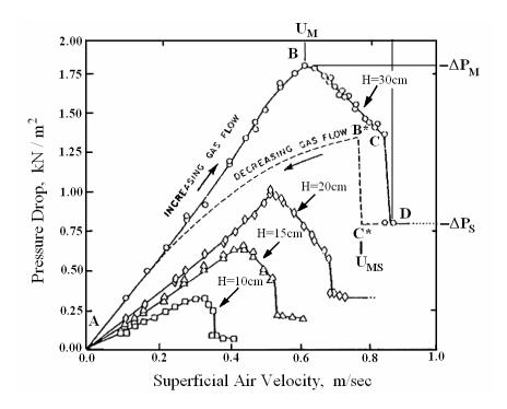
**Figure 5.2** Typical pressure drop-flow rate curves of conventional spouted bed (Mathur and Epstein, 1974).
