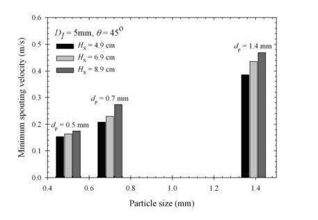
Figure 5.32 Effect of particle size on minimum spouting velocity.
