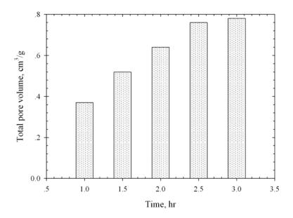
Figure 3.62 Effect of activation time on total pore volume of the palm kernel cake based activated carbon activated at  $900^{\circ}$ C with pure  $CO_2$ .
