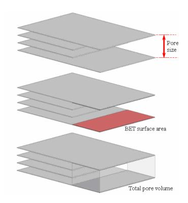
**Figure 4.4** Schematic representation of pore size, surface area, and total pore volume of graphite crystallite at any char burn-offs.
