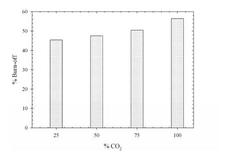
**Figure 3.50** Effect of CO<sub>2</sub> concentration on char burn-off of the palm shell based activated carbon activated at 850°C for 2.0 hrs.
