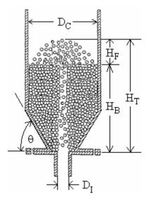
**Figure 5.3** Geometric dimensions of a spouted bed column.
