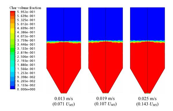
**Figure 5.49** Char particle concentration distribution at several air velocities.
