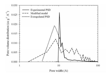
**Figure 4.19** Experimental, computed and extrapolated pore size distributions and of palm fiber based activated carbons at 56.5% burn-off.
