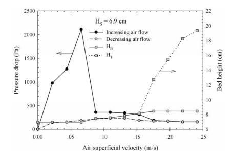
**Figure 5.24** Pressure drop–flow rate diagram and bed height of spouted bed for  $D_I = 5.0 \text{ mm}$ ,  $d_P = 0.5 \text{ mm}$ ,  $\theta = 45^{\circ}$  and  $H_S = 6.9 \text{ cm}$ .
