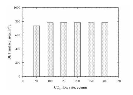
**Figure 3.66** Effect of CO<sub>2</sub> flow rate on BET surface area of the palm kernel cake based activated carbon activated at 900°C with pure CO<sub>2</sub> for 2.0 hrs.
