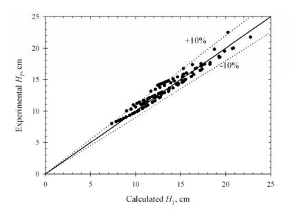
**Figure 5.40** Comparison of experimental and calculated total bed height by Equation (5.54).
