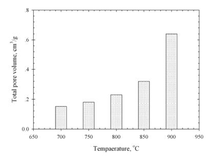
Figure 3.57 Effect of activation temperature on total pore volume of the palm kernel cake based activated carbon activated with pure  $CO_2$  for 2.0 hrs.
