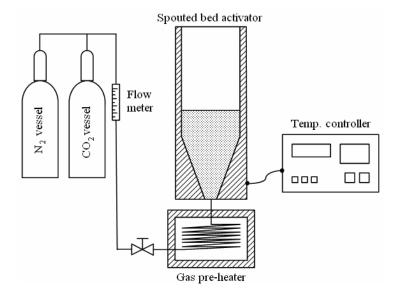
**Figure 5.5** Schematic diagram of spouted bed activator.
