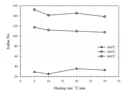
**Figure 3.6** Effect of heating rate on the final yield and iodine number of the palm shell chars for particle size of 1.4 mm carbonized at 1.0 hr of holding time.
