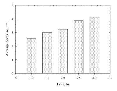
Figure 3.63 Effect of activation time on average pore size of the palm kernel cake based activated carbon activated at  $900^{\circ}$ C with pure  $CO_2$ .
