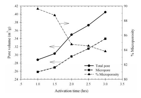
**Figure 5.43** Effect of activation time on total and micropore volume, and percentage microporosity of activated carbons prepared at 900°C in the batch spouted bed activator.
