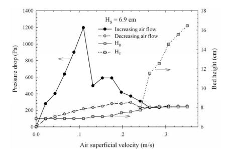
**Figure 5.14** Pressure drop–flow rate diagram and bed height of spouted bed for  $D_I = 7.0 \text{ mm}, d_P = 0.5 \text{ mm}, \theta = 45^{\circ} \text{ and } H_S = 6.9 \text{ cm}.$
