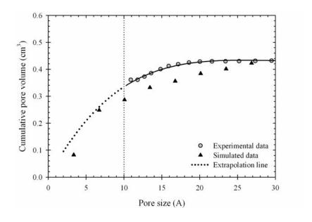
**Figure 4.14** Extrapolation of cumulative pore volume at small pore size for calculation of PSD of palm shell based activated carbons.
