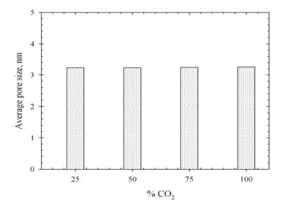
**Figure 3.73** Effect of CO<sub>2</sub> concentration on average pore size of the palm kernel cake based activated carbon activated at 900°C for 2.0 hrs.
