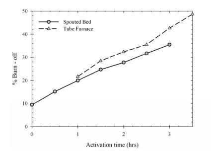
**Figure 5.41** Effect of activation time on the extent of char burn-off during activation with  $CO_2$  at  $900^{\circ}C$ .
