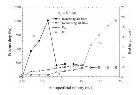
**Figure 5.21** Pressure drop—flow rate diagram and bed height of spouted bed for  $D_I = 5.0 \text{ mm}, d_P = 0.5 \text{ mm}, \theta = 60^{\circ} \text{ and } H_S = 8.3 \text{ cm}.$
