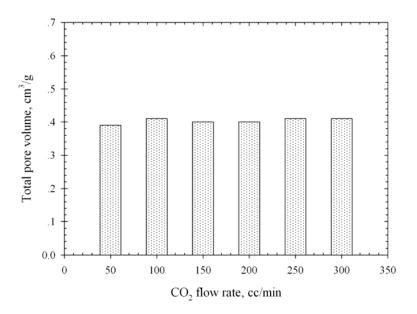
Figure 3.27 Effect of  $CO_2$  flow rate on total pore volume of the palm shell based activated carbon activated at  $900^{\circ}$ C with pure  $CO_2$  for 2.0 hrs.
