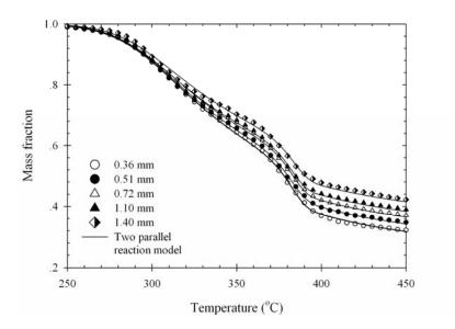
**Figure 2.14** TG data and two-parallel reaction model fitting for palm shell pyrolyzed at heating rate of 20°C /min for different particle sizes.
