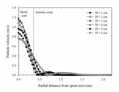
Figure 5.52 Velocity profiles of palm-shell particles at air velocity of  $1.143 U_{MS}$ .
