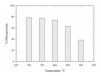
Figure 3.59 Effect of activation temperature on percentage microporosity of the palm kernel cake based activated carbon activated with pure  $CO_2$  for 2.0 hrs.
