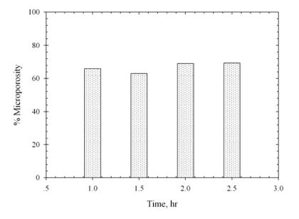
Figure 3.44 Effect of activation time on percentage microporosity of the palm fiber based activated carbon activated at  $850^{\circ}$ C with pure  $CO_2$ .
