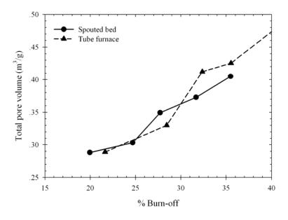
Figure 5.45 Effect of char burn-off on total pore volume.
