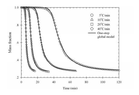
Figure 2.10 TG data and one-step global model fitting of palm kernel cake.
