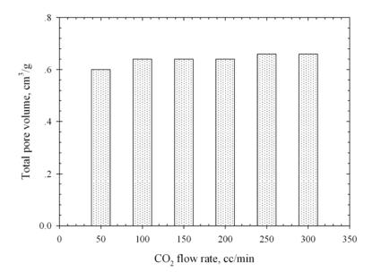
**Figure 3.67** Effect of  $CO_2$  flow rate on total pore volume of the palm kernel cake based activated carbon activated at  $900^{\circ}$ C with pure  $CO_2$  for 2.0 hrs.
