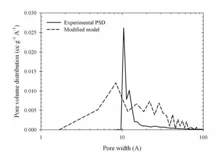
**Figure 4.18** Experimental and computed pore size distributions of oil-palm fiber based activated carbons at 56.5% burn-off.
