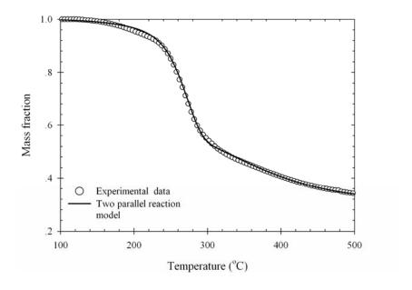
Figure 2.20 TG data and model fitting for longan seed pyrolyzed at 10°C/min.
