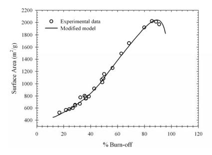
**Figure 4.11** Experimental data and simulated results of surface area of palm shell based activated carbons.
