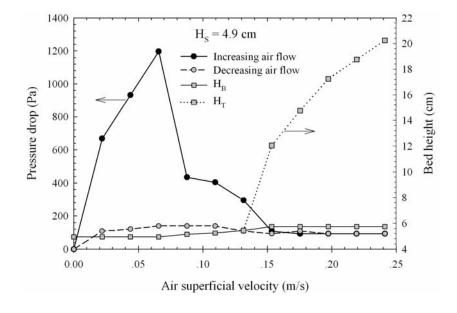
**Figure 5.23** Pressure drop–flow rate diagram and bed height of spouted bed for  $D_I = 5.0 \text{ mm}$ ,  $d_P = 0.5 \text{ mm}$ ,  $\theta = 45^{\circ}$  and  $H_S = 4.9 \text{ cm}$ .
