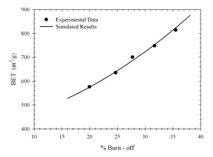
**Figure 5.71** Experimental and simulated BET surface area of activated carbons prepared from palm shell in spouted bed activator.
