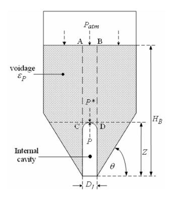
Figure 5.37 Configuration of a turbulent free-jet in spouted bed.
