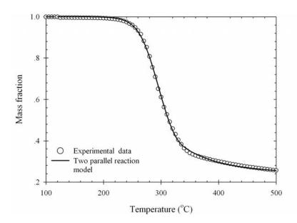
**Figure 2.21** TG data and model fitting for cassava waste residue pyrolyzed at 10°C/min.
