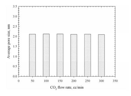
**Figure 3.29** Effect of  $CO_2$  flow rate on average pore size of the palm shell based activated carbon activated at  $900^{\circ}$ C with pure  $CO_2$  for 2.0 hrs.
