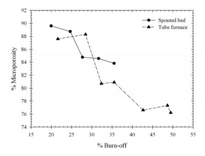
Figure 5.46 Effect of char burn-off on percentage microporosity.
