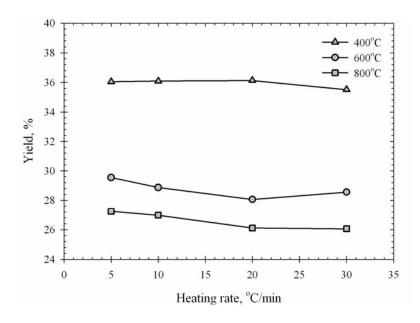
**Figure 3.14** Effect of heating rate on the final yield of the palm kernel cake chars carbonized at 1.0 hr of holding time.
