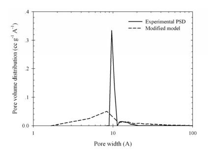
**Figure 4.13** Experimental and computed pore size distributions of palm shell based activated carbons at 48.5% burn-off.
