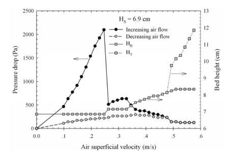
**Figure 5.18** Pressure drop–flow rate diagram and bed height of spouted bed for  $D_I = 7.0 \text{ mm}$ ,  $d_P = 1.4 \text{ mm}$ ,  $\theta = 45^{\circ}$  and  $H_S = 6.9 \text{ cm}$ .
