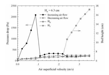
**Figure 5.22** Pressure drop–flow rate diagram and bed height of spouted bed for  $D_I = 5.0 \text{ mm}, d_P = 0.7 \text{ mm}, \theta = 60^{\circ} \text{ and } H_S = 6.3 \text{ cm}.$
