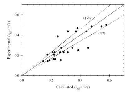
**Figure 5.38** Comparison of experimental and calculated minimum spouting velocities by Equation (5.51).
