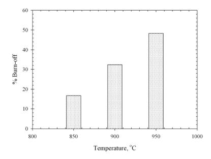
Figure 3.15 Effect of activation temperature on char burn-off of the palm shell based activated carbon activated with pure  $CO_2$  for 2.0 hrs.
