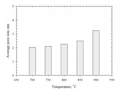
Figure 3.58 Effect of activation temperature on average pore size of the palm kernel cake based activated carbon activated with pure  $CO_2$  for 2.0 hrs.
