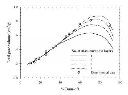
**Figure 4.7** Experimental data and simulated results of total pore volume for various maximum number of burnt out layers of longan seed based activated carbons.
