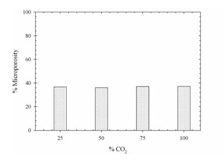
**Figure 3.74** Effect of CO<sub>2</sub> concentration on percentage microporosity of the palm kernel cake based activated carbon activated at 900°C for 2.0 hrs.
