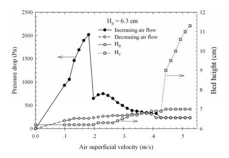
**Figure 5.11** Pressure drop–flow rate diagram and bed height of spouted bed for  $D_I = 7.0 \text{ mm}$ ,  $d_P = 1.4 \text{ mm}$ ,  $\theta = 60^{\circ}$  and  $H_S = 6.3 \text{ cm}$ .
