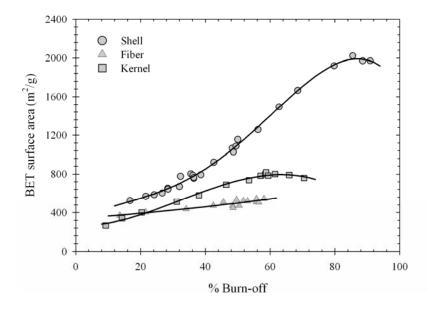
Figure 3.75 Effect of char burn-off on BET surface area.
