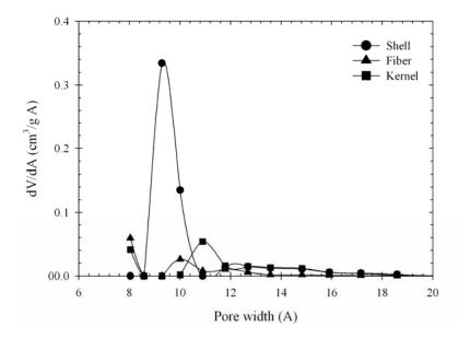
**Figure 3.78** Pore size distribution of activated carbons prepared at optimum conditions, determined by DFT model (El-Merraoui et al., 2000).
