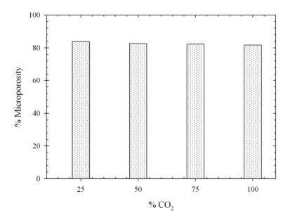
**Figure 3.33** Effect of CO<sub>2</sub> concentration on percentage microporosity of the palm shell based activated carbon activated at 900°C for 2.0 hrs.
