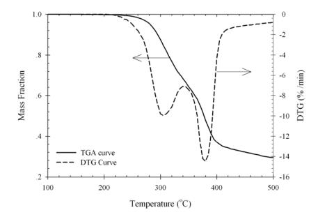
Figure 2.1 TG and DTG data of palm shell pyrolyzed at heating rate of 20°C/min.
