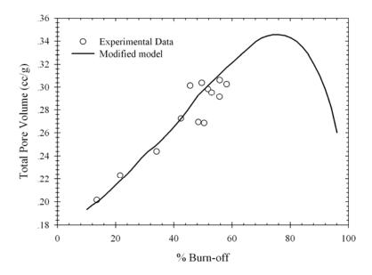
**Figure 4.17** Experimental data and simulated results of total pore volume of oil-palm fiber based activated carbons.
