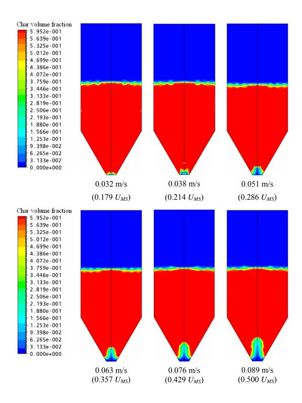
Figure 5.49 Char particle concentration distribution at several air velocities (Cont.).
