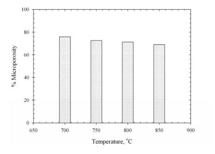
Figure 3.38 Effect of activation temperature on percentage microporosity of the palm fiber based activated carbon activated with pure  $CO_2$  for 2.0 hrs.
