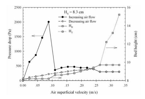
**Figure 5.9** Pressure drop–flow rate diagram and bed height of spouted bed for  $D_I = 7.0 \text{ mm}$ ,  $d_P$  of 0.7 mm,  $\theta = 60^{\circ}$  and  $H_S = 8.3 \text{ cm}$ .
