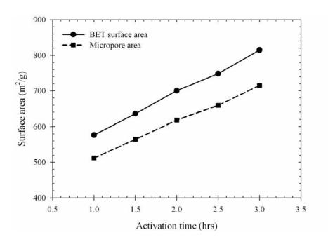
**Figure 5.42** Effect of activation time on BET and micropore area of activated carbons prepared at 900°C in the batch spouted bed activator.
