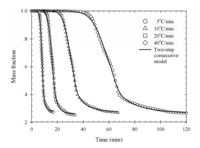
Figure 2.11 TG data and two-step consecutive model fitting of palm shell.
