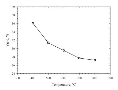
**Figure 3.12** Effect of carbonization temperature on the final yield of the palm kernel cake chars carbonized at heating rate of 5°C/min and 1.0 hr of holding time.
