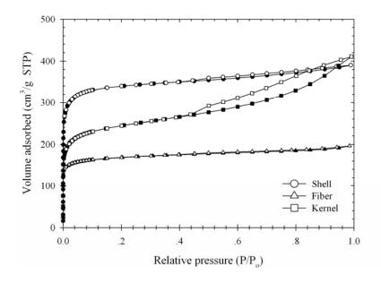
**Figure 3.77** N<sub>2</sub> adsorption isotherm at -196°C of activated carbons prepared at optimum conditions.
