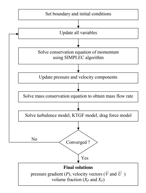
Figure 5.4 Flow sheet of the CFD simulation algorithm.
