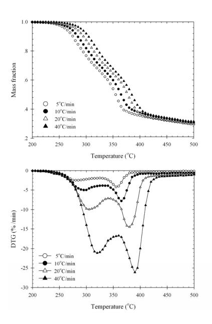
**Figure 2.5** TG and DTG data of palm shell pyrolyzed at particle size 0.36 mm for various heating rate.
