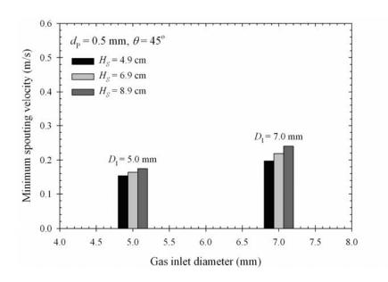
**Figure 5.34** Effect of gas inlet diameters on minimum spouting velocity for particle size of 0.5 mm and conical base angle 45°.
