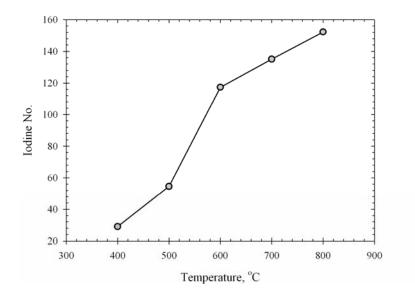
**Figure 3.2** Effect of carbonization temperature on the iodine number of the palm shell chars for particle size of 1.4 mm carbonized at heating rate of 5°C/min and 1.0 hr of holding time.
