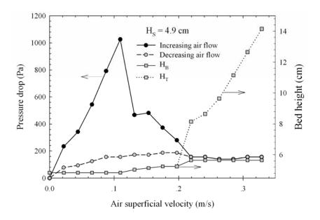
**Figure 5.13** Pressure drop–flow rate diagram and bed height of spouted bed for  $D_I = 7.0 \text{ mm}$ ,  $d_P = 0.5 \text{ mm}$ ,  $\theta = 45^{\circ}$  and  $H_S = 4.9 \text{ cm}$ .
