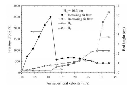
**Figure 5.10** Pressure drop—flow rate diagram and bed height of spouted bed for  $D_I = 7.0 \text{ mm}$ ,  $d_P$  of 0.7 mm,  $\theta = 60^\circ$  and  $H_S = 10.3 \text{ cm}$ .
