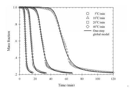
Figure 2.9 TG data and one-step global model fitting of palm fiber.
