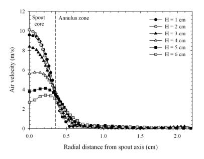
**Figure 5.51** Velocity profiles of air at air velocity of  $1.143U_{MS}$ .
