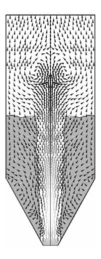
**Figure 5.67** Circulation pattern of air at air velocity of  $1.143U_{MS}$
