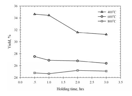
**Figure 3.10** Effect of holding time on the final yield of the palm fiber chars carbonized at 1.0 hr of holding time.
