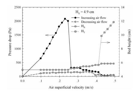
**Figure 5.29** Pressure drop–flow rate diagram and bed height of spouted bed for  $D_I = 5.0 \text{ mm}, d_P = 1.4 \text{ mm}, \theta = 45^{\circ} \text{ and } H_B = 4.9 \text{ cm}.$
