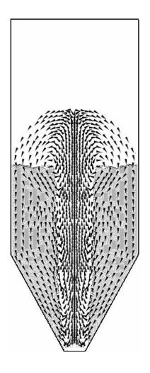
Figure 5.66 Circulation pattern of char particles at air velocity of  $1.143 U_{MS}$
