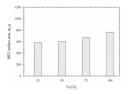
**Figure 3.31** Effect of CO<sub>2</sub> concentration on BET surface area of the palm shell based activated carbon activated at 900°C for 2.0 hrs.
