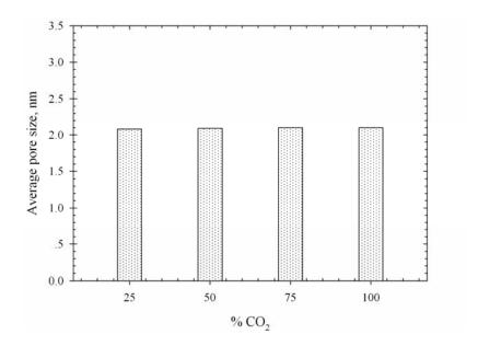
**Figure 3.34** Effect of CO<sub>2</sub> concentration on average pore size of the palm shell based activated carbon activated at 900°C for 2.0 hrs.
