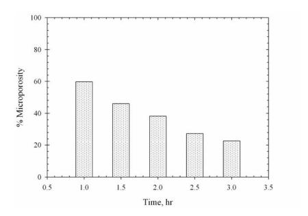
**Figure 3.64** Effect of activation time on percentage microporosity of the palm kernel cake based activated carbon activated at 900°C with pure CO<sub>2</sub>.
