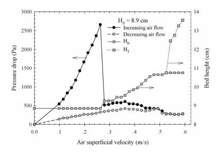
**Figure 5.19** Pressure drop–flow rate diagram and bed height of spouted bed for  $D_I = 7.0 \text{ mm}$ ,  $d_P = 1.4 \text{ mm}$ ,  $\theta = 45^{\circ}$  and  $H_S = 8.9 \text{ cm}$ .
