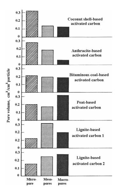
**Figure 1.1** Pore size distribution in some activated carbons obtained using different precursors (Bansal et al, 1988).
