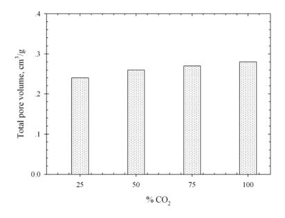
**Figure 3.52** Effect of CO<sub>2</sub> concentration on total pore volume of the palm fiber based activated carbon activated at 850°C for 2.0 hrs.
