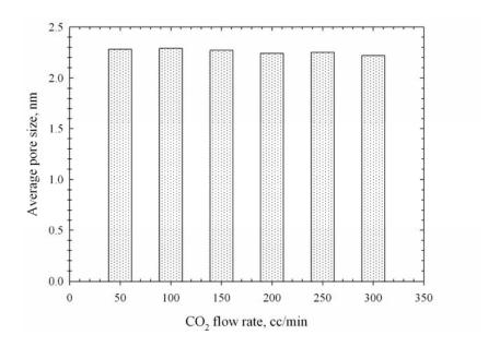
**Figure 3.49** Effect of  $CO_2$  flow rate on average pore size of the palm fiber based activated carbon activated at  $850^{\circ}$ C with pure  $CO_2$  for 2.0 hrs.
