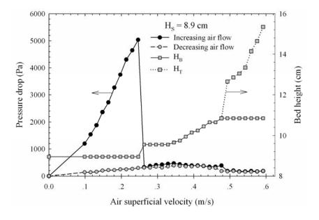
**Figure 5.31** Pressure drop–flow rate diagram and bed height of spouted bed for  $D_I = 5.0$  mm,  $d_P = 1.4$  mm,  $\theta = 45^{\circ}$  and  $H_B = 8.9$  cm.
