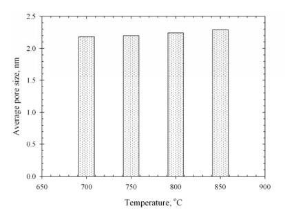
Figure 3.39 Effect of activation temperature on average pore size of the palm fiber based activated carbon activated with pure  $CO_2$  for 2.0 hrs.
