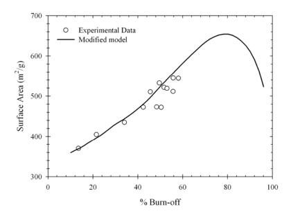
**Figure 4.16** Experimental data and simulated results of surface area of oil-palm fiber based activated carbons.
