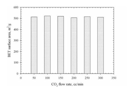
Figure 3.46 Effect of  $CO_2$  flow rate on BET surface area of the palm fiber based activated carbon activated at  $850^{\circ}$ C with pure  $CO_2$  for 2.0 hrs.
