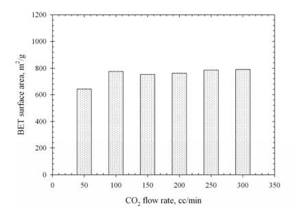
**Figure 3.26** Effect of CO<sub>2</sub> flow rate on BET surface area of the palm shell based activated carbon activated at 900°C with pure CO<sub>2</sub> for 2.0 hrs.
