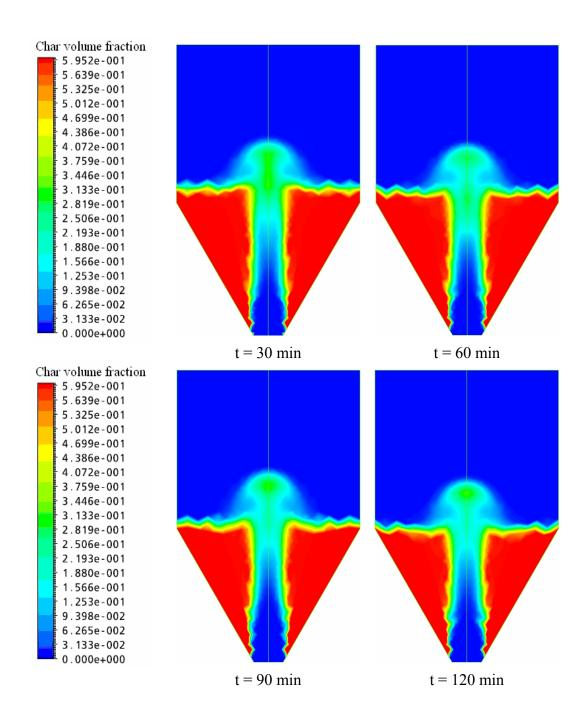
**Figure 5.70** Concentration profiles of palm-shell char at different activation times in the spouted bed activator
