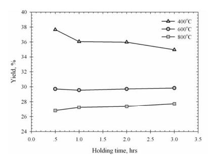
**Figure 3.13** Effect of holding time on the final yield of the palm kernel cake chars carbonized at 5°C/min of heating rate.
