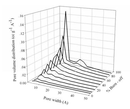
**Figure 4.10** The simulated pore size distributions of longan seed based activated carbons at various degrees of char burn-off.
