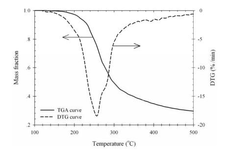
**Figure 2.3** TG and DTG data of palm kernel cake pyrolyzed at heating rate of 20°C/min.
