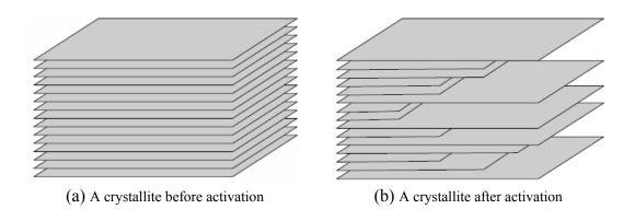
Figure 4.3 Schematic diagram of a crystallite structure.
