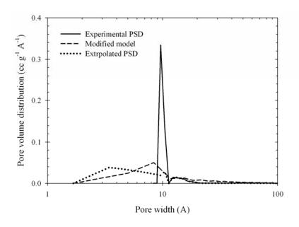
**Figure 4.15** Experimental, computed and extrapolated pore size distributions and of palm shell based activated carbons at 48.5% burn-off.
