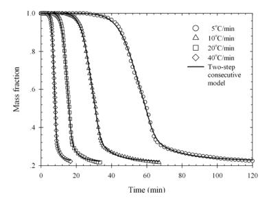
Figure 2.12 TG data and two-step consecutive model fitting of palm fiber.
