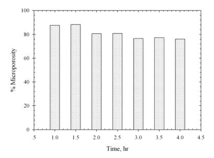
**Figure 3.24** Effect of activation time on percentage microporosity of the palm shell based activated carbon activated at 900°C.
