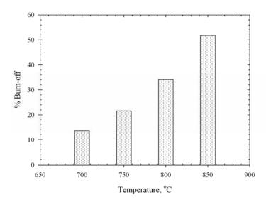
Figure 3.35 Effect of activation temperature on char burn-off of the palm fiber based activated carbon activated with pure  $CO_2$  for 2.0 hrs.
