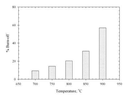
**Figure 3.55** Effect of activation temperature on char burn-off of the palm kernel cake based activated carbon activated with pure CO<sub>2</sub> for 2.0 hrs.
