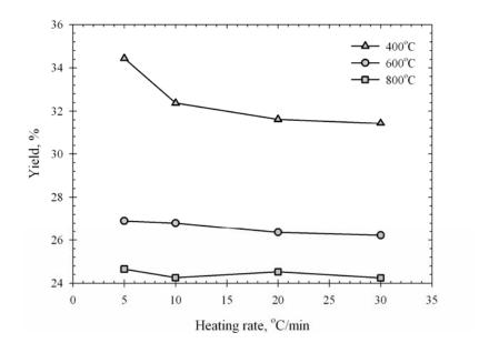
**Figure 3.11** Effect of heating rate on the final yield of the palm fiber chars carbonized at 5°C/min of heating rate.
