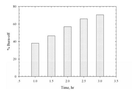
**Figure 3.60** Effect of activation time on char burn-off of the palm kernel cake based activated carbon activated at  $900^{\circ}$ C with pure  $CO_2$ .
