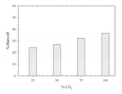
**Figure 3.30** Effect of CO<sub>2</sub> concentration on char burn-off of the palm shell based activated carbon activated at 900°C for 2.0 hrs.
