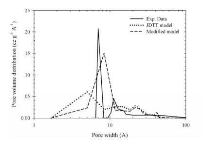
**Figure 4.9** Experimental and computed pore size distributions of longan seed based activated carbons at 90.1% burn-off.
