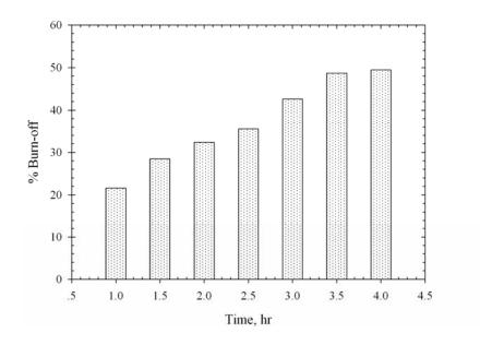
**Figure 3.18** Effect of activation time on char burn-off of the palm shell based activated carbon activated at 900°C.
