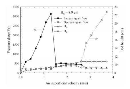
**Figure 5.28** Pressure drop–flow rate diagram and bed height of spouted bed for  $D_I = 5.0 \text{ mm}$ ,  $d_P = 0.7 \text{ mm}$ ,  $\theta = 45^{\circ}$  and  $H_S = 8.9 \text{ cm}$ .
