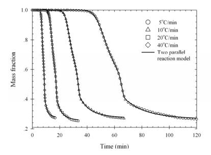
**Figure 2.15** TG data and two-parallel reaction model fitting for palm shell pyrolyzed for particle sizes of 0.36 mm at different heating rates.
