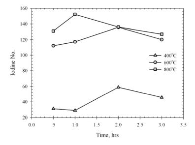
**Figure 3.8** Effect of holding time on the final yield and iodine number of the palm shell chars for particle size of 1.4 mm carbonized at heating rate of 5°C/min.
