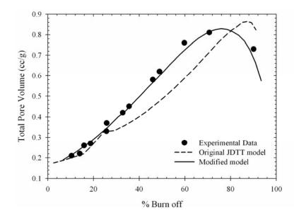
**Figure 4.6** Experimental data and simulated results of total pore volume of longan seed based activated carbons.
