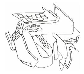
Figure 1.2 Schematic representation of activated carbon structure.
