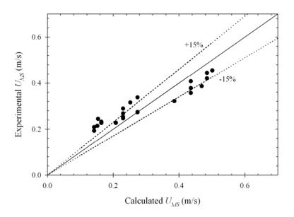
**Figure 5.39** Comparison of experimental and calculated minimum spouting velocities by Equation (5.53).
