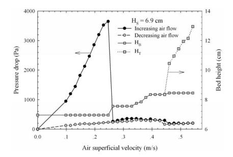
**Figure 5.30** Pressure drop–flow rate diagram and bed height of spouted bed for  $D_I = 5.0 \text{ mm}$ ,  $d_P = 1.4 \text{ mm}$ ,  $\theta = 45^{\circ}$  and  $H_B = 6.9 \text{ cm}$ .
