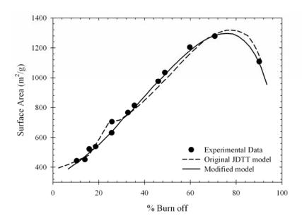
**Figure 4.5** Experimental data and simulated results of surface area of longan seed based activated carbons.
