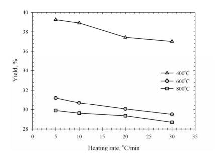
**Figure 3.5** Effect of heating rate on the final yield of the palm shell chars for particle size of 1.4 mm carbonized at 1.0 hr of holding time.
