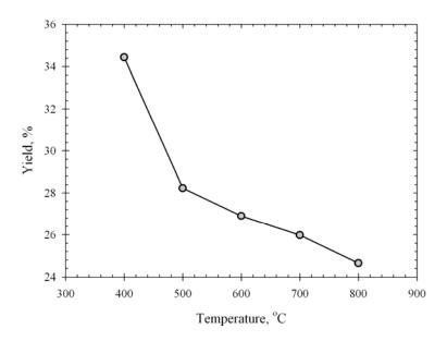
**Figure 3.9** Effect of carbonization temperature on the final yield of the palm fiber chars carbonized at heating rate of 5°C/min and 1.0 hr of holding time.
