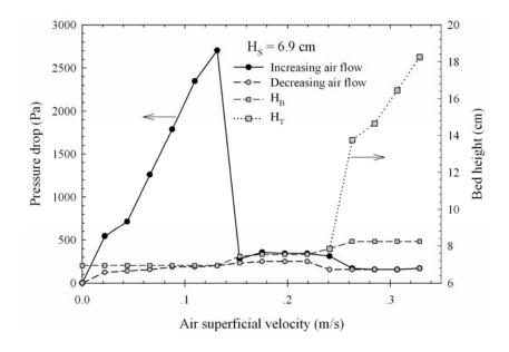
**Figure 5.27** Pressure drop–flow rate diagram and bed height of spouted bed for  $D_I = 5.0 \text{ mm}$ ,  $d_P = 0.7 \text{ mm}$ ,  $\theta = 45^{\circ}$  and  $H_S = 6.9 \text{ cm}$ .
