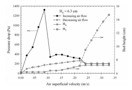
**Figure 5.8** Pressure drop–flow rate diagram and bed height of spouted bed for  $D_I = 7.0 \text{ mm}$ ,  $d_P$  of 0.7 mm,  $\theta = 60^{\circ}$  and  $H_S = 6.3 \text{ cm}$ .
