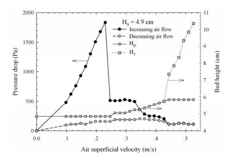
**Figure 5.17** Pressure drop–flow rate diagram and bed height of spouted bed for  $D_I = 7.0 \text{ mm}$ ,  $d_P = 1.4 \text{ mm}$ ,  $\theta = 45^{\circ}$  and  $H_S = 4.9 \text{ cm}$ .
