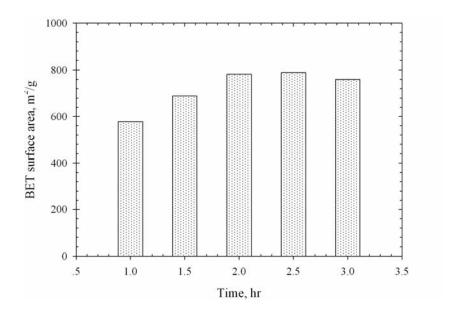
**Figure 3.61** Effect of activation time on BET surface area of the palm kernel cake based activated carbon activated at 900°C with pure CO<sub>2</sub>.
