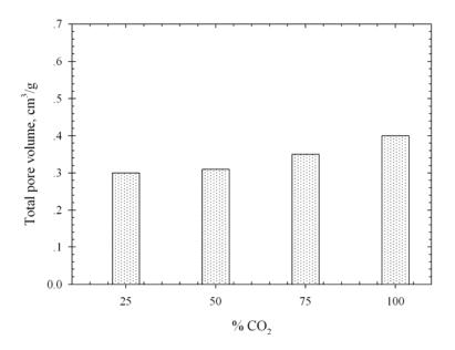
**Figure 3.32** Effect of CO<sub>2</sub> concentration on total pore volume of the palm shell based activated carbon activated at 900°C for 2.0 hrs.
