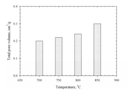
**Figure 3.37** Effect of activation temperature on total pore volume of the palm fiber based activated carbon activated with pure CO<sub>2</sub> for 2.0 hrs.
