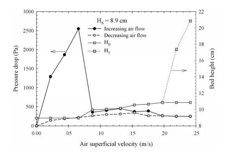
**Figure 5.25** Pressure drop–flow rate diagram and bed height of spouted bed for  $D_I = 5.0 \text{ mm}$ ,  $d_P = 0.5 \text{ mm}$ ,  $\theta = 45^{\circ}$  and  $H_S = 8.9 \text{ cm}$ .
