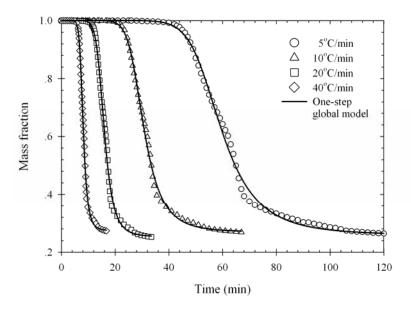
Figure 2.8 TG data and one-step global model fitting of palm shell.
