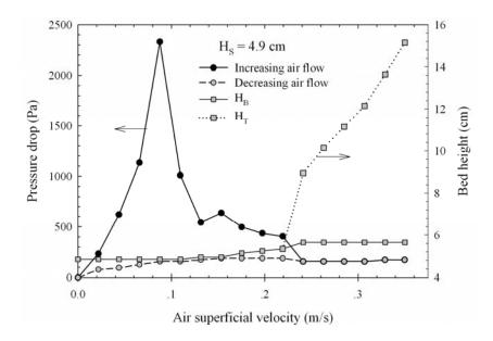
**Figure 5.16** Pressure drop–flow rate diagram and bed height of spouted bed for  $D_I = 7.0 \text{ mm}, d_P = 0.7 \text{ mm}, \theta = 45^{\circ} \text{ and } H_S = 4.9 \text{ cm}.$
