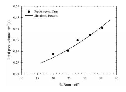
**Figure 5.72** Experimental and simulated total pore volume of activated carbons prepared from palm shell in spouted bed activator.
