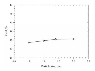
**Figure 3.3** Effect of particle size on the final yield and iodine number of the palm shell chars carbonized at 600°C, 5°C/min of heating rate, and 1.0 hr of holding time.
