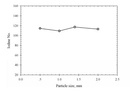
**Figure 3.4** Effect of particle size on the final yield and iodine number of the palm shell chars carbonized at 600°C, 5°C/min of heating rate, and 1.0 hr of holding time.
