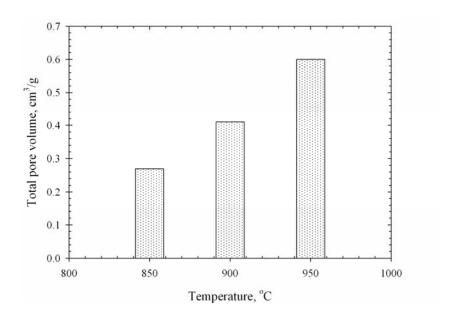
Figure 3.17 Effect of activation temperature on total pore volume of the palm shell based activated carbon activated with pure  $CO_2$  for 2.0 hrs.
