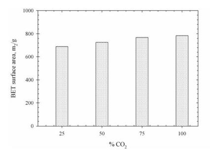
**Figure 3.71** Effect of CO<sub>2</sub> concentration on BET surface area of the palm kernel cake based activated carbon activated at 900°C for 2.0 hrs.
