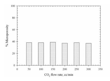
**Figure 3.69** Effect of CO<sub>2</sub> flow rate on percentage microporosity of the palm kernel cake based activated carbon activated at 900°C with pure CO<sub>2</sub> for 2.0 hrs.
