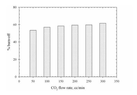
**Figure 3.65** Effect of  $CO_2$  flow rate on char burn-off of the palm kernel cake based activated carbon activated at  $850^{\circ}$ C with pure  $CO_2$  for 2.0 hrs.
