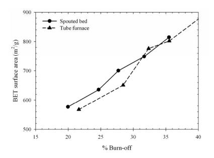
Figure 5.44 Effect Effect of char burn-off on BET surface area.
