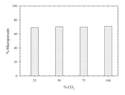
**Figure 3.54** Effect of CO<sub>2</sub> concentration on percentage microporosity of the palm fiber based activated carbon activated at 850°C for 2.0 hrs.
