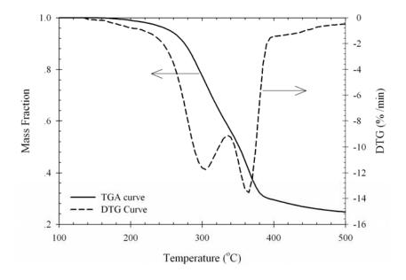
Figure 2.2 TG and DTG data of palm fiber pyrolyzed at heating rate of 20°C/min.
