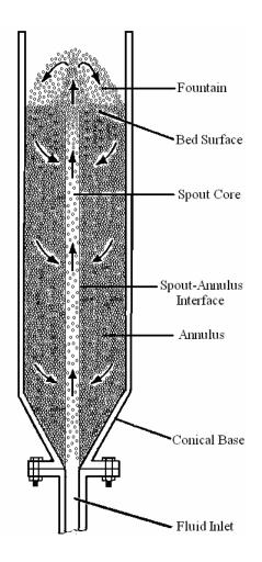
**Figure 5.1** Schematic diagram of a conventional spouted bed (Mathur and Epstein, 1974).
