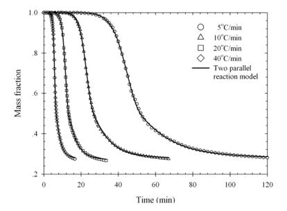
**Figure 2.17** TG data and two-parallel reaction model fitting for palm kernel cake pyrolyzed at different heating rates.
