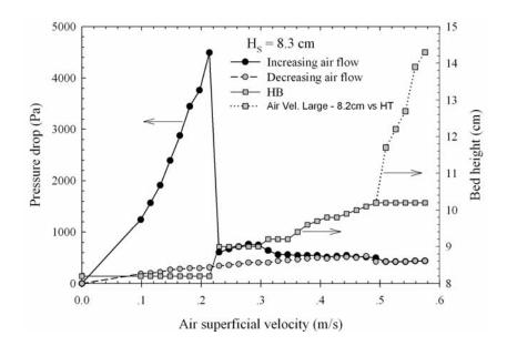
**Figure 5.12** Pressure drop–flow rate diagram and bed height of spouted bed for  $D_I = 7.0 \text{ mm}$ ,  $d_P = 1.4 \text{ mm}$ ,  $\theta = 60^{\circ}$  and  $H_S = 8.3 \text{ cm}$ .
