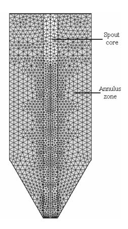
**Figure 5.6** Numerical grids of spouted bed used in CFD simulation.
