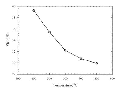
**Figure 3.1** Effect of carbonization temperature on the final yield of the palm shell chars for particle size of 1.4 mm carbonized at heating rate of 5°C/min and 1.0 hr of holding time.
