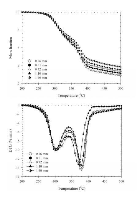
Figure 2.4 TG and DTG data of palm shell pyrolyzed at heating rate of 20°C/min.
