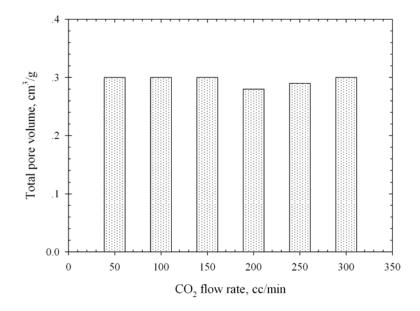
**Figure 3.47** Effect of CO<sub>2</sub> flow rate on total pore volume of the palm fiber based activated carbon activated at 850°C with pure CO<sub>2</sub> for 2.0 hrs.
