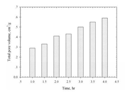
**Figure 3.20** Effect of activation time on total pore volume of the palm shell based activated carbon activated at 900°C.
