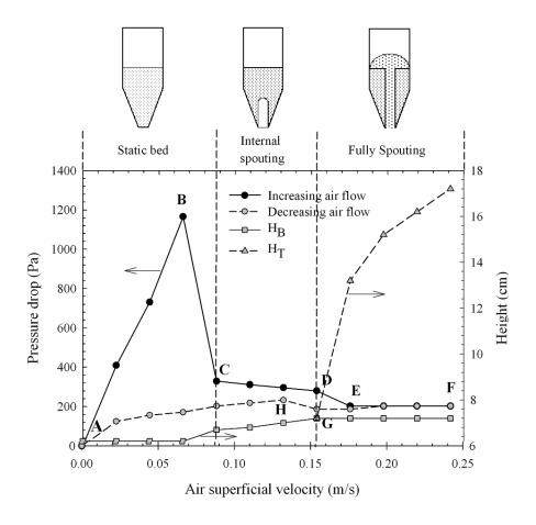
**Figure 5.7** Typical pressure drop–flow rate diagram and bed height for increasing air flow of spouted bed for  $D_I = 7.0$  mm,  $d_P$  of 0.50 mm,  $\theta = 60^{\circ}$  and  $H_S = 6.3$  cm.
