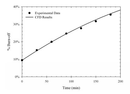
**Figure 5.69** Experimental and CFD simulated char burn-off gasified as a function of activation time in the spouted bed activator
