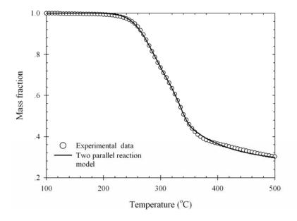
Figure 2.18 TG data and model fitting for coconut shell pyrolyzed at 10°C/min.
