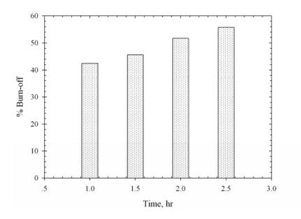
Figure 3.40 Effect of activation time on char burn-off of the palm fiber based activated carbon activated at  $850^{\circ}$ C with pure  $CO_2$ .
