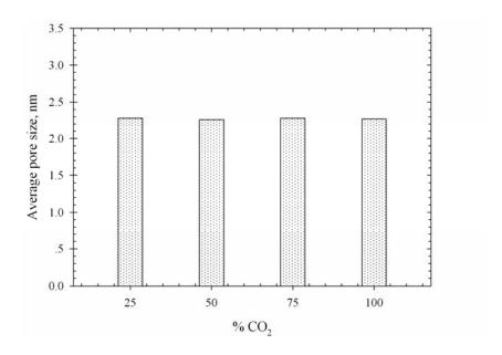
**Figure 3.53** Effect of CO<sub>2</sub> concentration on average pore size of the palm fiber based activated carbon activated at 850°C for 2.0 hrs.
