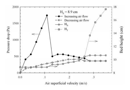
**Figure 5.15** Pressure drop–flow rate diagram and bed height of spouted bed for  $D_I = 7.0 \text{ mm}$ ,  $d_P = 0.5 \text{ mm}$ ,  $\theta = 45^{\circ}$  and  $H_S = 8.9 \text{ cm}$ .
