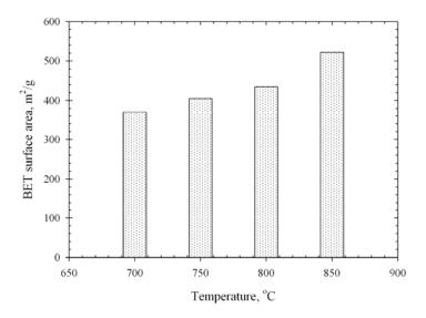
**Figure 3.36** Effect of activation temperature on BET surface area of the palm fiber based activated carbon activated with pure  $CO_2$  for 2.0 hrs.
