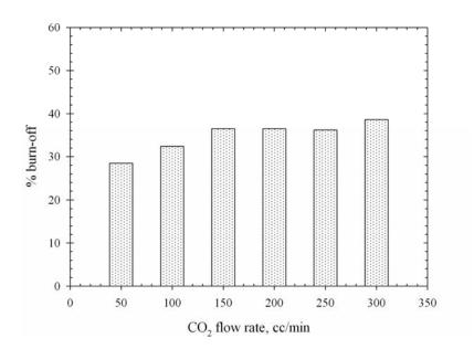
**Figure 3.25** Effect of CO<sub>2</sub> flow rate on char burn-off of the palm shell based activated carbon activated at 900°C with pure CO<sub>2</sub> for 2.0 hrs.
