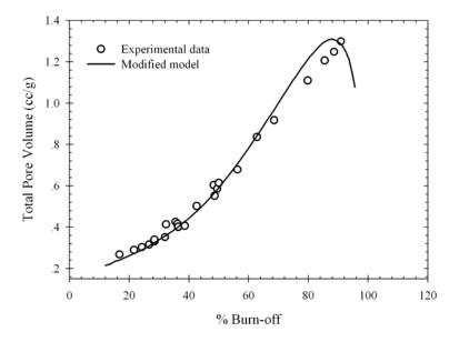
**Figure 4.12** Experimental data and simulated results of total pore volume of palm shell based activated carbons.
