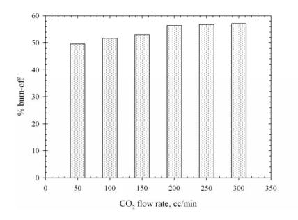
Figure 3.45 Effect of  $CO_2$  flow rate on char burn-off of the palm fiber based activated carbon activated at  $850^{\circ}$ C with pure  $CO_2$  for 2.0 hrs.
