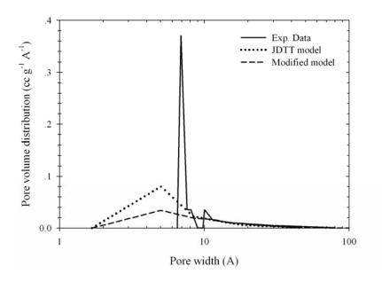
**Figure 4.8** Experimental and computed pore size distributions of longan seed based activated carbons at 47.2 % burn-off.
