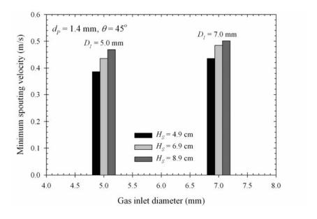
**Figure 5.35** Effect of gas inlet diameters on minimum spouting velocity for particle size of 1.4 mm and conical base angle 45°.
