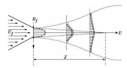
Figure 5.36 Configuration of a turbulent free-jet.
