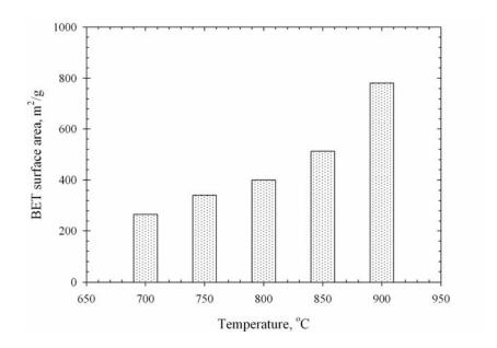
Figure 3.56 Effect of activation temperature on BET surface area of the palm kernel cake based activated carbon activated with pure  $CO_2$  for 2.0 hrs.
