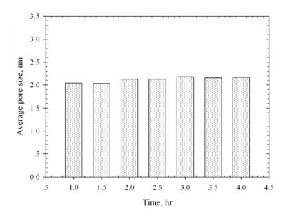
**Figure 3.22** Effect of activation time on average pore size of the palm shell based activated carbon activated at 900°C.
