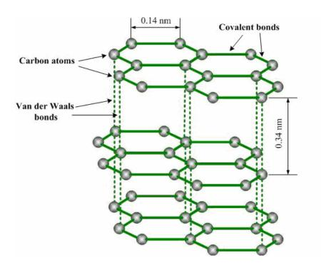
Figure 4.1 Schematic diagram of graphite structure.
