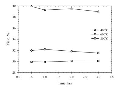
**Figure 3.7** Effect of holding time on the final yield and iodine number of the palm shell chars for particle size of 1.4 mm carbonized at heating rate of 5°C/min.
