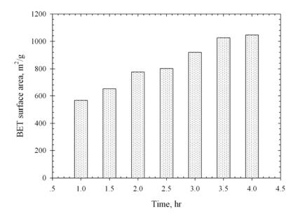
**Figure 3.19** Effect of activation time on BET surface area of the palm shell based activated carbon activated at 900°C.
