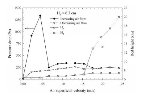
**Figure 5.20** Pressure drop–flow rate diagram and bed height of spouted bed for  $D_I = 5.0 \text{ mm}, d_P = 0.5 \text{ mm}, \theta = 60^{\circ} \text{ and } H_S = 6.3 \text{ cm}.$
