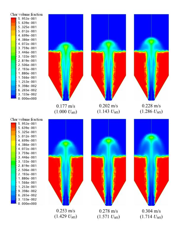
**Figure 5.49** Char particle concentration distribution at several air velocities (Cont.).
