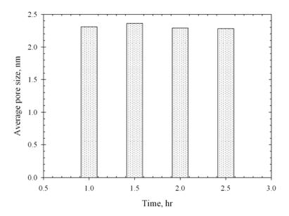
**Figure 3.43** Effect of activation time on average pore size of the palm fiber based activated carbon activated at 850°C with pure CO<sub>2</sub>.
