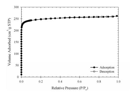
**Figure 5.47** N<sub>2</sub> adsorption isotherm at -196°C of activated carbon prepared at 900°C for activation time of 3.0 hrs in the batch spouted bed.
