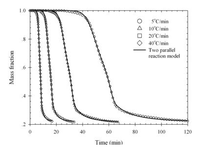
**Figure 2.16** TG data and two-parallel reaction model fitting for palm fiber pyrolyzed at different heating rates.
