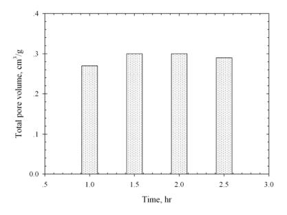
Figure 3.42 Effect of activation time on total pore volume of the palm fiber based activated carbon activated at  $850^{\circ}$ C with pure  $CO_2$ .
