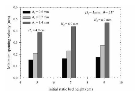
Figure 5.33 Effect of initial bed heights on minimum spouting velocity.
