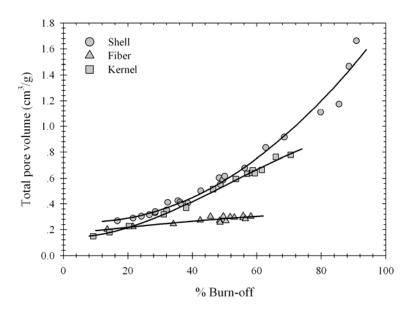
Figure 3.76 Effect of char burn-off on total pore volume.
