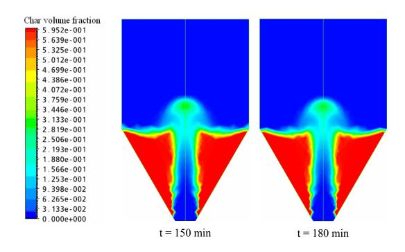
**Figure 5.70** Concentration profiles of palm-shell char at different activation times in the spouted bed activator (Cont.)
