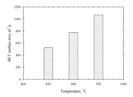
Figure 3.16 Effect of activation temperature on BET surface area of the palm shell based activated carbon activated with pure  $CO_2$  for 2.0 hrs.
