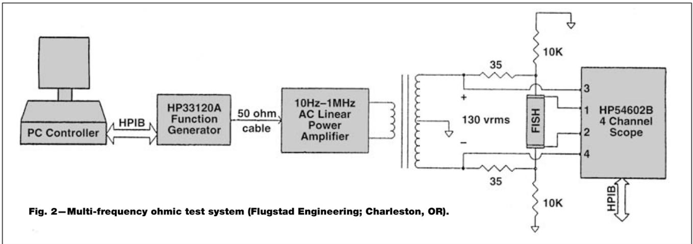
Fig. 2—Multi-frequency ohmic test system (Flugstad Engineering; Charleston, OR).
