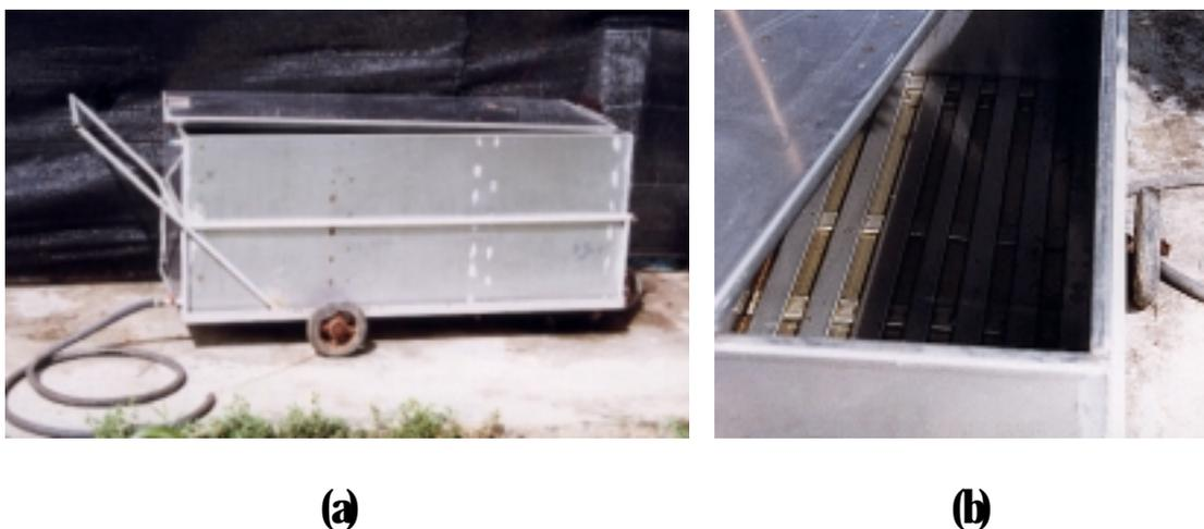
**Fig 5** Photos of 540L fermentor that made from stainless steel (3 wheels drive), comfortable for movement, there are tube and its connection line for steaming a Front view, b Inside Fermentor has sieve to contain substrate during sterile and fermentation
