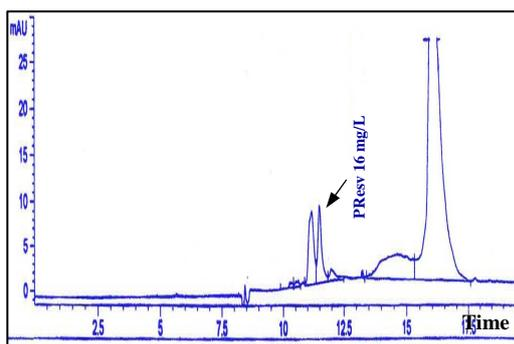
**Figure 15** Electropherogram of standard trans-resveratrol (16 mg/L) spiked plasma was performed with a diode-array detector using an Agilent Technologies model G1600AX. The capillary was an uncoated fused silica of 50  $\mu\text{m}$  i.d. (Agilent). Electrophoretic analyses were performed in 40 mM sodium tetraborate, 20% acetonitrile, pH 9.32, at 25 kV, 25°C. Samples were injected by hydrodynamic 0.5 p.s.i. for 5s. Detection wavelength was 220 nm.
