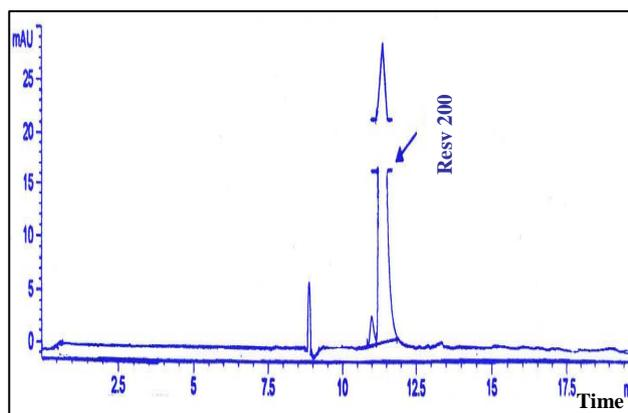
**Figure 14** Electropherogram of standard trans-resveratrol 200 mg/L was performed with a diode-array detector using an Agilent Technologies model G1600AX. The capillary was uncoated fused silica of 50  $\mu\text{m}$  i.d. with effective and total lengths of 50 and 75 cm. Electrophoretic analyses were performed in 40 mM sodium tetraborate, 20% acetonitrile, pH 9.32, at 25 kV, 25°C. Samples were injected by hydrodynamic (0.5 p.s.i.; 1 p.s.i.=6894.76 Pa) for 5s. Detection wavelength was 220 nm.
