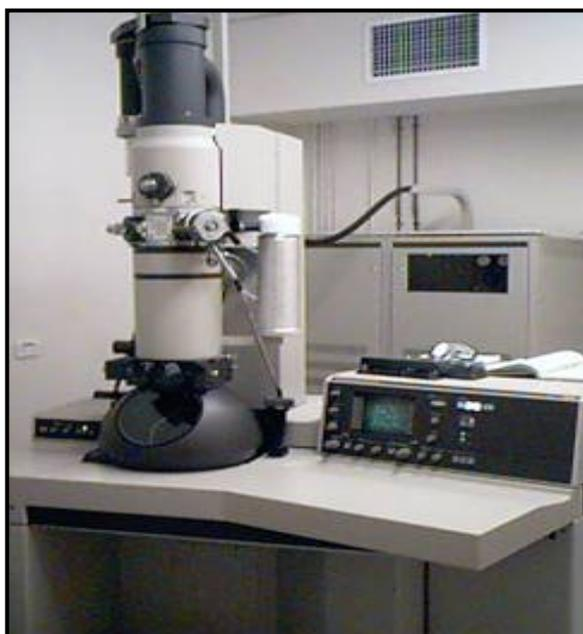
**Figure 8** Transmission electronmicroscope (TEM) (Philips CM10).
