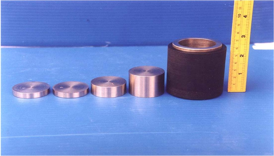
**Figure 3.4** Billets are put in the chamber. When testing the specimen, specimen is put into the chamber then billet number 1 is filled up in the chamber. Billet number 1 is the representation of the pore volume of carbonate rock.
