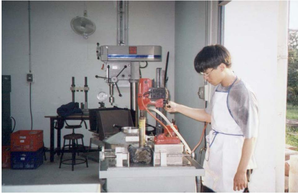
**Figure 3.1** Coring Machine is the instrument that used for drilling the rock samples with cylinder shape.
