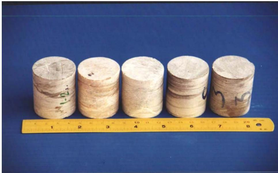
**Figure 3.2** The specimen shape is cylinder. The specimen size is two inches long and one and a half inches diameter.
