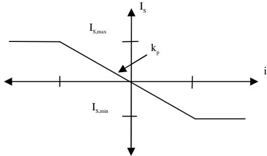
**Fig. 4.** P-controller characteristic
