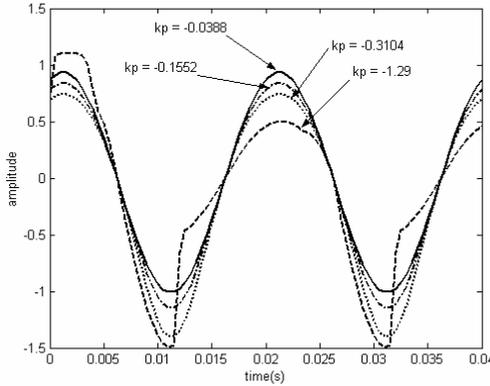
**Fig. 5.** Compensated waveforms with  $k_p$  adjustment
