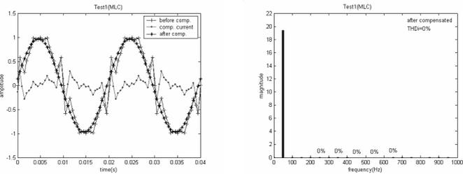
(d) waveforms and spectrum resulting from the MLC method
