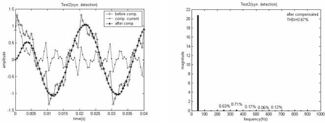
(b) waveforms and spectrum resulting from the SD method
