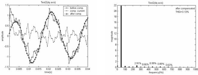
(a) waveforms and spectrum resulting from the DQ method
