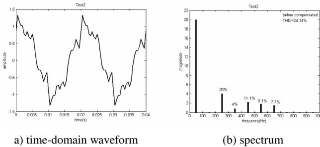
**Fig. 8.** Current waveform for Test 2
