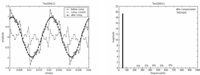
(d) waveforms and spectrum resulting from the MLC method
