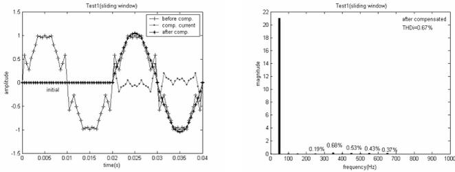
(c) waveforms and spectrum resulting from the SWF method
