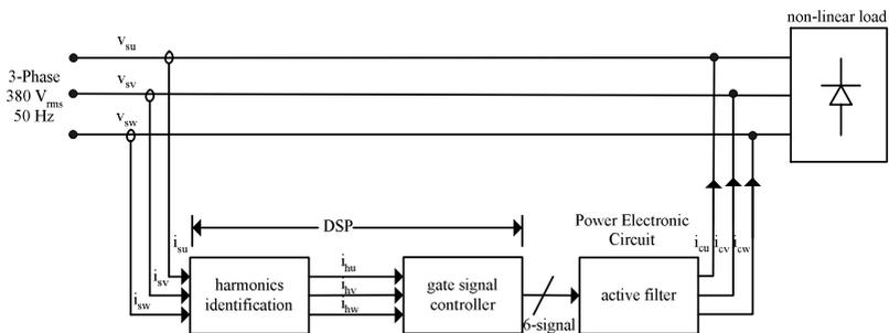
Fig. 1. Structure of active power filters
