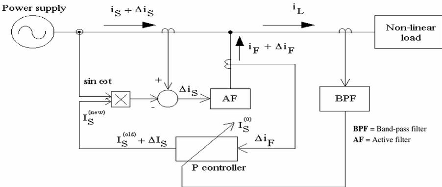
Fig. 2. Power active filter using MLC method
