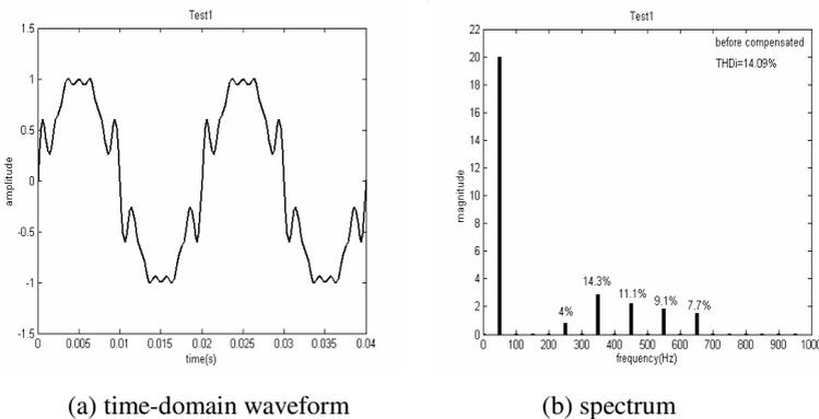
**Fig. 6.** Current waveform for Test 1
