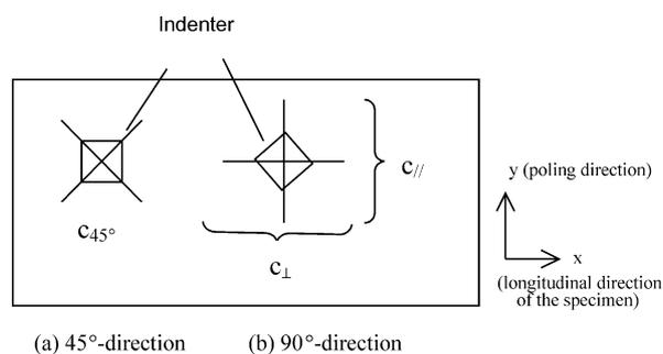
Fig. 2. Relative direction between specimen and indenter on the indenting surface.
