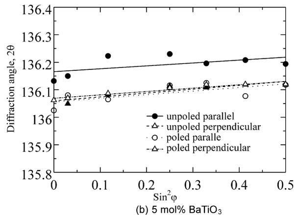
Fig. 7. Relationship between diffraction angle and  $\sin^2\varphi$  for (146) diffraction of  $\alpha$ -Al<sub>2</sub>O<sub>3</sub> matrix for BaTiO<sub>3</sub>/Al<sub>2</sub>O<sub>3</sub> composites sintered at 1450 °C.
