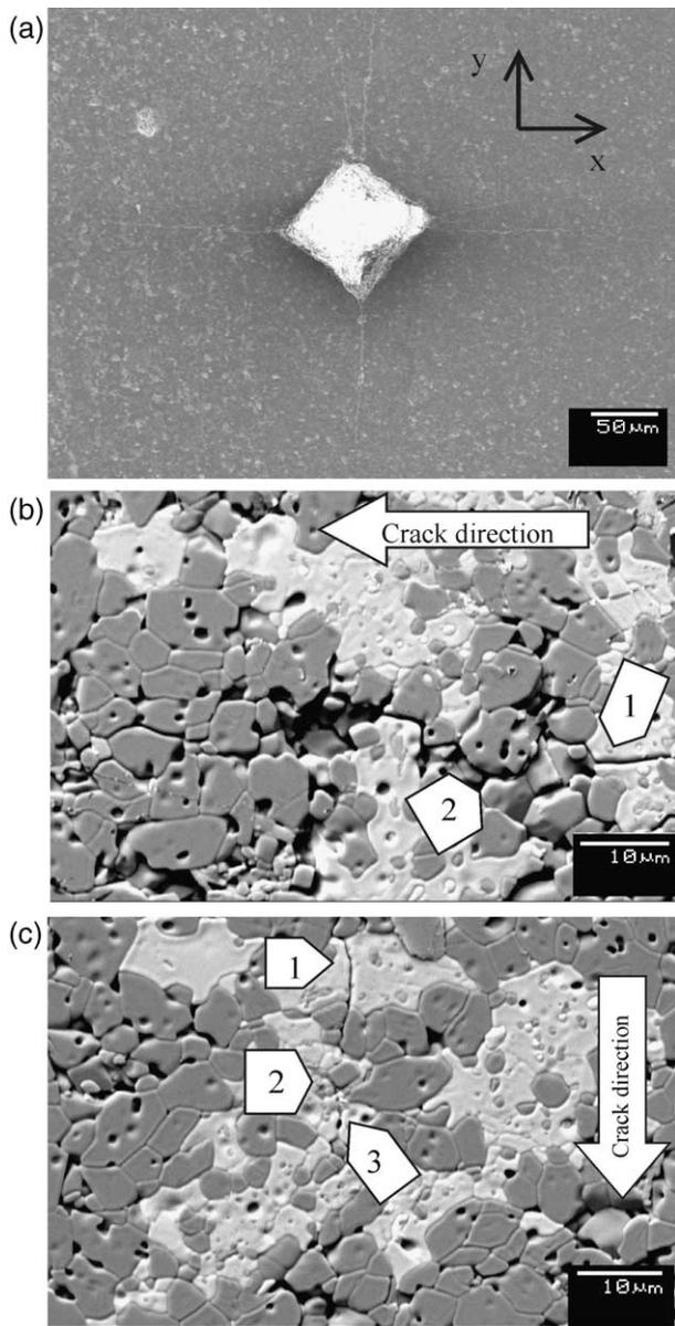
Fig. 4. Cracks propagating from a Vickers indentation in the unpoled 5 mol% BaTiO<sub>3</sub>/Al<sub>2</sub>O<sub>3</sub> composite. Arrows indicate; (1) deflection at or near BaTiO<sub>3</sub> particles, (2) crack bridging, (3) crack arresting at or in the intermediate aggregates. (a) Macro view of the indentation crack, (b) crack path in  $x$  direction, (c) crack path in  $y$  direction.
