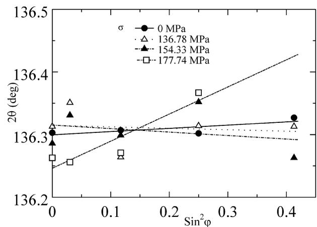
Fig. 8.  $\sin^2\varphi$  diagram for Al<sub>2</sub>O<sub>3</sub> under loading.
