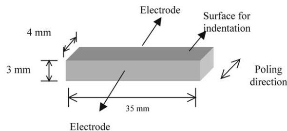
Fig. 1. Specimen dimensions, electrode/indentation surfaces and poling direction.
