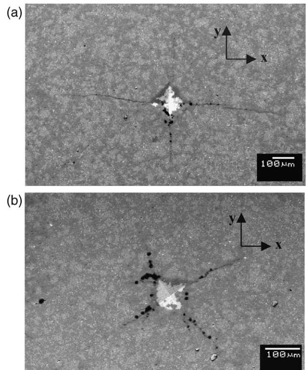
Fig. 5. Macroscopic view of the cracks propagating from Vickers indentation for poled specimens. (a) 90° direction, (b) 45° direction.
