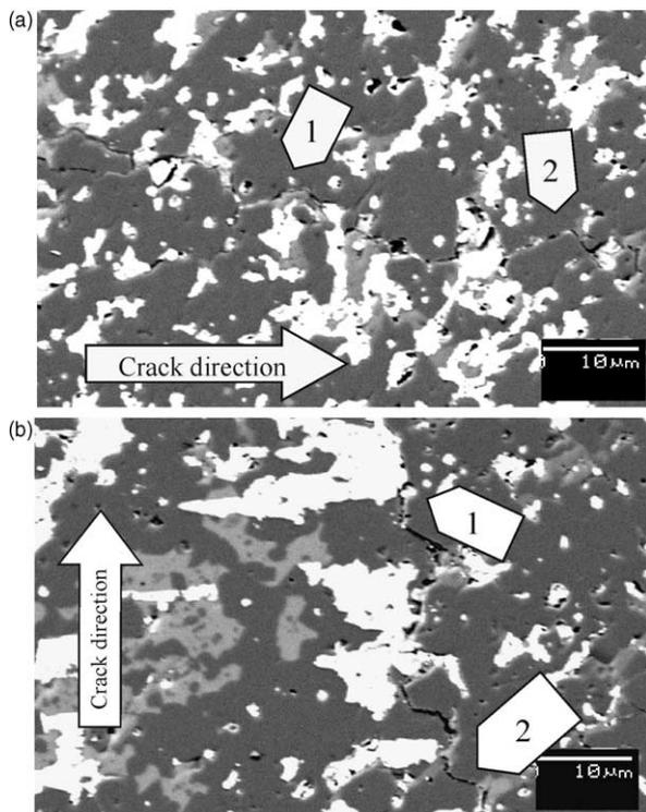
Fig. 6. Crack paths for 5 mol% BaTiO<sub>3</sub>/Al<sub>2</sub>O<sub>3</sub> composite sintered at 1450 °C. Arrows indicate; (1) deflection at or near BaTiO<sub>3</sub> particles, (2) crack bridging. (a)  $x$  direction (perpendicular to the poling direction), (b)  $y$  direction (parallel to the poling direction).
