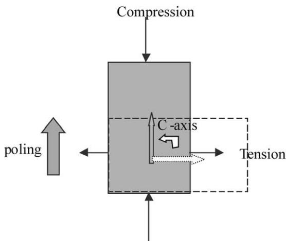
Fig. 9. A schematic of stresses generated from a 90° domain switching under poling electric field.
