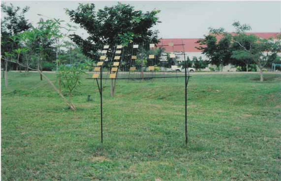
**Figure 3.2** The standard arrangement for natural exposure experiment.
