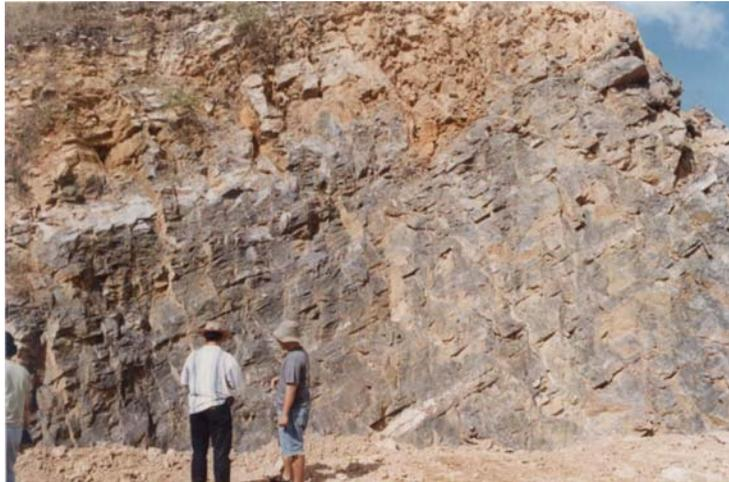
**Figure A.21** Blocky rock slope of limestone quarry is located near with Khao Shee Chan, Chon Buri province (slope no.9).
