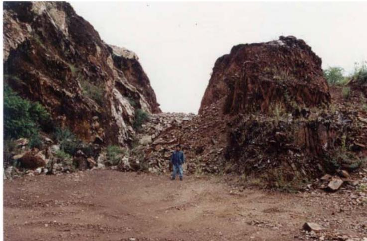
**Figure A.51** Footwall and Hanging wall of Barite mining, Chaing Khan district, Loei province (slope nos.18-23).
