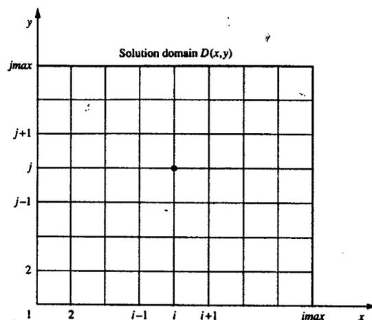
Figure:2.3 Solution domain  $D(x, y)$  and finite difference grid.
