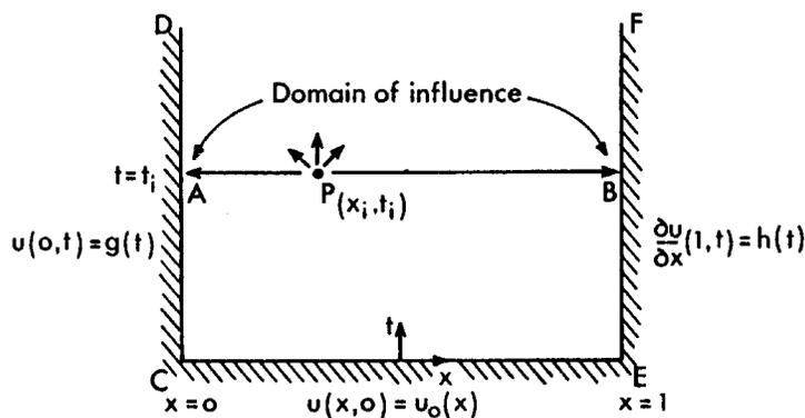
Figure:2.2 Computational domain for a parabolic PDE.
