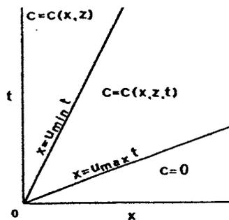
Figure:3.2 Characteristics  $x = u_{\max} t$  and  $x = u_{\min} t$ , separating the region where the concentration is time dependent from the two regions where the pollutant has not yet arrived and steady-state conditions are established.
