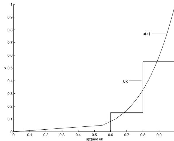
Figure:3.1 Wind profile  $u = z^{0.2}$  and approximating step function  $u_k$  for  $q = 5$  and uniform vertical grid spacing  $\Delta z = 0.05$ .
