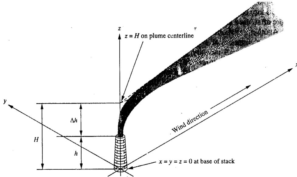
Figure:1.1 Coordinate system and nomenclature for the Gaussian plume idea.
