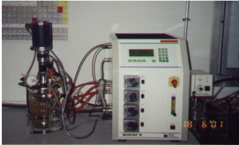
**Figure 3.4** Two litter of reactor for liquid fermentation
