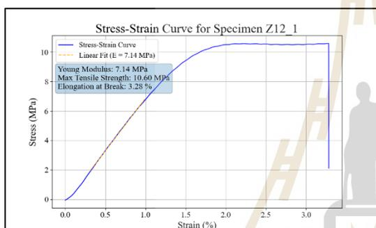
neat resin, z-orientation, 12s exposure time,
