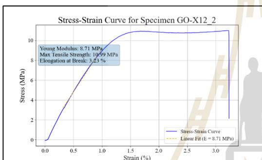
rGO resin, x-orientation, 12s exposure time,
