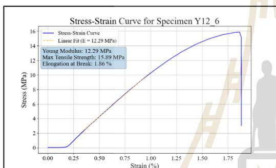
neat resin, y-orientation, 12s exposure time,
