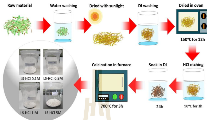
Figure 3.1 The step of SiO 2 nanoparticles synthesis by 1 st HCl etching.
