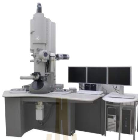
Figure 3.8 Transmission Electron Microscope (TEM), FEI Tecnai G 2 20 200kV TEM/STEM/EDX/Tomography.
