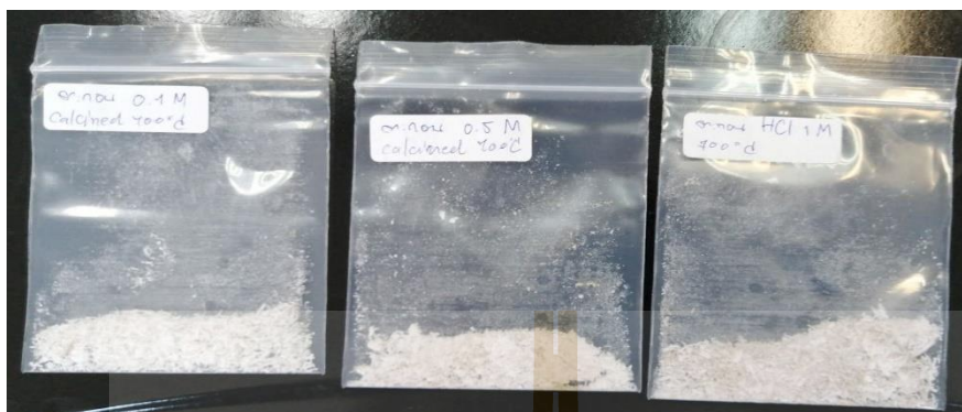
Sediment from samples treated with acid after calcined at 700°C 3h
