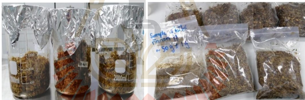
Untreated and acid-treated samples before calcination
