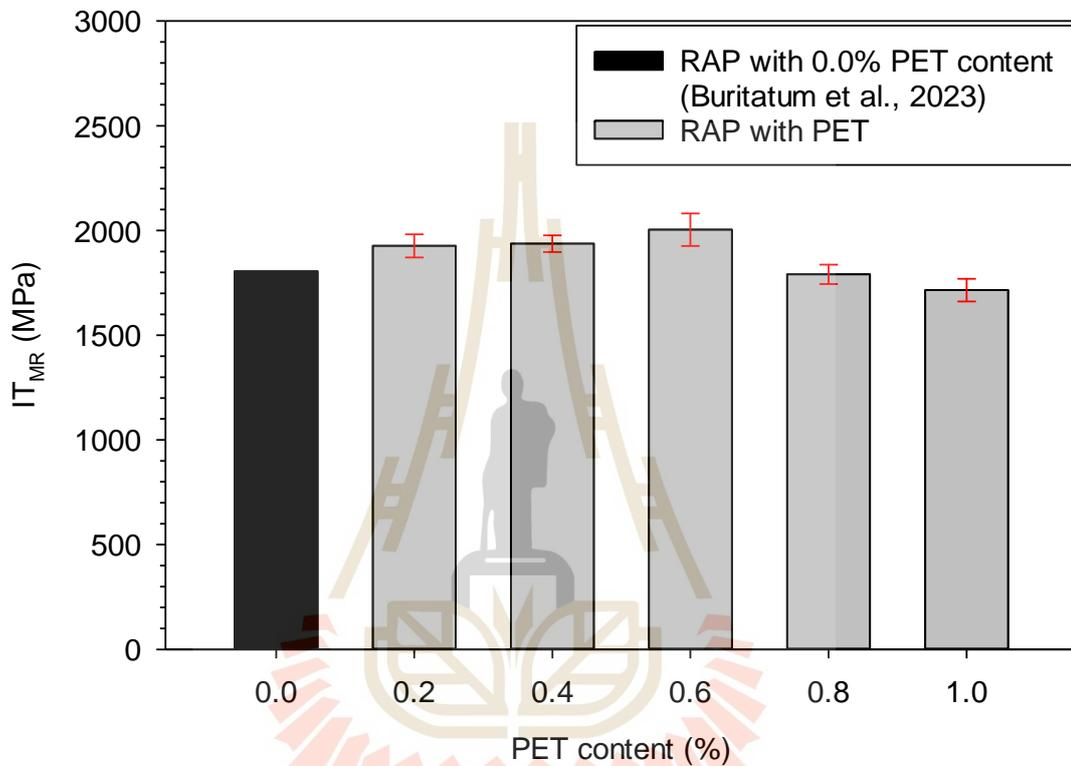
Figure 3.4  $IT_{MR}$  of RAP asphalt concrete samples versus PET content.
