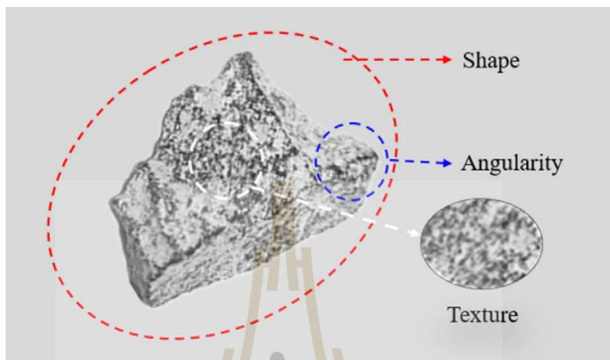
**Figure 2.1** Morphological characterizations of an aggregate (Gong et al., 2021).
