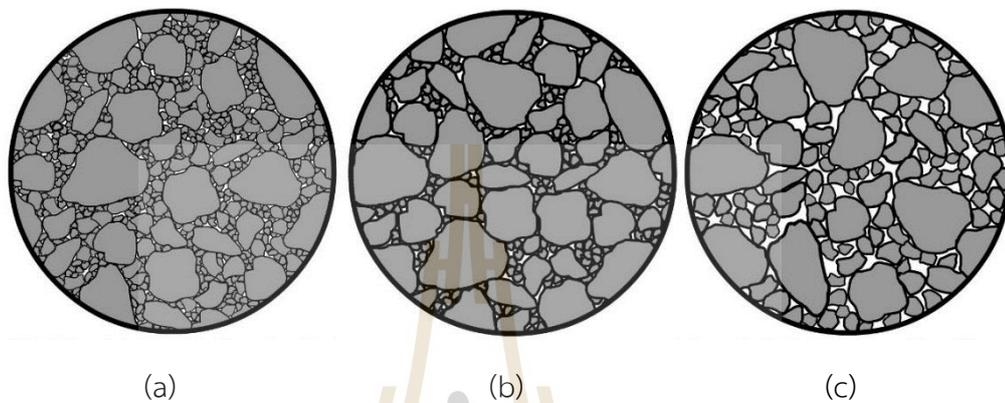
**Figure 2.4** Asphalt concrete mixture schematic (a) Dense-graded mixture, (b) Gap-graded mixture, and (c) Open-graded mixture (Facts, 2007).
