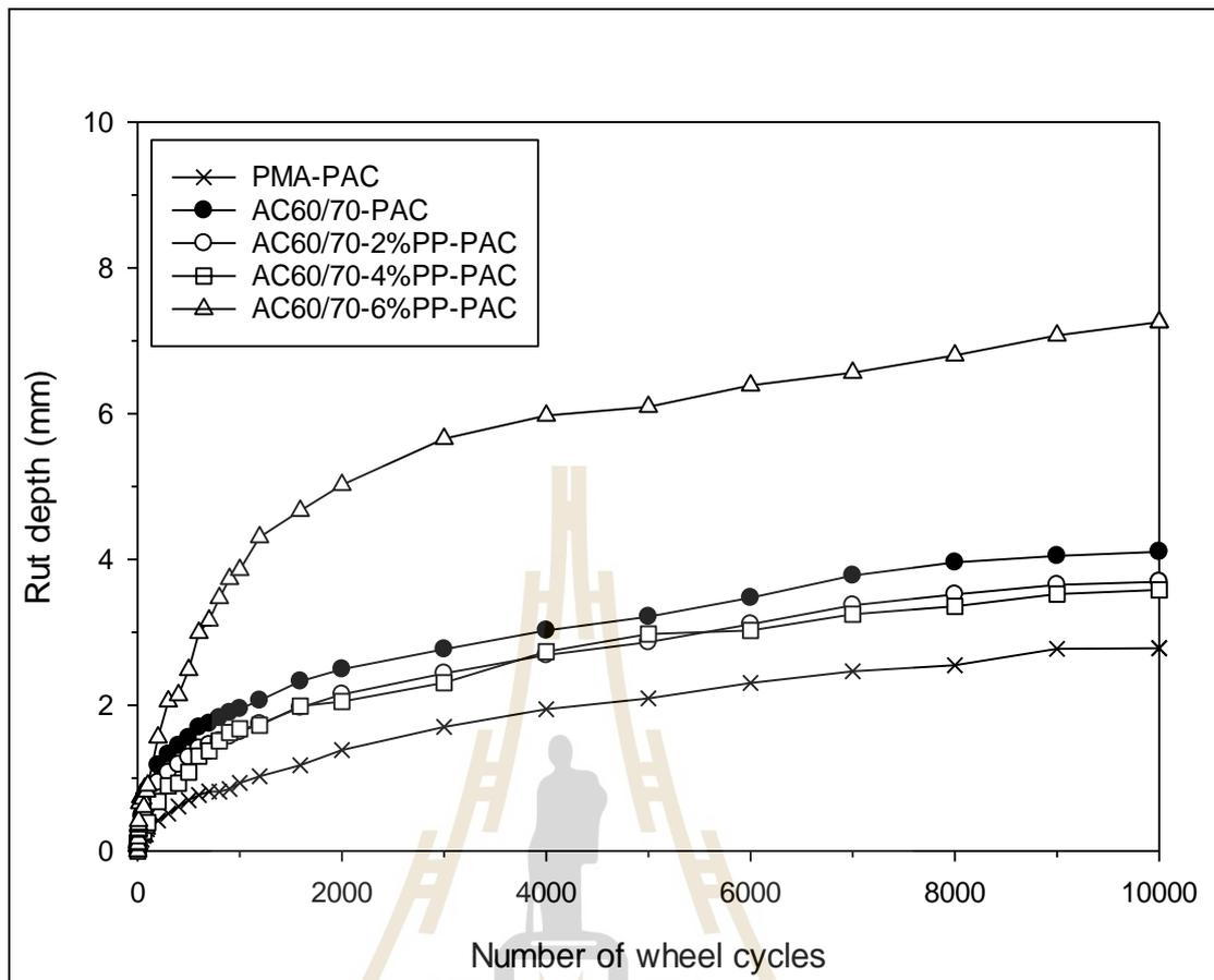
Figure 5.8 The rut depth of PAC samples under testing wheel cycles
