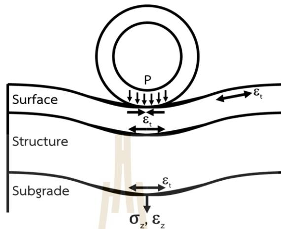
Figure 2.8 Tensile and compressive strain in pavement
