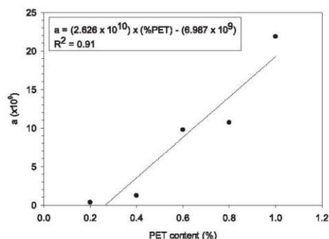
Fig. 8. Fatigue parameter ( $a$ ) of RAP asphalt concrete with PET samples versus PET content.
