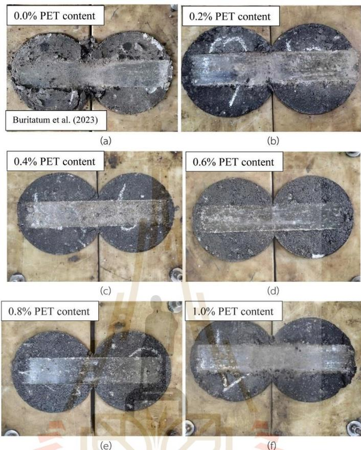
Fig. 11. Failure characteristics of RAP asphalt concrete modified with (a) 0%PET content [16], (b) 0.2%PET content, (c) 0.4%PET content, (d) 0.6%PET content, (e) 0.8%PET content, and (f) 1.0%PET content.
