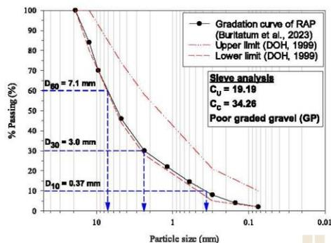
Fig. 2. Gradation curve of aggregate (modified from [16]).
