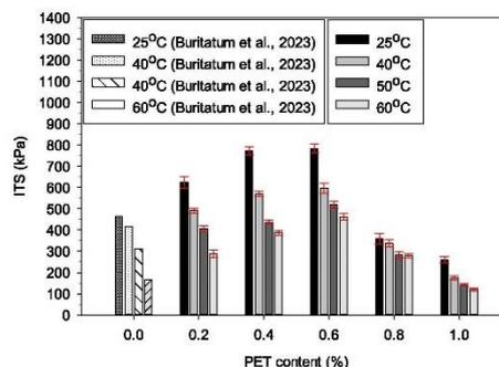
Fig. 3. ITS of RAP asphalt concrete samples at 25°C, 40°C, 50°C, and 60°C and PET content.
