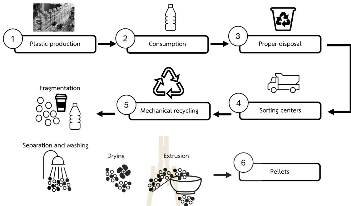
**Figure 2.6** Schematic illustration of mechanical recycling of plastic materials (Duarte & Faxina, 2021).
