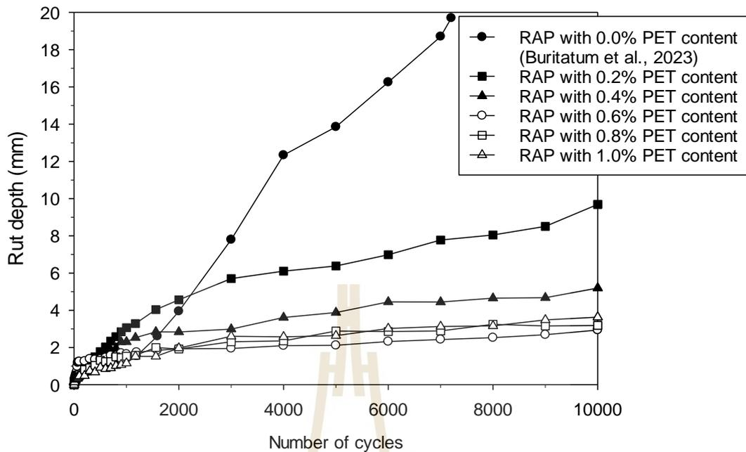
**Figure 3.10** Rut depth of RAP asphalt concrete at various PET content versus number of cycles.
