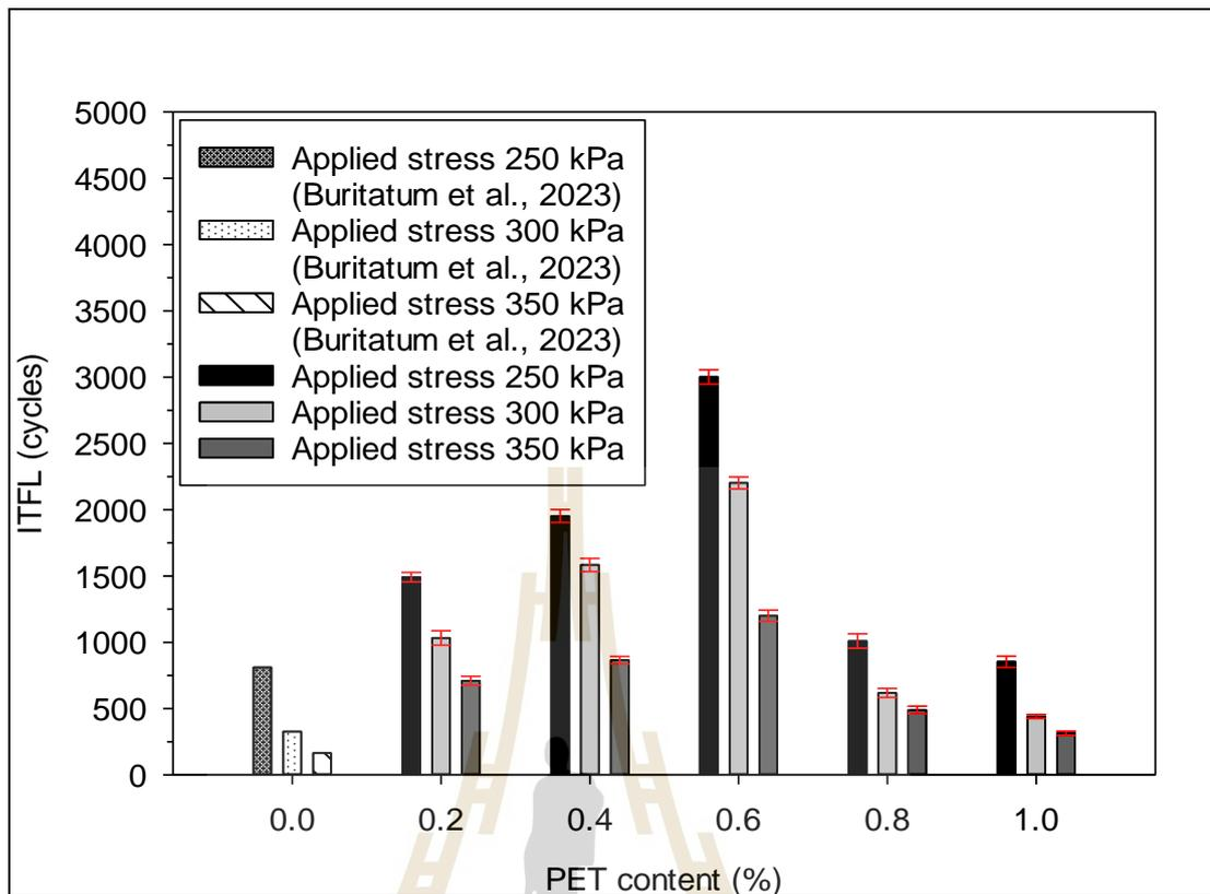
**Figure 3.6** ITFL of RAP asphalt concrete samples versus applied stress at different PET content.
