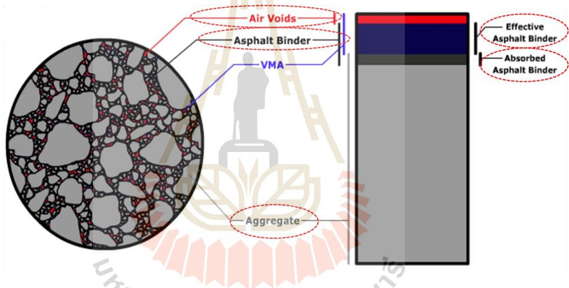
Figure 2.5 The volume fractions of asphalt concrete mixture (Kumar et al., 2021)
