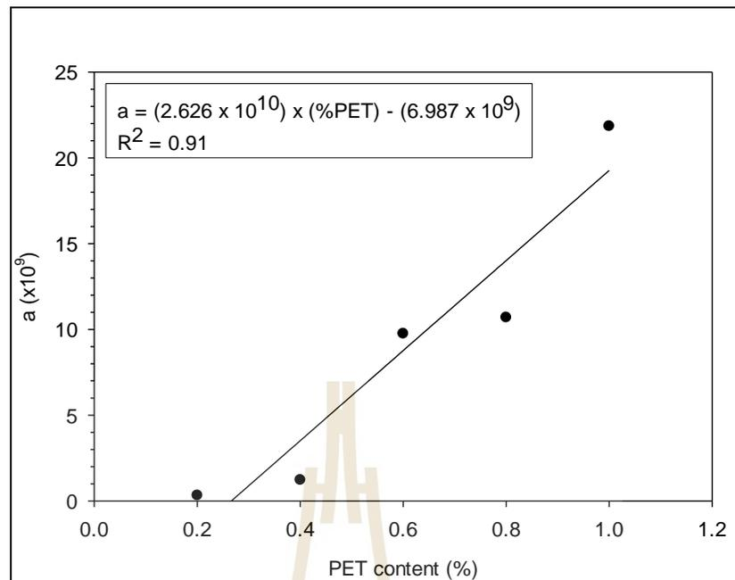
Figure 3.8 Fatigue parameter ( $a$ ) of RAP asphalt concrete with PET samples versus PET content.
