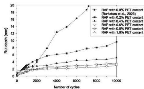
Fig. 10. Rut depth of RAP asphalt concrete at various PET content versus number of cycles.
