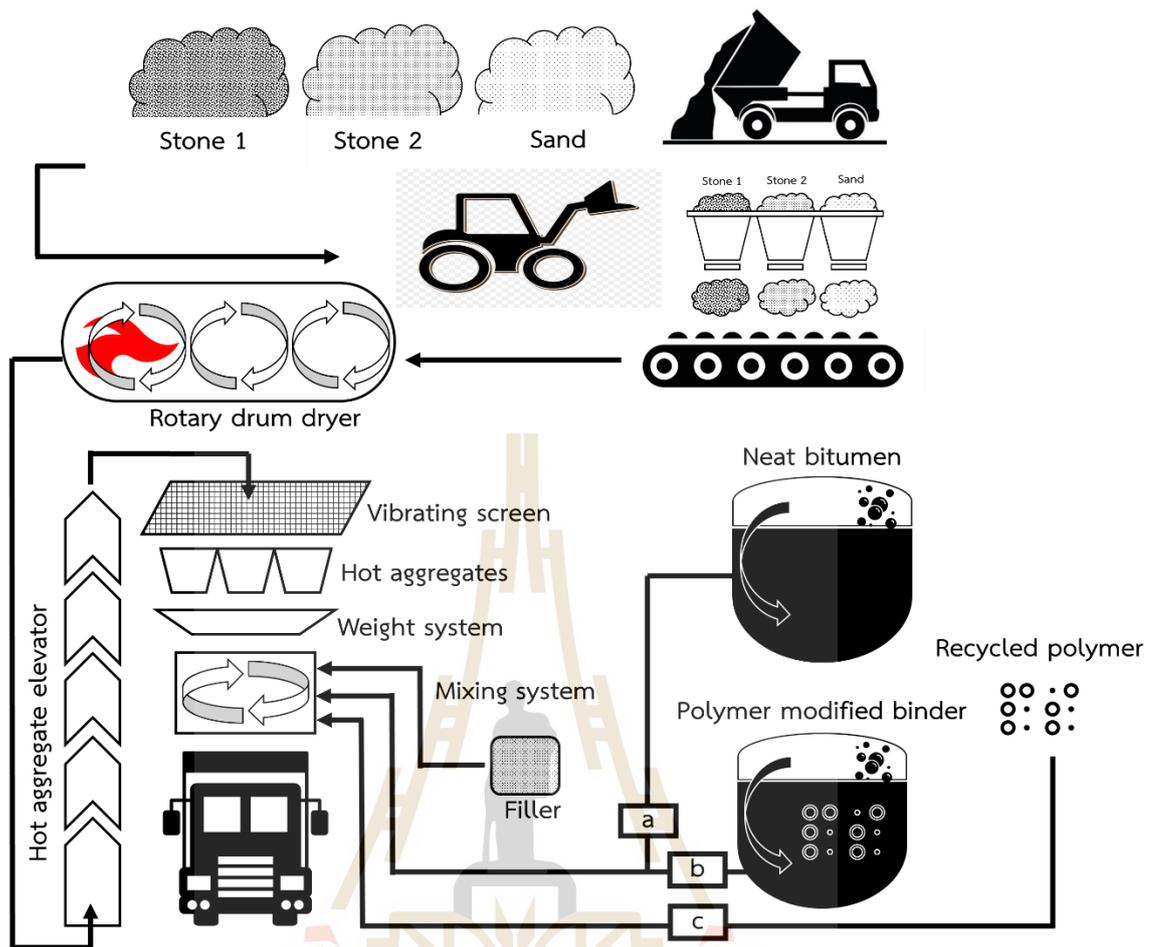
**Figure 2.7** Schematic illustrates of the wet and dry processes in a discontinuous asphalt plant (Brasileiro et al., 2019).
