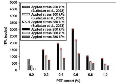
Fig. 6. ITFL of RAP asphalt concrete samples versus applied stress at different PET content.
