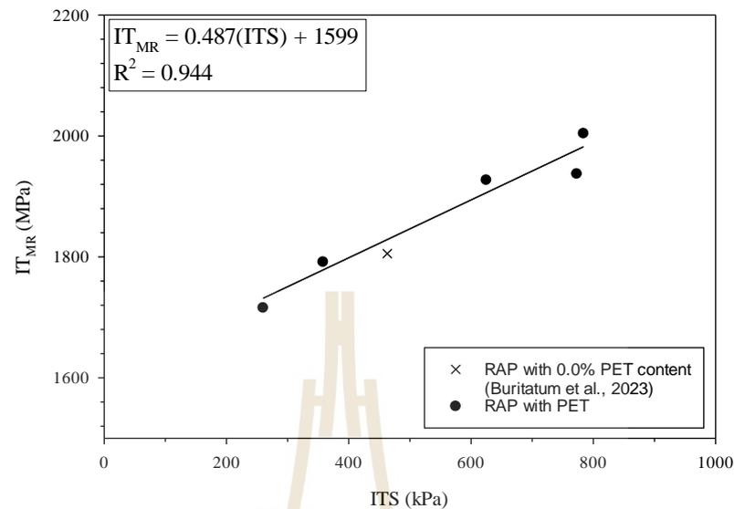
**Figure 3.5** Relationship between  $IT_{MR}$  and ITS of RAP asphalt concrete samples.
