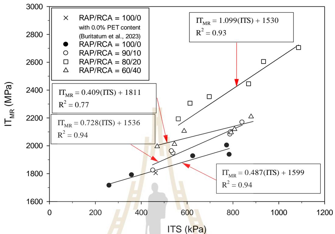
**Figure 4.5** Relationship between  $IT_{MR}$  and ITS of RAP-RCA-PET asphalt concrete.
