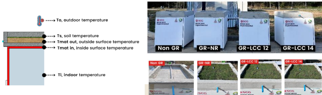
Figure 4.20 Open-air experimental green roofs
