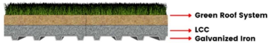
Figure 5.2 Layer system of GR-LCC 12
