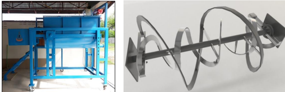
Figure 3.2 Horizontal LCC mixer machine and stirring blades agitator type
