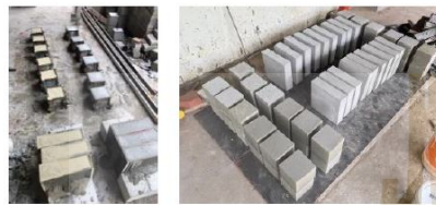
Fig 4. LCC molding process
