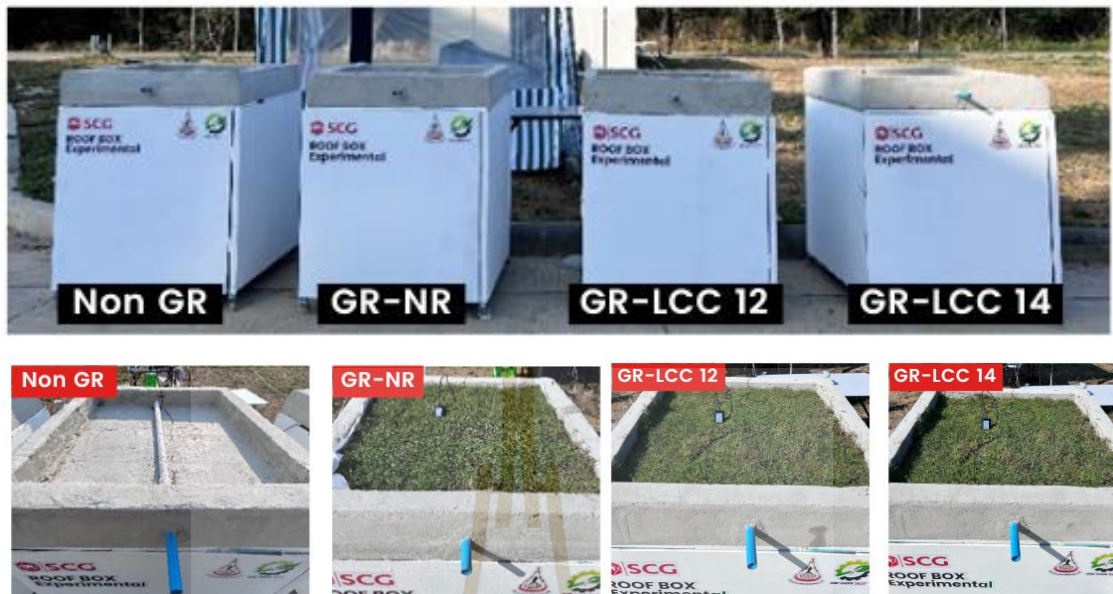
Figure 3.10 The view of the open-air experiment and green roof models
