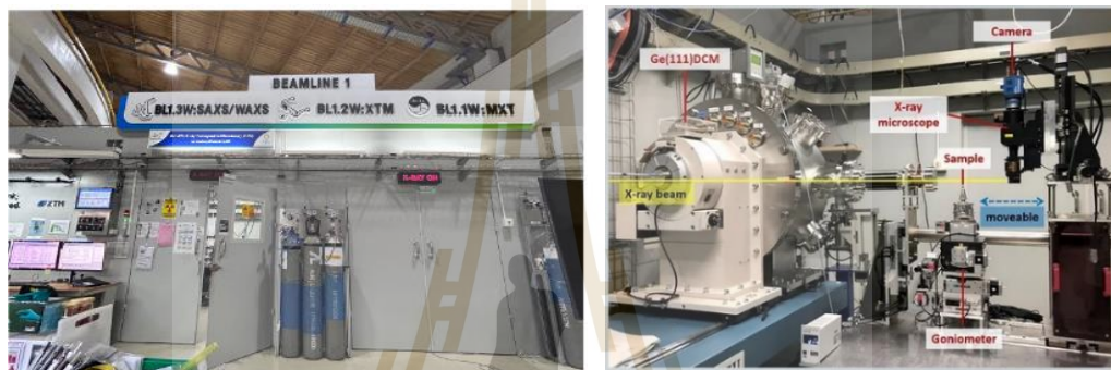
Figure 3.6 Beamline of Synchrotron Radiation X-ray Tomographic Microscopy (SRXTM)
