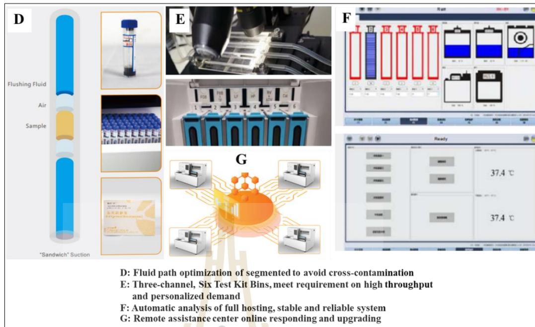
Figure 2.9 A feature on Automatic stool processing machine (D-G)
