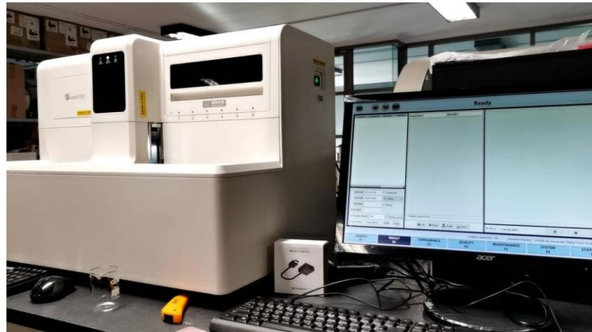
Figure 2.7 Machine composition of FA280 Fully Automatic Feces Analyzer (Orienter, China 2022)
