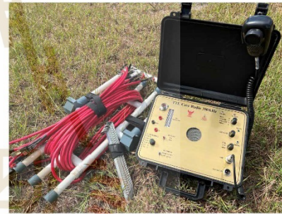
Fig.17 Prototype of TTE 350 kHz cave transceiver
