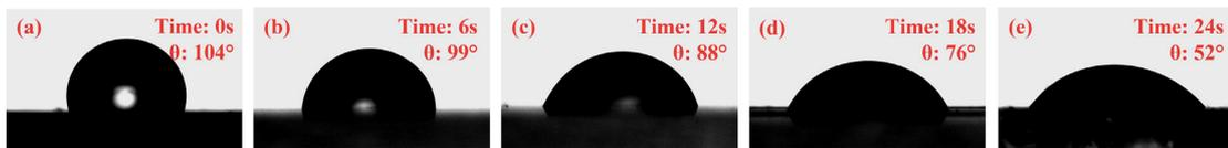
**Figure 2.17** The contact angle of glycerol droplet on the poly(dimethylsiloxane) film (a) without and with the oxygen plasma treatment using different exposure time that were (b) 6, (c) 12, (d) 18, and (e) 24 s (Duangkanya et al., 2022).
